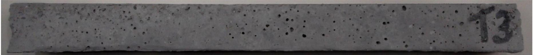
Figure 6.16: Photo of unreinforced specimen on the first day (UNR).
