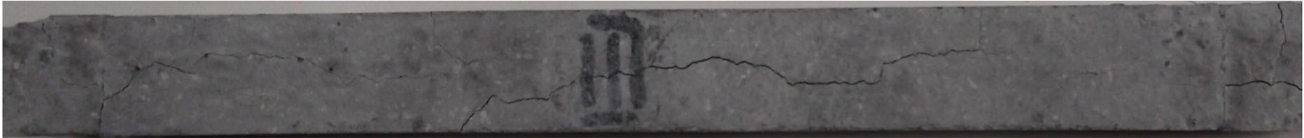
Figure 6.19: Photo of specimen at the end of 30 days which was reinforced with Wire 40 KG.
