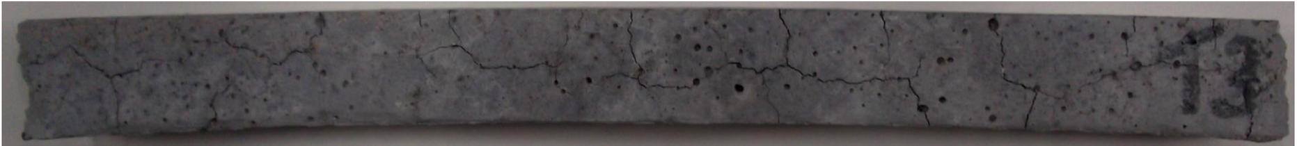
Figure 6.17: Photo of unreinforced specimen at the end of 30 days (UNR).
