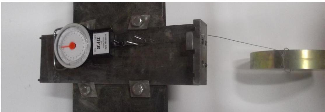
Figure 5.13: System to determine friction loss.
