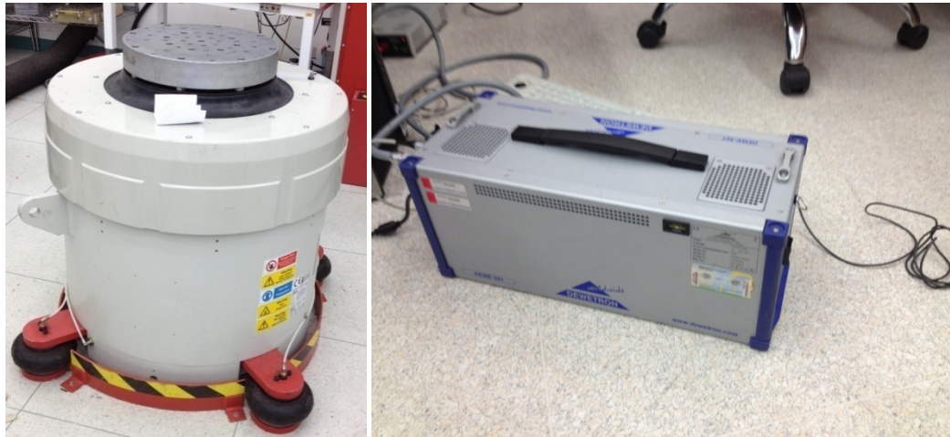
Figure 6.1 LDS V875LS-440 air cooled vibrator (left) and DEWETRON-501 (right)
