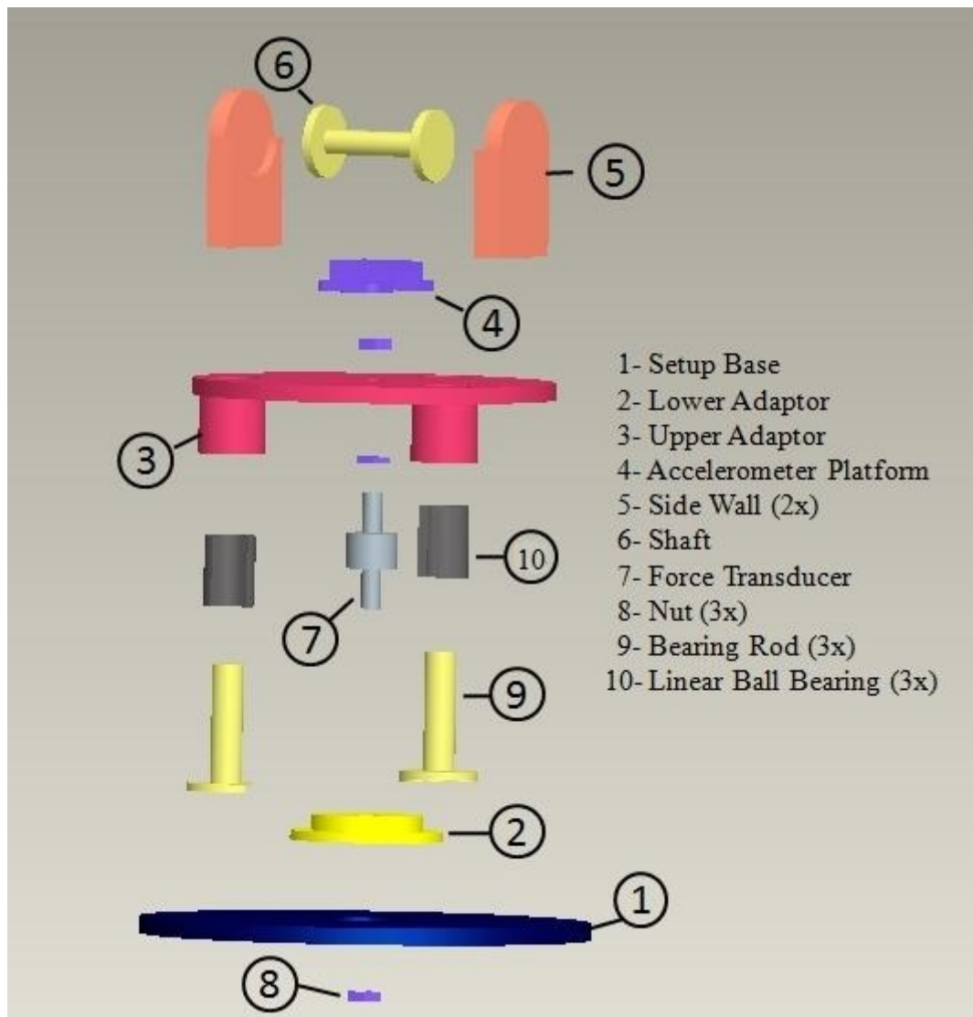
Figure 5.5 Exploded view for the simplified CAD model of the modified test setup
