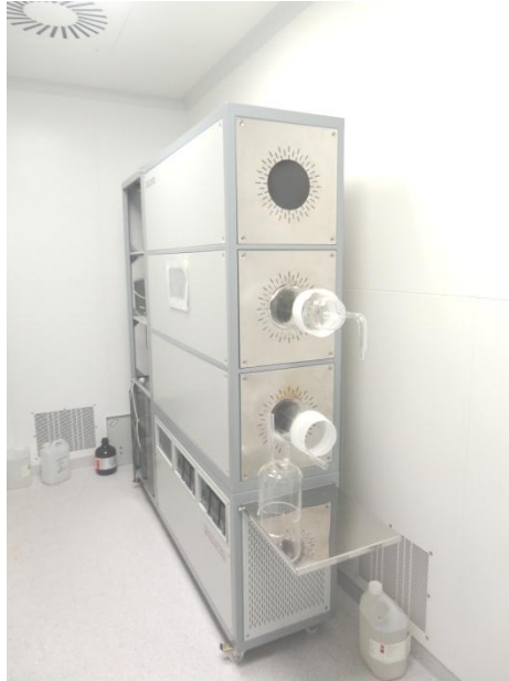
Fig. 3.3 Thermal oxidation furnace in METU-Central Laboratory Cleanrooms
