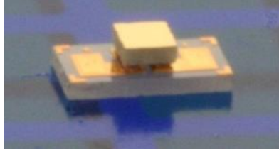
Figure 3.18 Nextreme UPF4 Optocooler TM thermoelectric cooler. (1.5x2.5 mm 2 footprint).
