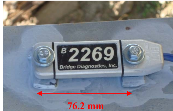
Figure 2.20: Installed BDI ST-350 strain transducer
