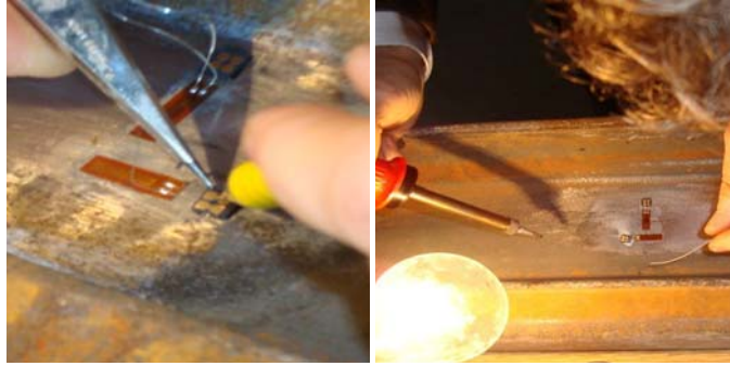
Figure 2.32: Placing (left) and welding terminals (right)
