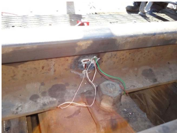
Figure 2.49: two foil strain gages of rail load sensor located on inner web of rail at exit of first span
