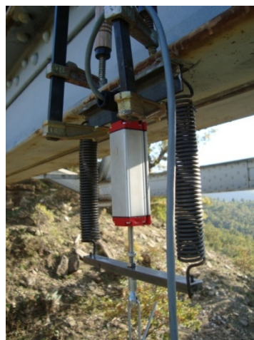
Figure 2.47: Installed LVDT mechanism on middle of first span's bottom chord
