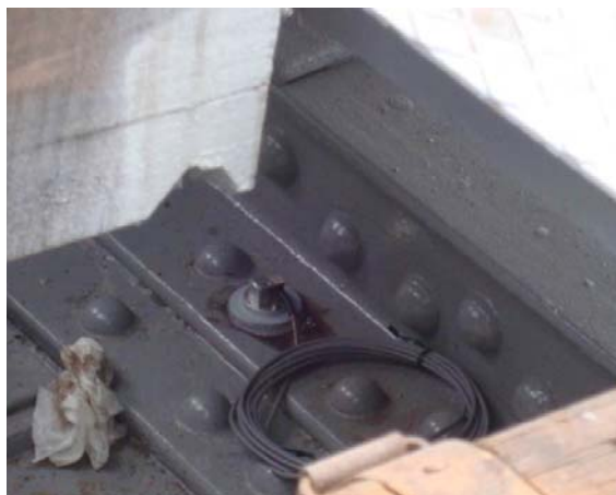
Figure 2.54: Installed accelerometer at the joint U2
