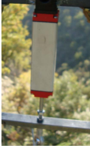
Figure 2.22: Installed Opkon LPM potentiometrical LVDT
