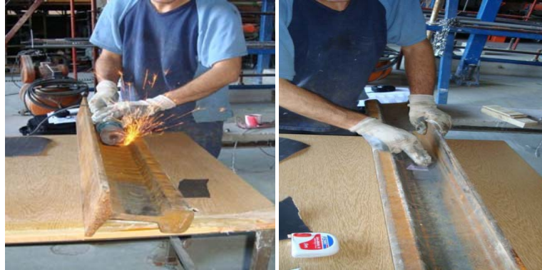
Figure 2.30: Removing impurities by mechanically (left) and chemically (right)
