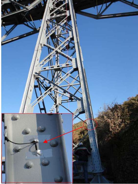
Figure 2.55: Installed strain transducer on 19 m pier.
