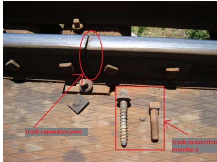
Figure 2.4: S49 Railroad track, expansion joint and railroad track connection members
