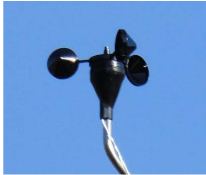
Figure 2.24: Installed NRG #40C Anemometer
