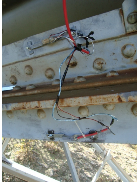
Figure 2.43: Installed two omega gages on critical compression member U1U2
