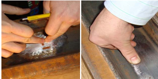
Figure 2.31: Placing (left) and fixing strain gages (right)
