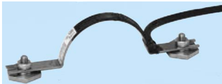
Figure 2.21: Installed Kyowa BCD-E70S strain transducer
