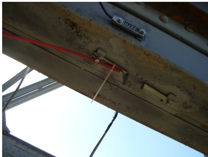
Figure 2.45: Installed one omega gage on bottom flange and one BDI gage on web of critical tension member L1L2
