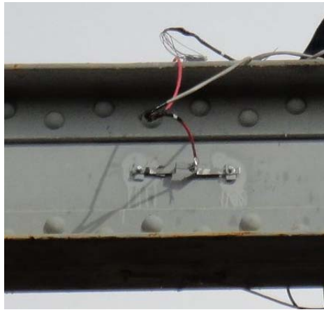
Figure 2.28: Installed and painted omega sensor on web of tension member L2L3
