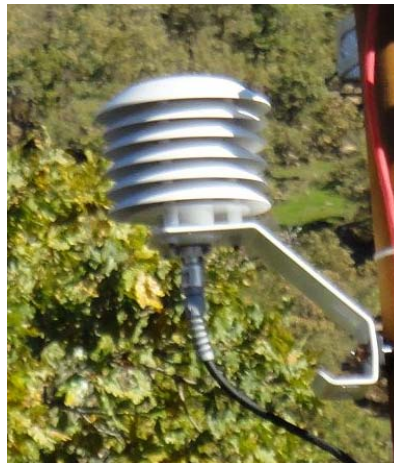
Figure 2.23: Installed Campbell Scientific CS215 Temperature and Relative Humidity Sensor
