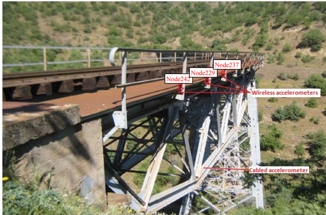
Figure 2.42: Location of wireless and cabled accelerometers used during first field study
