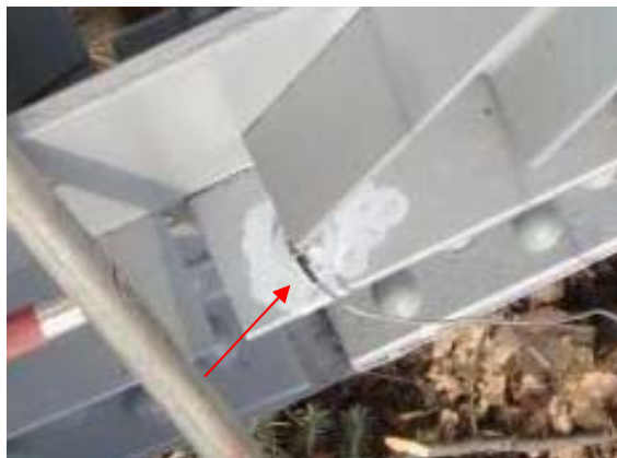
Figure 2.53: Installed accelerometer at the joint L2
