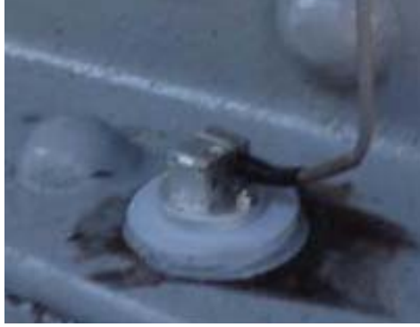
Figure 2.26: Installed Kyowa AS-5GB Accelerometer
