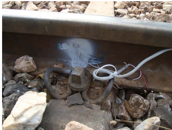
Figure 2.48: two foil strain gages of rail load sensor located on outer web of rail at entrance of first span
