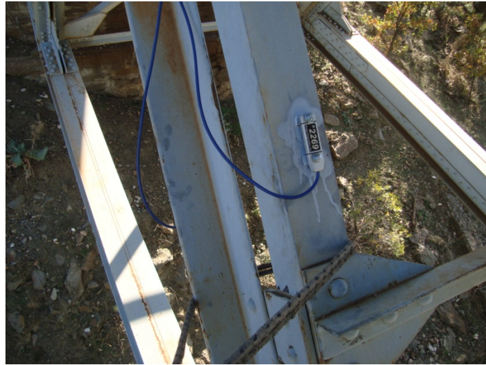
Figure 2.44: Installed two BDI gages on critical tension-compression member U1L2
