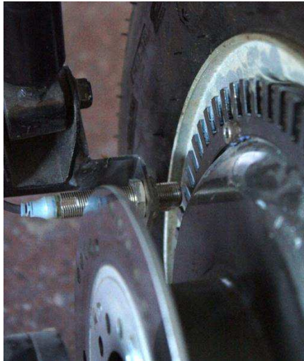
Figure 3-17: Proximity sensor and the encoder disc at the rear wheel
