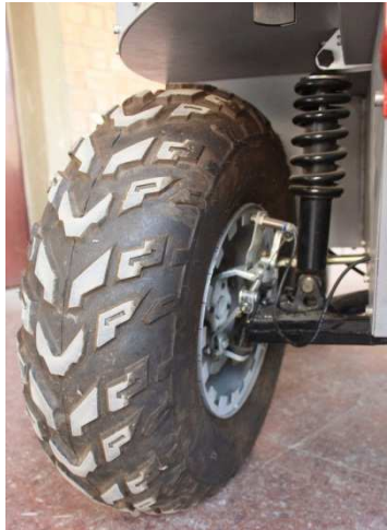
Figure 3-6: Steering and suspension mechanism at front wheels
