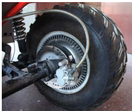
Figure 3-16: Hub motor, wheel, brake system, suspension and rear axle assembly
