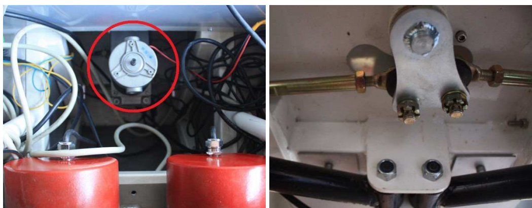
Figure 3-4: Steering motor from top (left) and rods from bottom (right)
