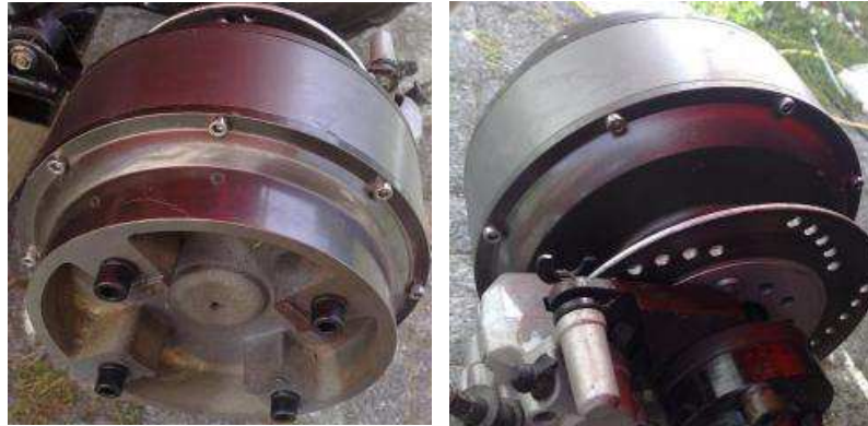
Figure 3-15: In-wheel motor that is mounted in the rear wheels
