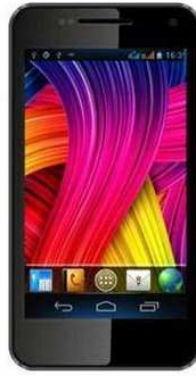
Figure 1.17: An Indian-bound dual-SIM Android smartphone with a 4.3" (800x480) Super AMOLED display [38]
