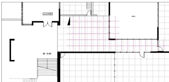
diagram of homogeneity | homogeneous space plan | repeating squares | waffle slab highlighted
