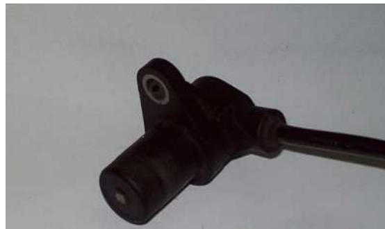
Figure 3.20: Magnetic pick-up which is used in our system
