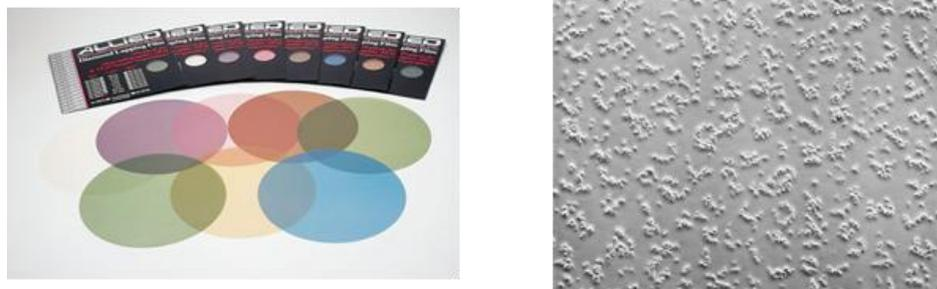
**Figure 3.2** Diamond lapping films and microscope image of diamond particles
