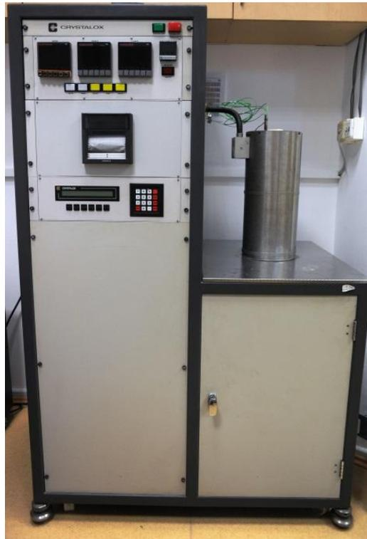
**Figure 2.9** Three-zone vertical Bridgman furnace located at METU Physics Department
