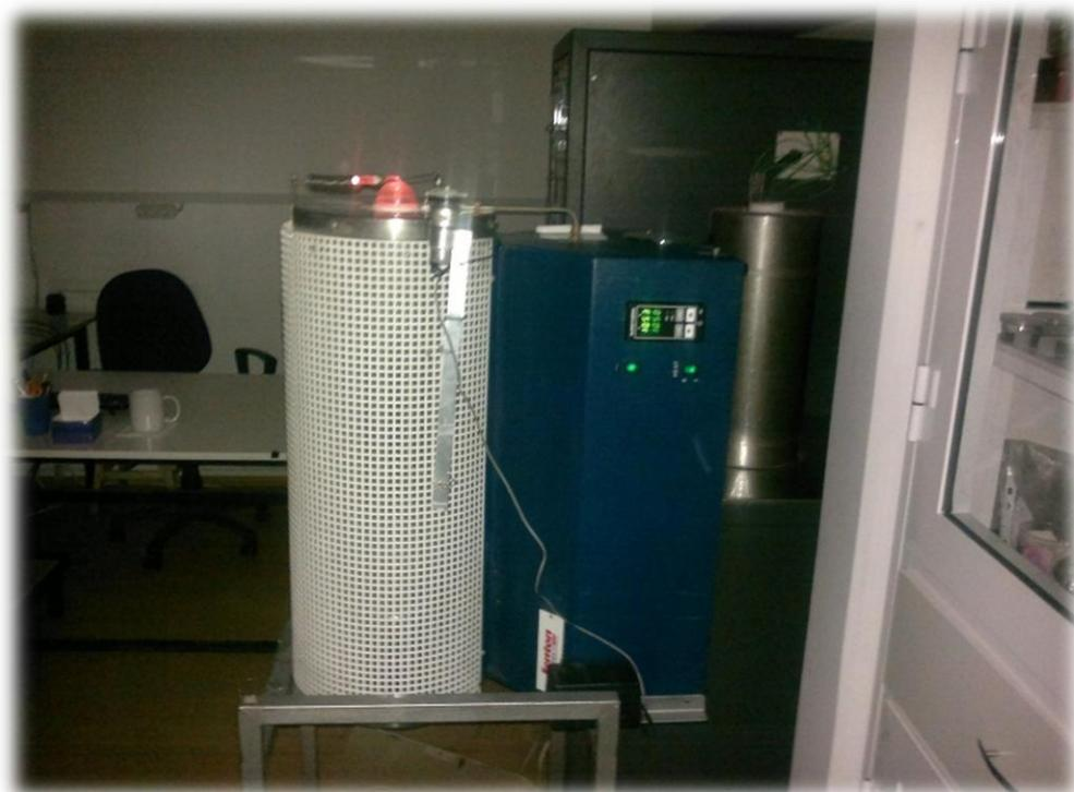
**Figure 2.8** Vertical homogenization furnace with rocking apparatus located at METU Physics Department
