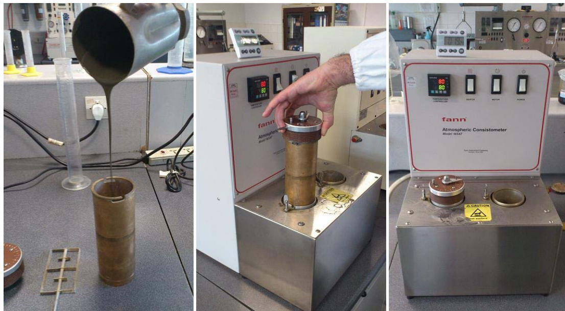
Figure 3-2 Cement slurry conditioning in the atmospheric consistometer
