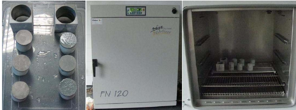
Figure 3-5 Dehydration of core specimens at temperature-controlled oven
