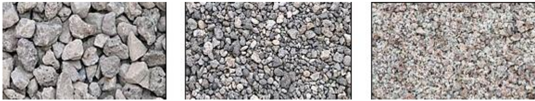
Figure 2-3 Left to right, air-cooled BFS, expanded BFS and GGBFS (NSA 2012)
