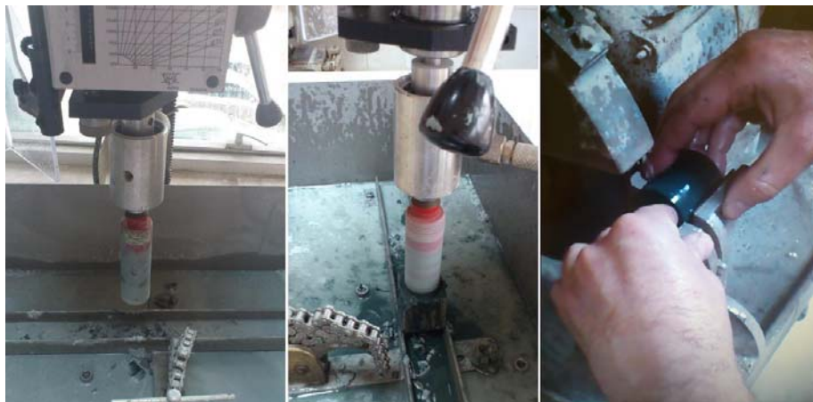
Figure 3-4 Coring and smoothing the edges of specimens
