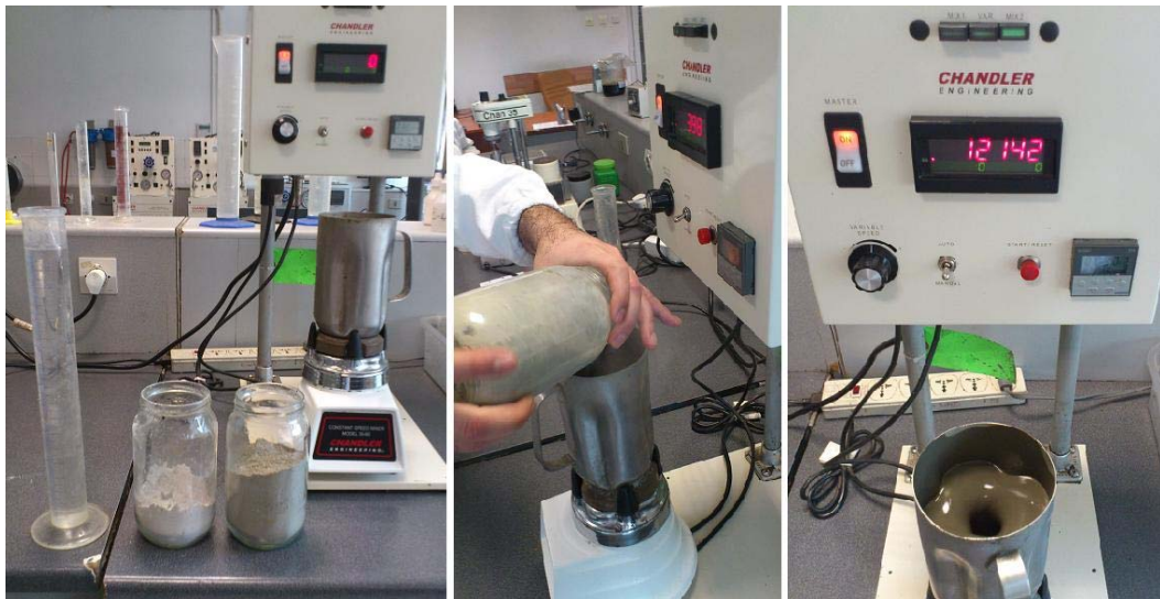
Figure 3-1 Cement slurry preparation with multi-speed mixer
