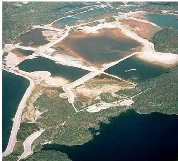
Figure 2.6 Ring-dike type impoundment (Steiner, 2006)
