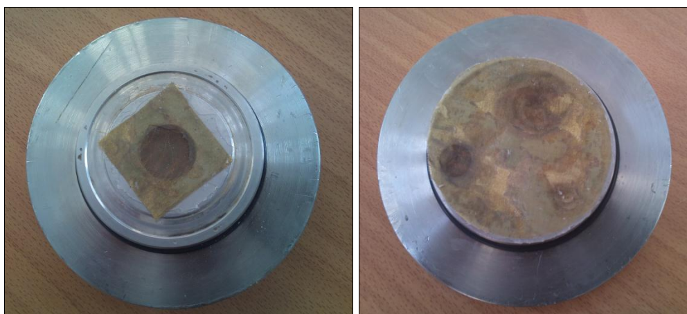
Figure 7. 4 Back and front covers are sealed with metal screens
