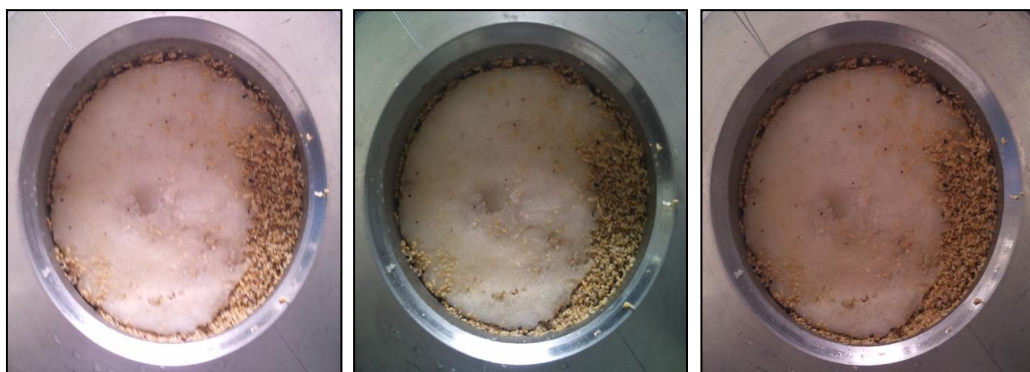
Figure 8. 5 Hydrate formation at the top of the cell from run #3 (Hydrate formation test within the sediments particle size of which are lower than 0.840 mm)
