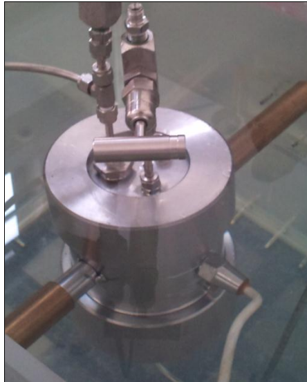
Figure 7. 2 The high pressure cell of hydrate formation and dissociation
