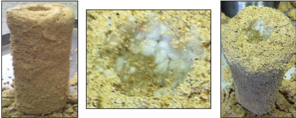
Figure 8. 13 Pictures indicating the hydrate formation within unconsolidated sand pack system (Hydrate permeability test at 50% hydrate saturation and CO 2 injection into CH 4 hydrate in unconsolidated sediments particle size of which range between 0.5 mm and 0.25 mm)
