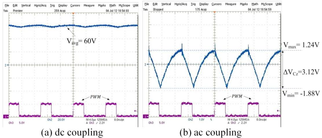
**Figure 5-5**  $C_z$  voltage waveform against applied PWM in CCM, a) dc coupling, b) ac coupling
