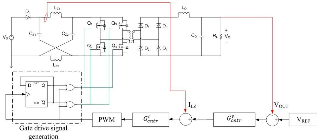
**Figure 4-10** Closed-loop simulation model of Z-source dc/dc converter
