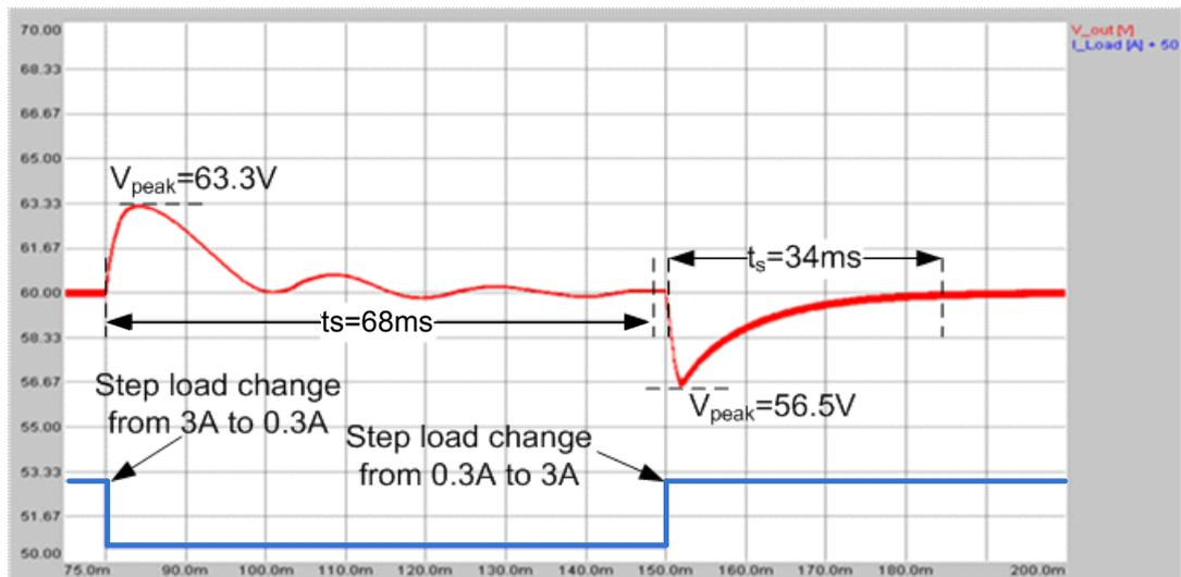
**Figure 4-12** Output voltage during full-load-to-10% load-to-full-load transition under 18V input voltage
