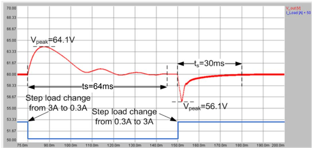
**Figure 4-11** Output voltage during full-load-to-10% load-to-full-load transition under 32V input voltage
