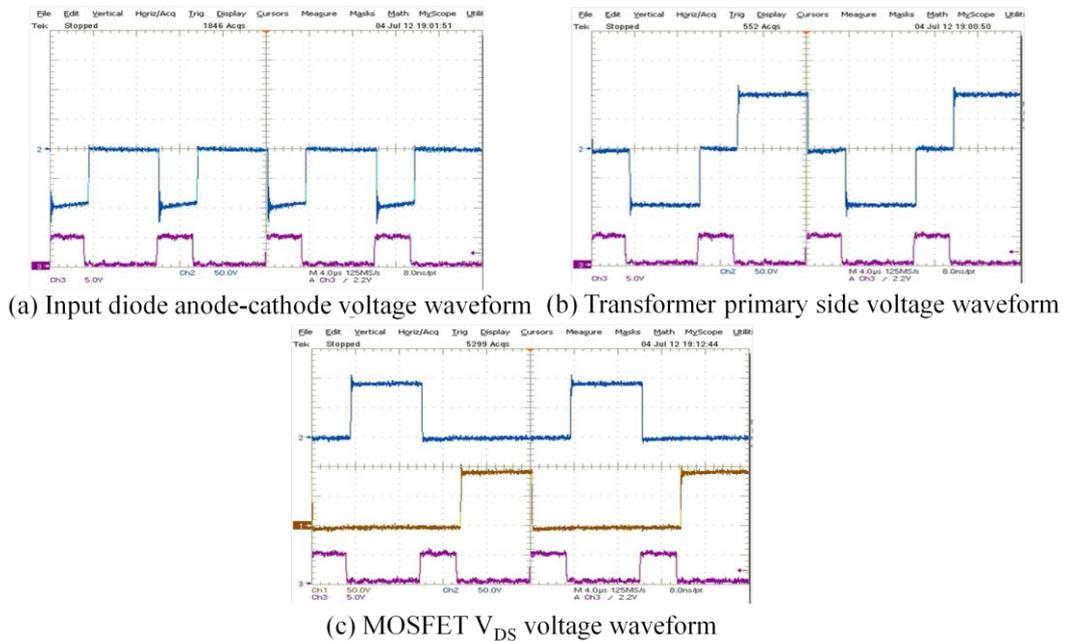
**Figure 5-7** a)  $D_i$  anode-cathode, b) isolation transformer primary side, c)  $Q_1 - Q_3$  cross-pair  $v_{DS}$  voltage waveforms against applied PWM in CCM
