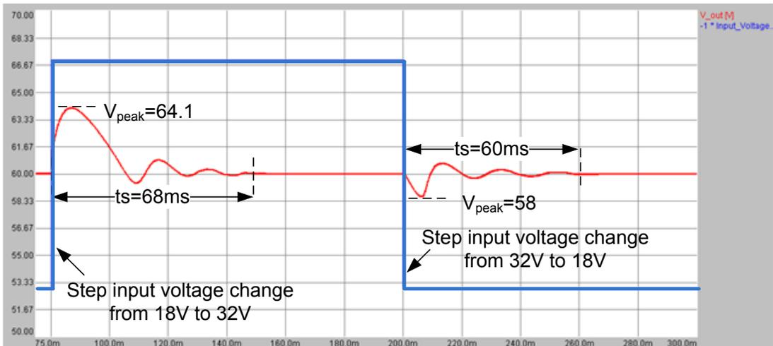
**Figure 4-14** Output voltage during 18V-to-32V-to-18V input voltage transition under 10% load
