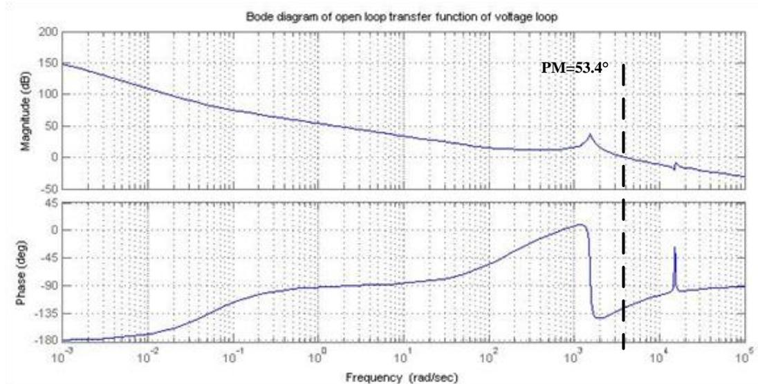
**Figure 4-8** Bode diagram of the compensated open-loop transfer function of voltage loop
