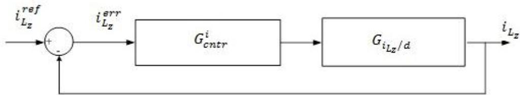
**Figure 4-2** Current loop control block diagram
