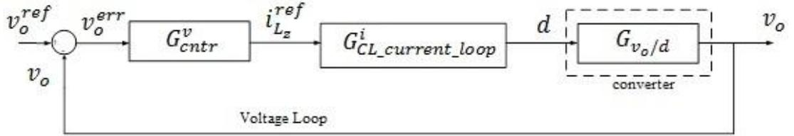
**Figure 4-6** Voltage loop control block diagram
