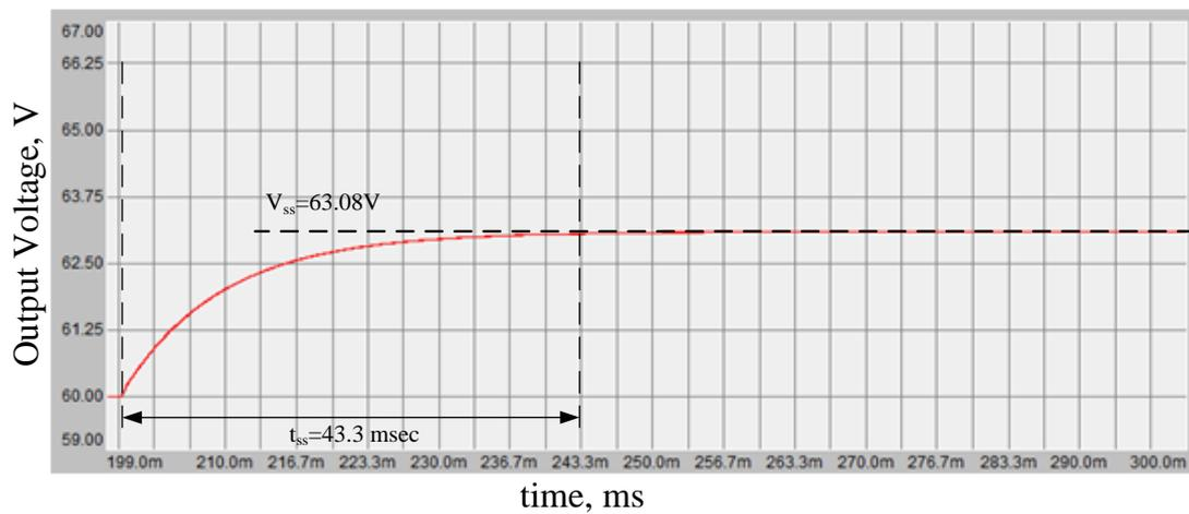
**Figure 3-19** Dynamic response of the circuit model simulated by SIMPLORER to verify input voltage to output voltage transfer function in DCM-2 mode of operation
