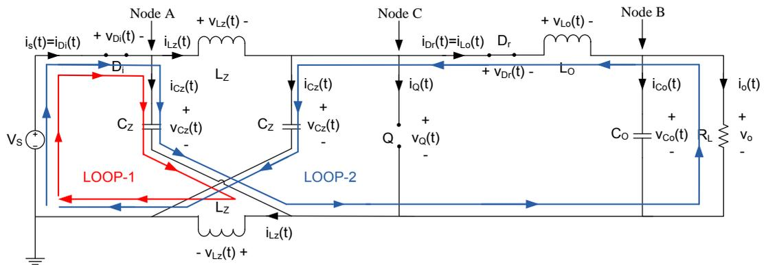
**Figure 2-12** Active loops during mode-3 in DCM-2 operation of Z-source dc/dc converter
