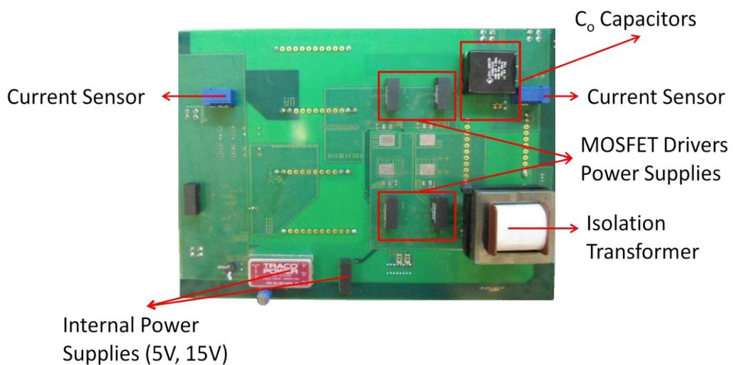
**Figure 5-2** Bottom view of the prototype converter
