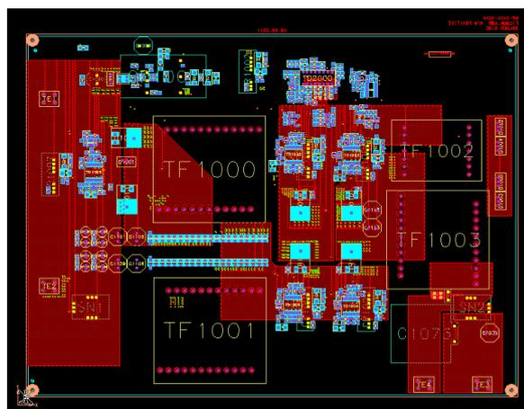
Figure C-2 Bottom side layout of the prototype converter
