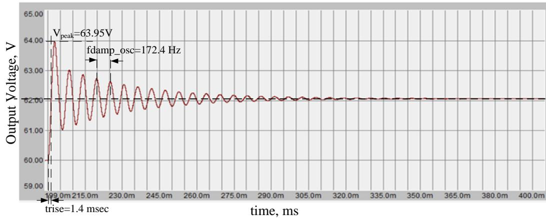
**Figure 3-10** Dynamic response of the circuit model for input voltage to output voltage transfer function,  $G_{v_o/v_s}^{CCM}(s)$  by SIMPLORER
