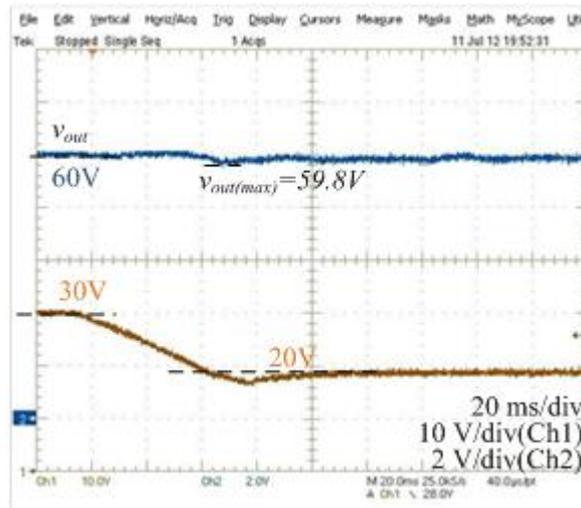
**Figure 5-28** The output voltage response of the converter against a ramp input voltage decay from 30 V to 20 V for  $i_{Load}=0.2$  A
