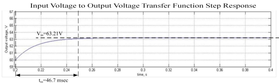
**Figure 3-21** Dynamic response of  $G_{v_o/v_s}^{DCM}(s)$ , input voltage to output voltage transfer function in DCM-2 mode of operation obtained by SIMULINK
