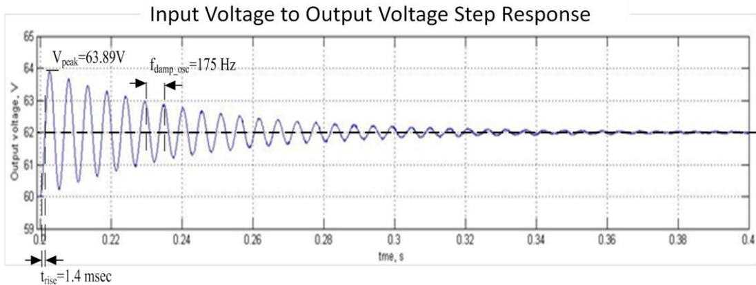
**Figure 3-12** Dynamic response of input voltage to output voltage transfer function in CCM,  $G_{v_o/v_s}^{CCM}(s)$  simulated in SIMULINK
