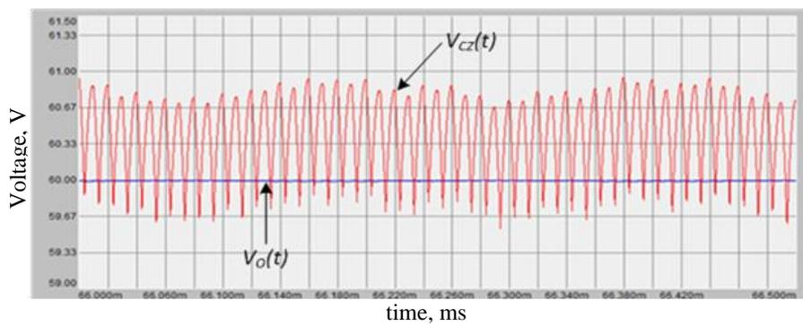
**Figure 3-2** Z-source network capacitor and output voltage in CCM
