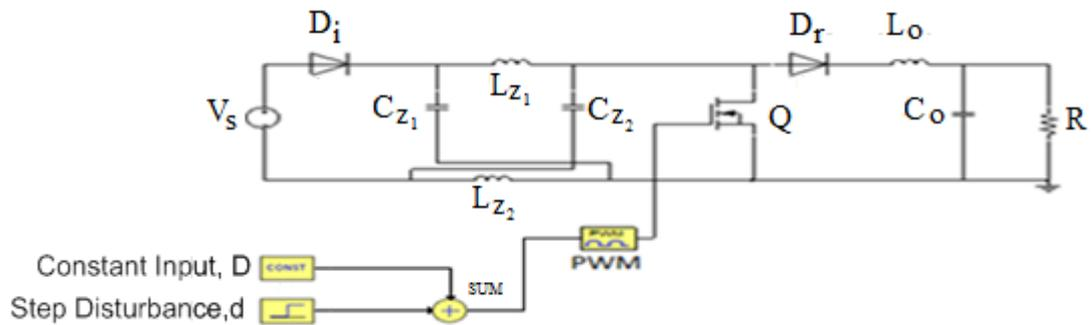
**Figure 3-5** Circuit configurations simulated in order to verify  $G_{v_o/d}^{CCM}(s)$
