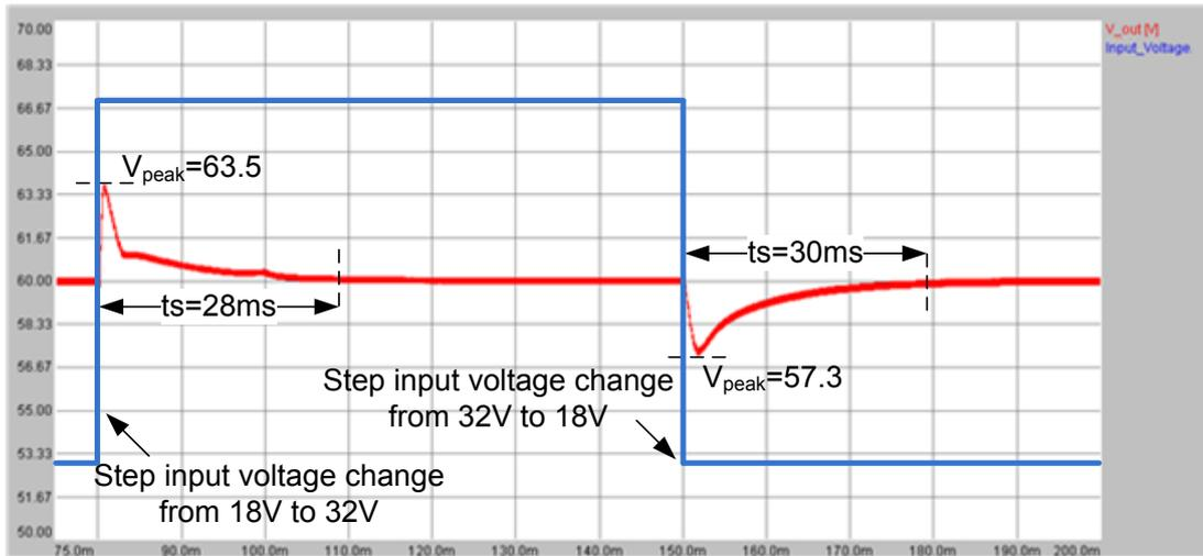
**Figure 4-13** Output voltage during 18V-to-32V-to-18V input voltage transition under full-load
