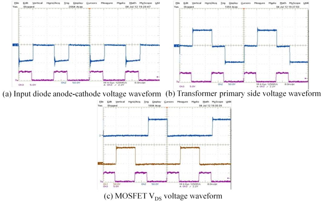
**Figure 5-12** a)  $D_i$  anode-cathode, b) isolation transformer primary side, c)  $Q_1 - Q_3$  cross-pair  $v_{DS}$  voltage waveforms against applied PWM in DCM-2
