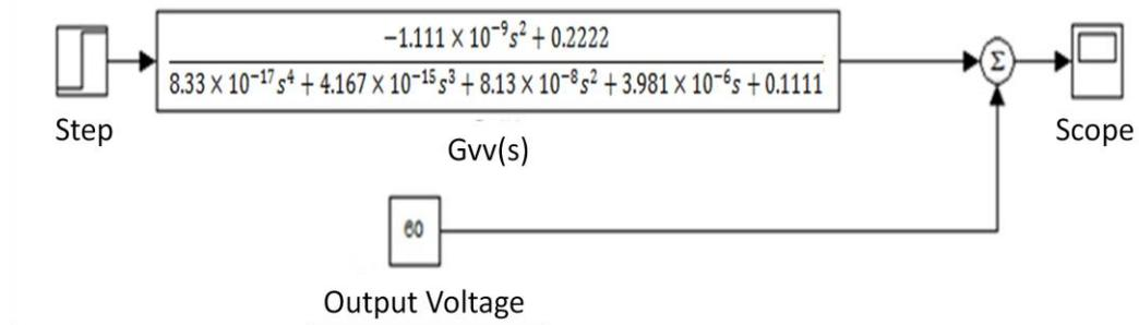
**Figure 3-11** Input voltage to output voltage transfer function in CCM,  $G_{v_o/v_s}^{CCM}(s)$  simulated in SIMULINK
