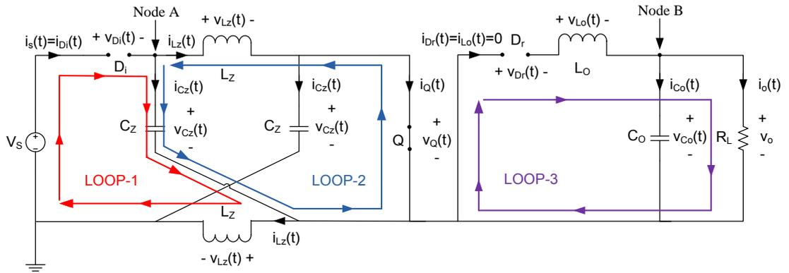
**Figure 2-11** Active loops during mode-2 in DCM-2 operation of Z-source dc/dc converter
