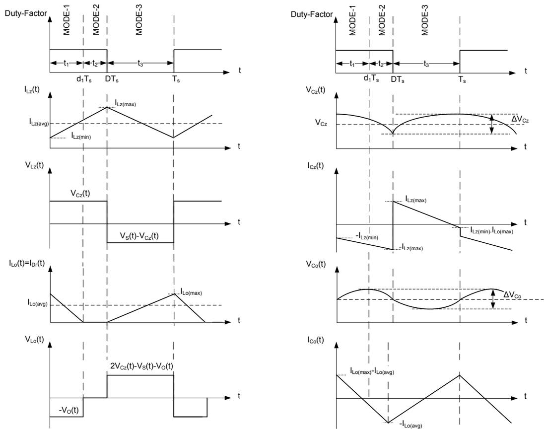
**Figure 2-13** Capacitors ( $C_{Z1}$  and  $C_{Z2}$ ) and inductors ( $L_{Z1}$  and  $L_{Z2}$ ) voltage and current waveforms during the DCM-2 operation of Z-source dc/dc converter
