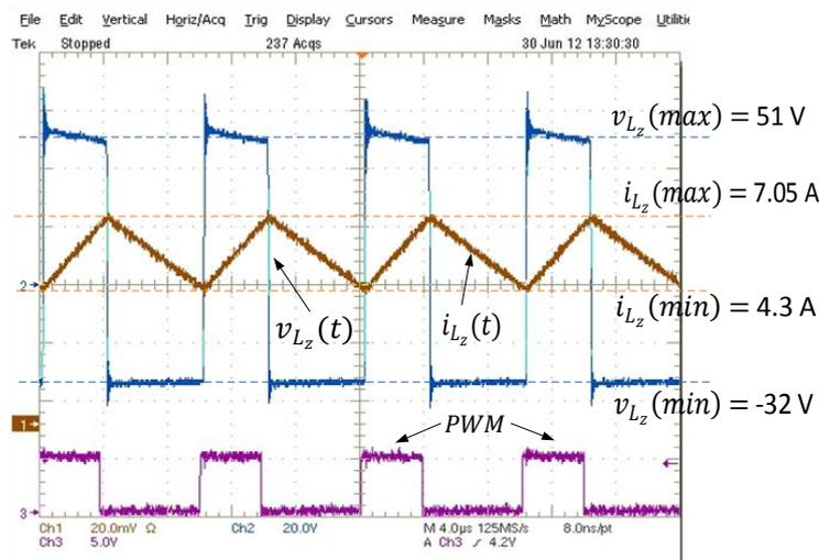
**Figure 5-8**  $L_Z$  current and voltage waveform against applied PWM in DCM-2
