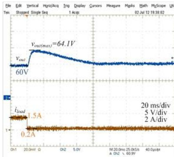
**Figure 5-16** The output voltage response of the converter against a step change of loading from 1.5 A to 0.2 A for  $V_s=30$  V
