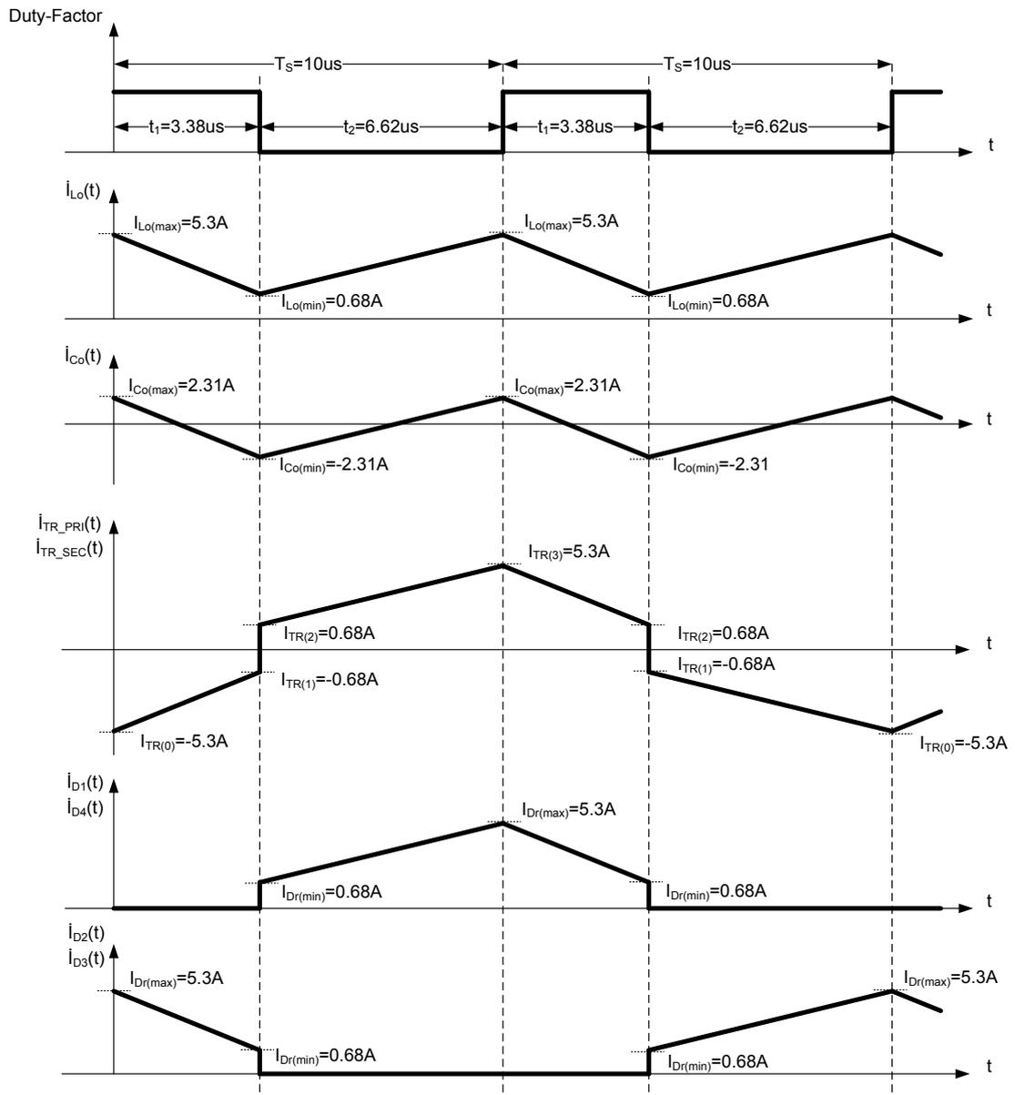
**Figure 5-32** Determination of current waveform magnitudes regarding the circuit elements for open-loop control
