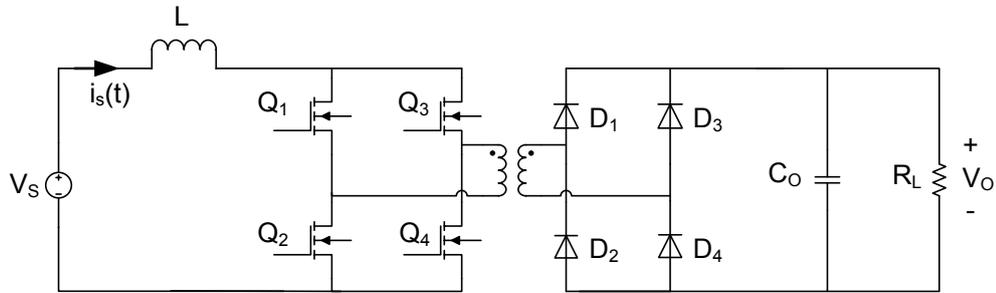
**Figure 1-1** C-fed full-bridge dc/dc converter
