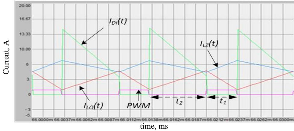
**Figure 3-3** Input diode, Z-source network inductor and output filter inductor current waveforms in CCM
