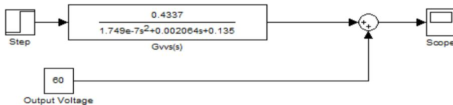
**Figure 3-20** Input voltage to output voltage transfer function in DCM-2 mode of operation simulated in SIMULINK
