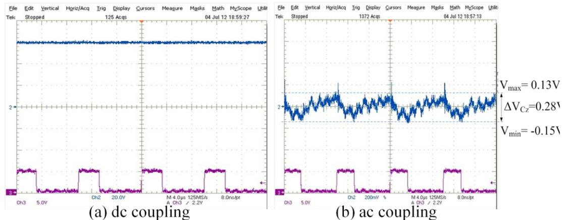
**Figure 5-6** Output voltage waveform against applied PWM in CCM, a) dc coupling, b) ac coupling
