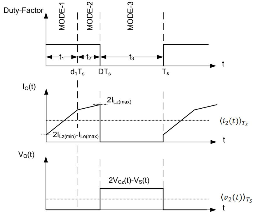
**Figure 2-16** Switch (MOSFET) waveforms over a period
