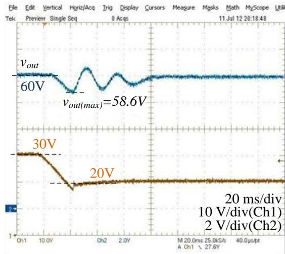
**Figure 5-29** The output voltage response of the converter against a ramp input voltage decay from 30 V to 20 V for  $i_{Load}=1.5$  A
