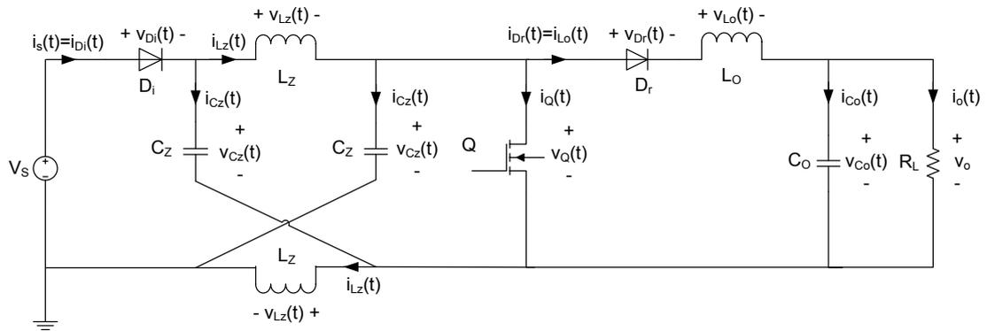
**Figure 2-3** Defining electrical variables in simplified equivalent circuit for Z-source dc/dc converter
