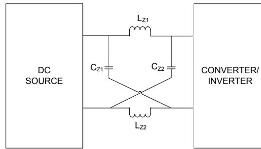
**Figure 1-2** Z-source impedance network
