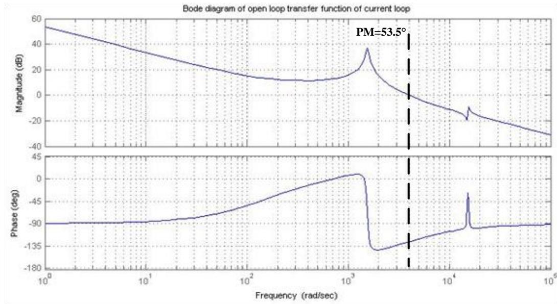
**Figure 4-5** Bode diagram of the compensated open-loop transfer function of current loop
