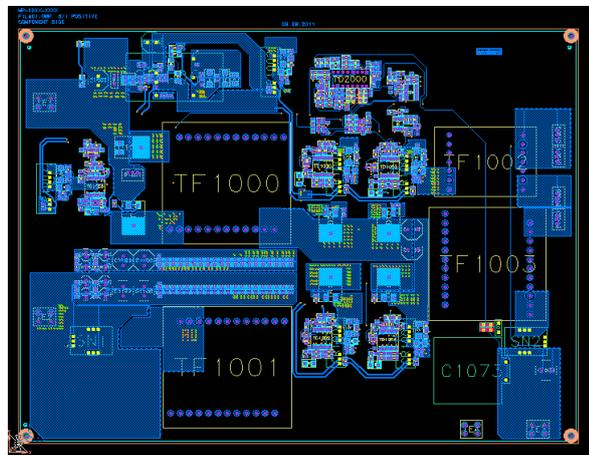
Figure C-1 Top side layout of the prototype converter
