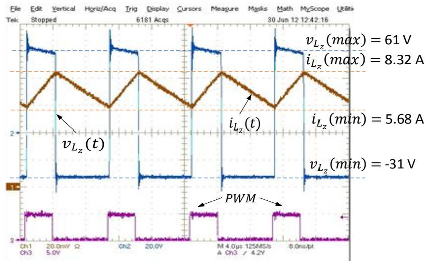
**Figure 5-3** Voltage and current waveforms of  $L_z$  against applied PWM in CCM
