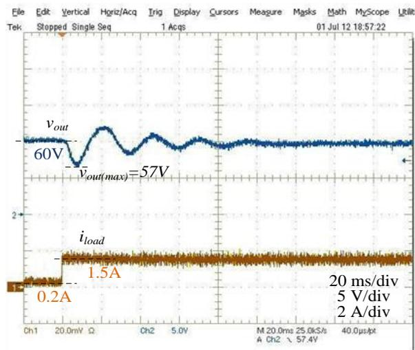
**Figure 5-13** The output voltage response of the converter against a step change of loading from 0.2 A to 1.5 A for  $V_s=20$  V
