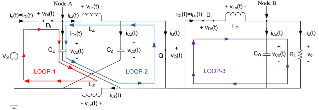
**Figure 2-10** Active loops during mode-1 in DCM-2 operation of Z-source dc/dc converter
