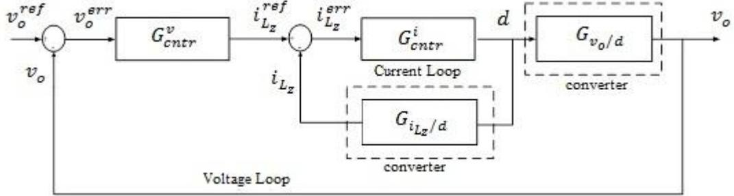
**Figure 4-1** Control block diagram of the converter
