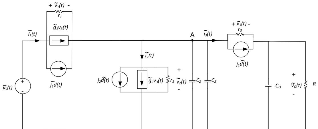
**Figure 2-22** Reduced order small signal ac model of the Z-source dc/dc converter
