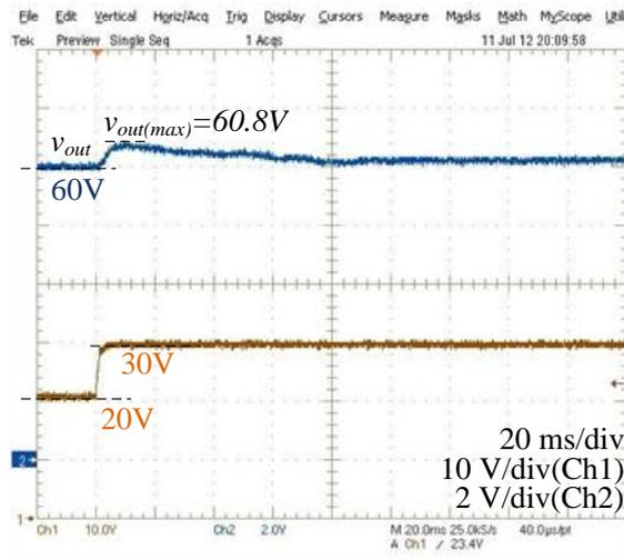
**Figure 5-25** The output voltage response of the converter against a step change of the input voltage from 20 V to 30 V for  $i_{Load}=0.2$  A
