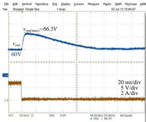
**Figure 5-24** The output voltage response of the converter against a step unloading from 3 A to 0.2 A for  $V_s=30$  V
