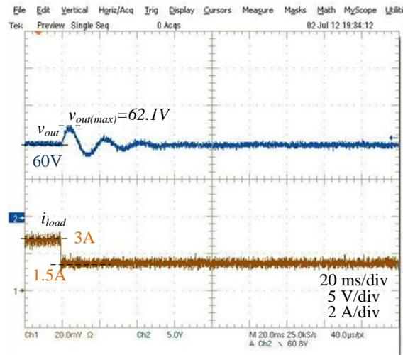
**Figure 5-20** The output voltage response of the converter against a step unloading from 3 A to 1.5 A for  $V_s=30$  V
