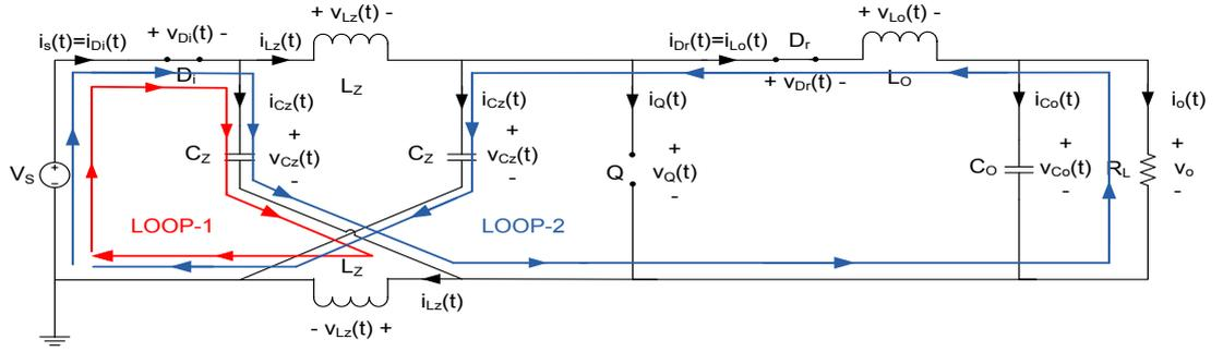
**Figure 2-5** Active loops during mode-2 in CCM operation of Z-source dc/dc converter
