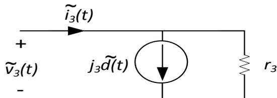
**Figure 2-20** Small signal ac model of the rectification diode
