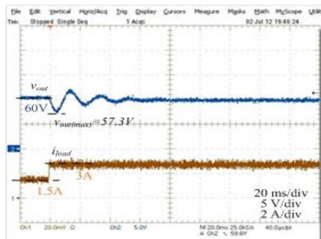
**Figure 5-18** The output voltage response of the converter against a step loading from 1.5 A to 3 A for  $V_s=30$  V
