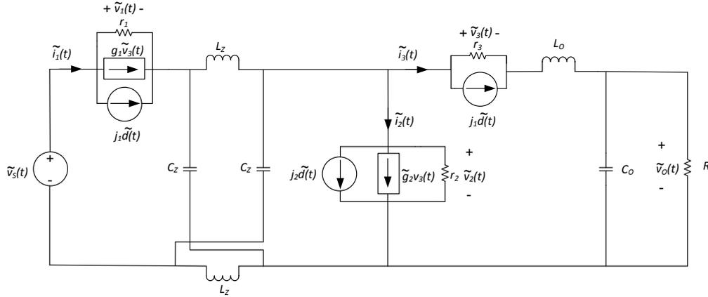
**Figure 2-21** Small signal ac model of the Z-source dc/dc converter in DCM-2 operation
