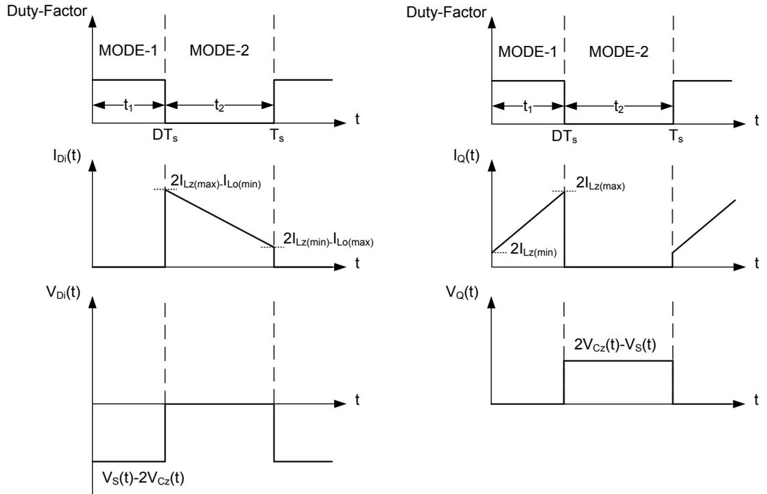
**Figure 2-7** Voltage and current waveforms regarding the switching elements ( $D_i$  and  $Q$ ) during the CCM operation of Z-source dc/dc converter
