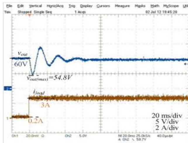
**Figure 5-22** The output voltage responses of the converter against a step increase of loading from 0.2 A to 3 A for  $V_s=30$  V
