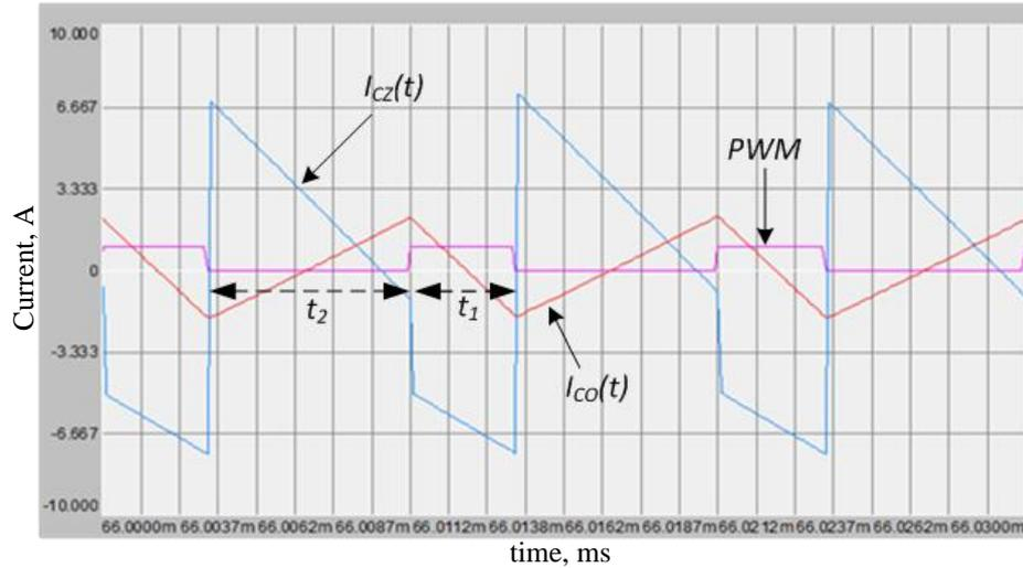
**Figure 3-4** Z-source network capacitor and output filter capacitor current variation in CCM
