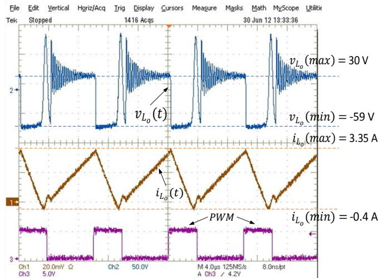
**Figure 5-9**  $L_o$  current and voltage waveform against applied PWM in DCM-2
