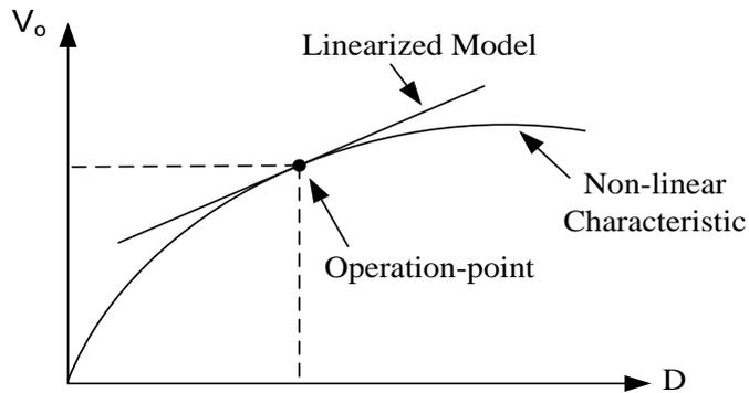
**Figure 2-9** Linearization of non-linear function at an operating point
