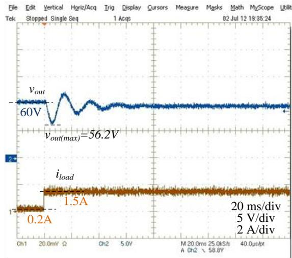
**Figure 5-14** The output voltage response of the converter against a step change of loading from 0.2 A to 1.5 A for  $V_s=30$  V
