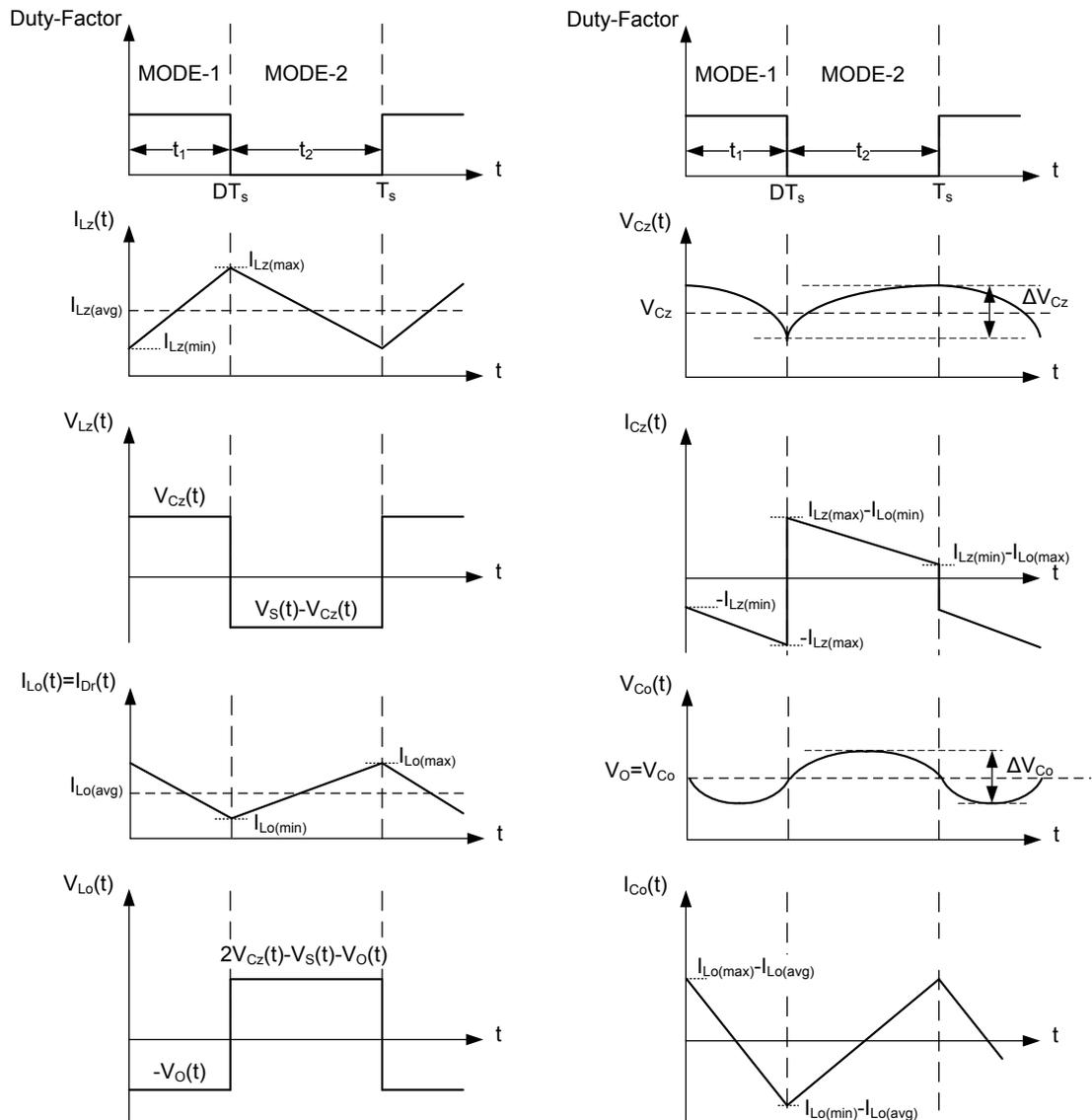
**Figure 2-6** Voltage and current waveforms regarding the circuit elements during the CCM operation of Z-source dc/dc converter
