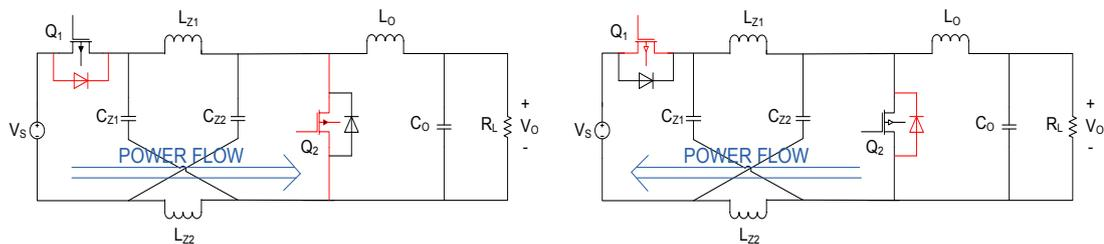
**Figure 1-3** Bidirectional power flow operation
