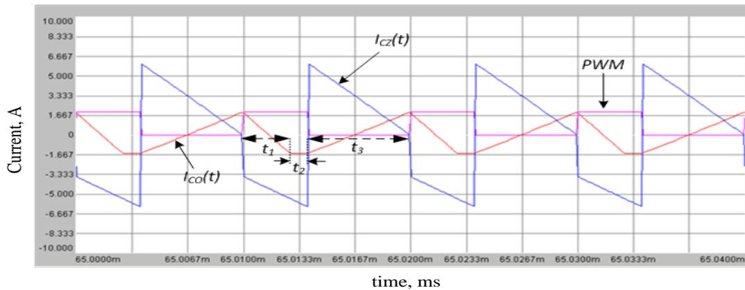
**Figure 3-15** Current waveforms belonging to Z-source network capacitor and output filter capacitor in DCM-2 operation
