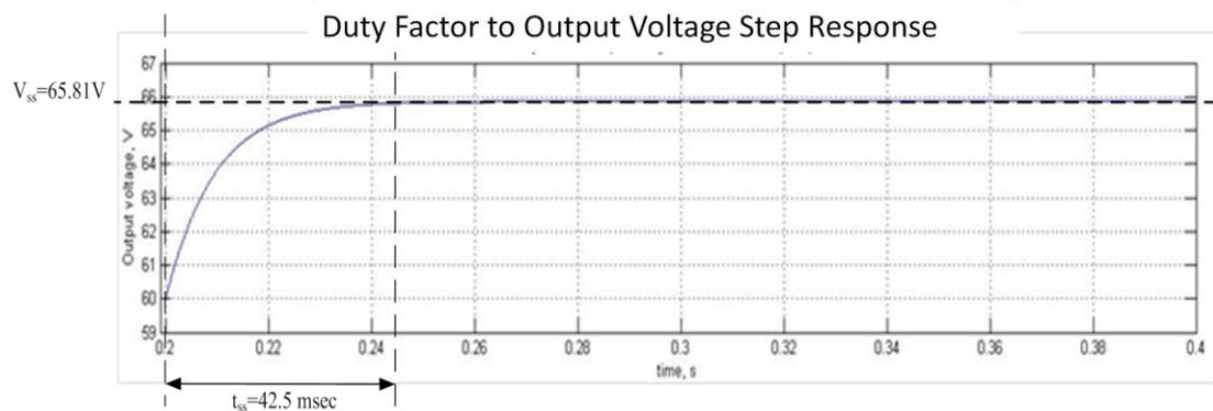
**Figure 3-18** Dynamic response of  $G_{v_o/d}^{DCM}(s)$ , duty factor to output voltage transfer function in DCM-2 mode of operation obtained by SIMULINK
