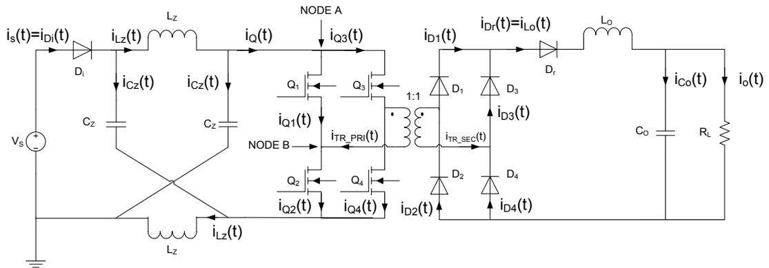
**Figure 5-31** Defining electrical variables for efficiency analysis of Z-source dc/dc converter
