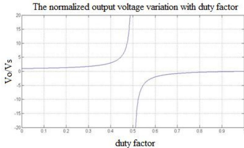
**Figure 2-8** Variation of the normalized output voltage  $V_o/V_s$  with duty factor,  $D$
