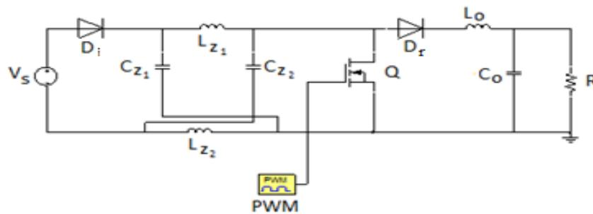
**Figure 3-1** Simplified circuit diagram of Z-source dc/dc converter for CCM simulation
