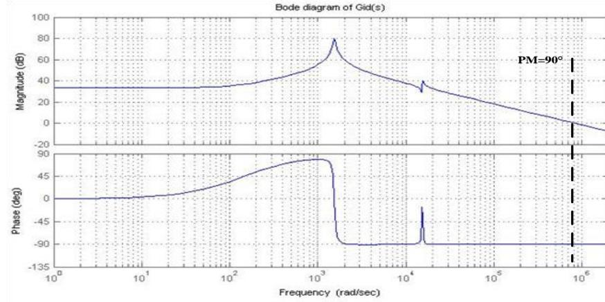
**Figure 4-4** Bode diagram of  $G_{i_{Lz}/d}(s)$
