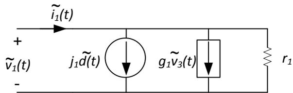
**Figure 2-18** Small signal ac model of the input diode
