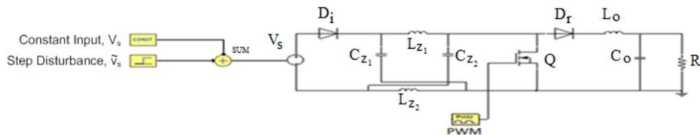
**Figure 3-9** Circuit model simulated in SIMPLORER in order to verify input voltage to output voltage transfer function,  $G_{v_o/v_s}^{CCM}(s)$
