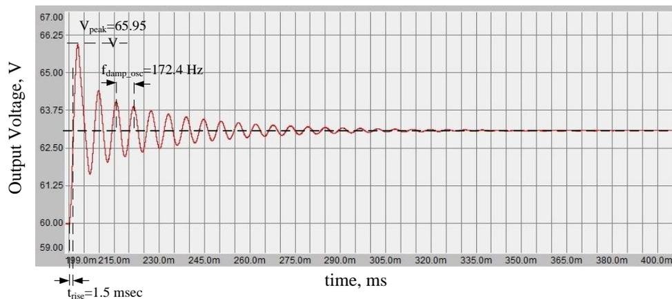
**Figure 3-6** Dynamic response of the circuit model simulated in SIMPLORER to verify duty factor to output voltage transfer function in CCM
