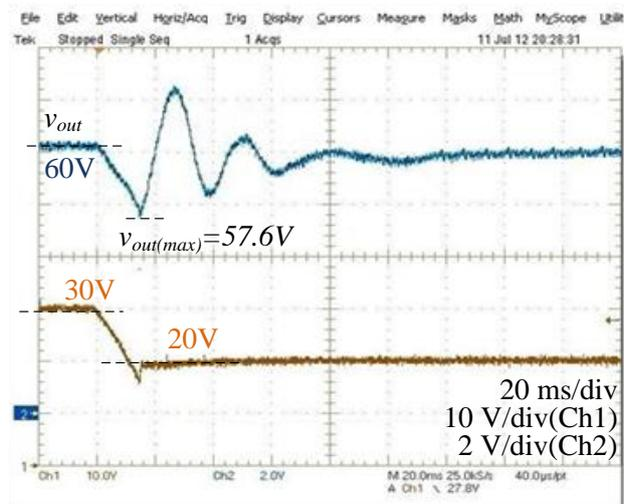
**Figure 5-30** The output voltage response of the converter against a ramp input voltage decay from 30 V to 20 V for  $i_{Load}=3$  A
