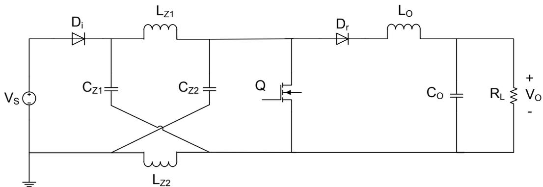
**Figure 2-2** Simplified circuit diagram for Z-source dc/dc converter
