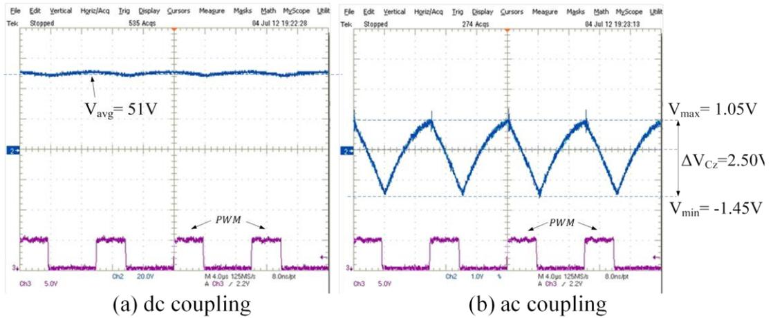
**Figure 5-10**  $C_z$  voltage waveform against applied PWM in DCM-2, a) dc coupling, b) ac coupling
