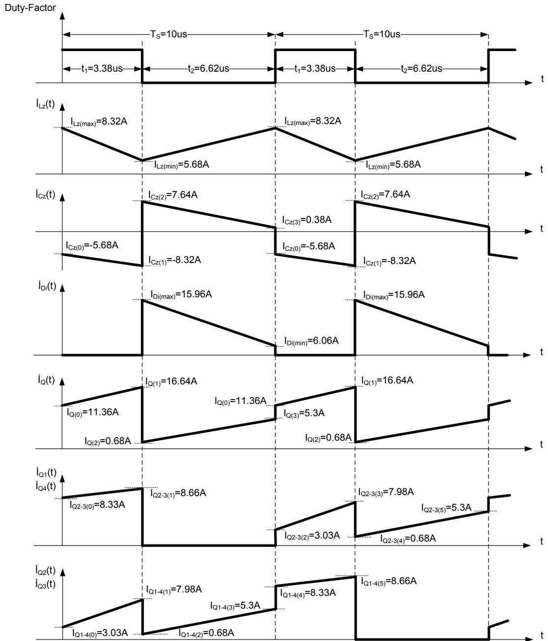
**Figure 5-33** Determination of current waveform magnitudes regarding the circuit elements for open-loop control
