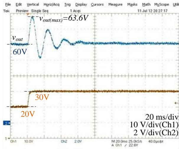
**Figure 5-27** The output voltage response of the converter against a step change of input voltage from 20 V to 30 V for  $i_{Load}=3$  A
