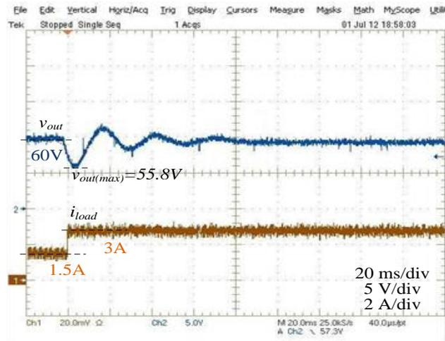
**Figure 5-17** The output voltage response of the converter against a step loading from 1.5 A to 3 A for  $V_s=20$  V
