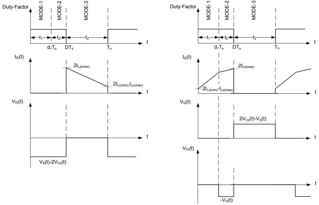
**Figure 2-14** Switching elements ( $D_i$  and  $Q$ ) voltage and current waveforms during the CCM operation of Z-source dc/dc converter
