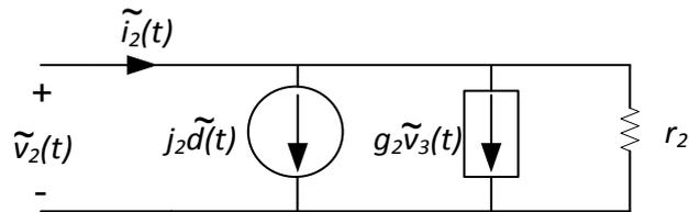
**Figure 2-19** Small signal ac model of the switch
