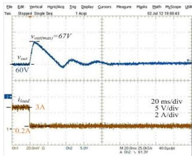
**Figure 5-23** The output voltage response of the converter against a step unloading from 3 A to 0.2 A for  $V_s=20$  V
