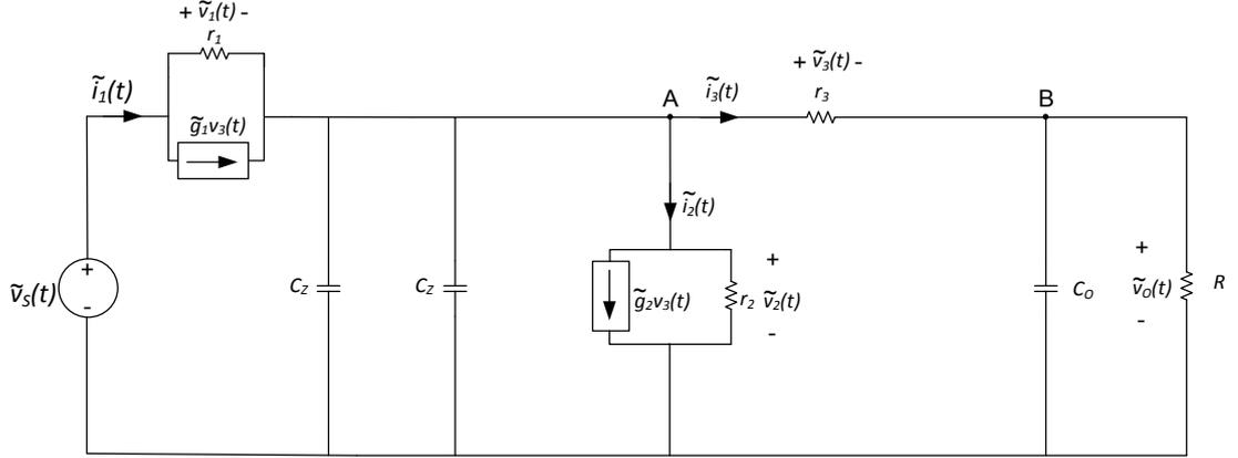
**Figure 2-24** Small signal ac model for determination of  $G_{v_o/v_s}^{DCM}(s)$  in DCM-2 operation
