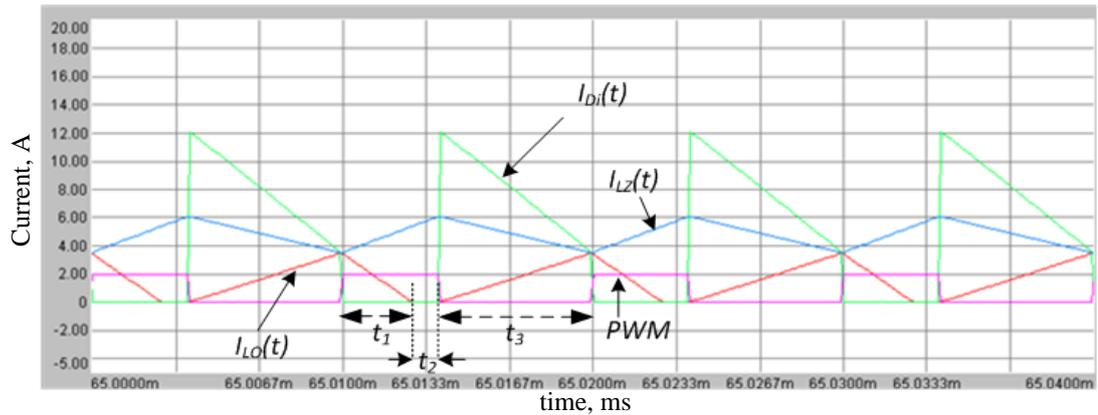
**Figure 3-14** Current waveforms belonging to input diode, Z-source network inductor and output filter inductor in DCM-2 operation
