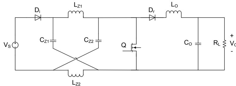
**Figure 1-4** Z-source dc/dc converter with filter inductor and capacitor
