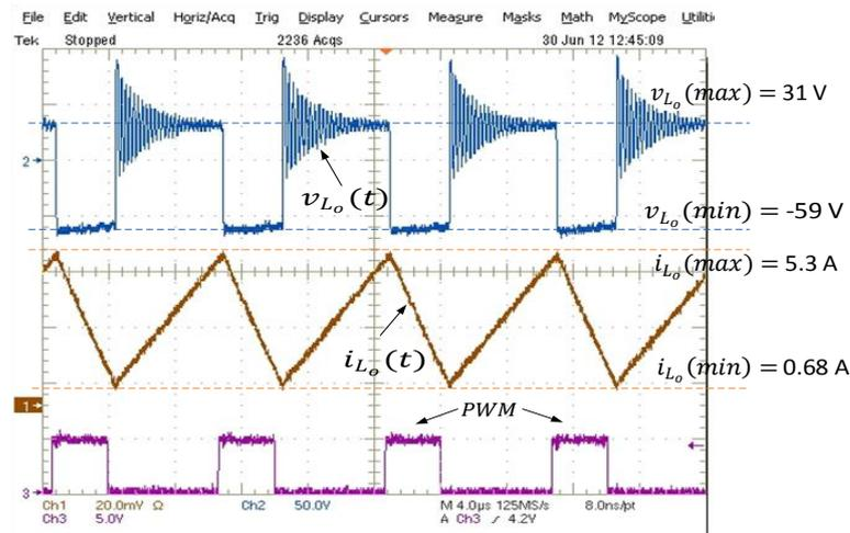
**Figure 5-4** Voltage and current waveforms of  $L_o$  against applied PWM in CCM
