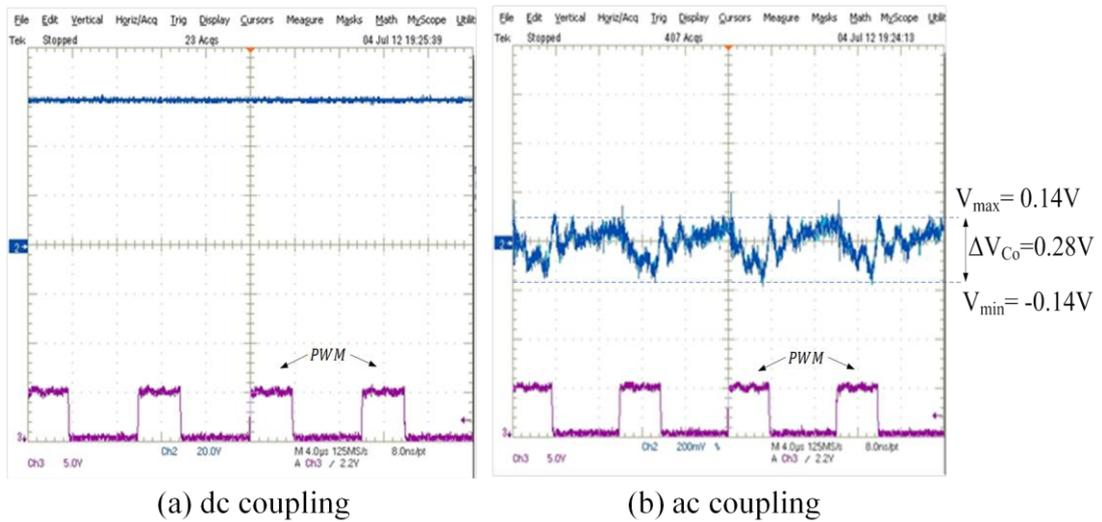
**Figure 5-11** The output voltage waveform against applied PWM in DCM-2, a) dc coupling, b) ac coupling
