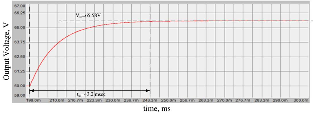
**Figure 3-16** Dynamic response of the circuit model simulated in SIMPLORER to verify duty factor to output voltage transfer function in DCM-2 of operation
