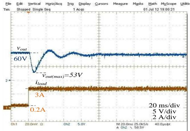
**Figure 5-21** The output voltage response of the converter against a step increase of loading from 0.2 A to 3 A for  $V_s=20$  V
