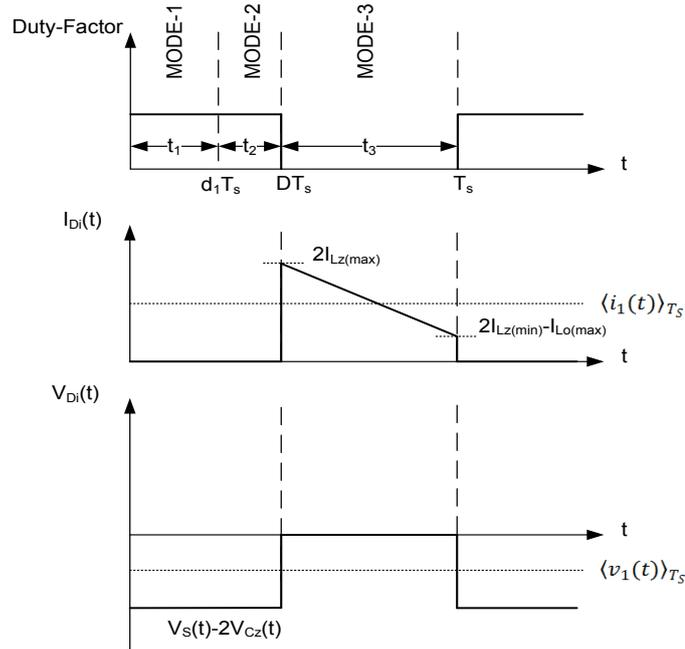
**Figure 2-15** Input diode voltage and current waveforms over a period
