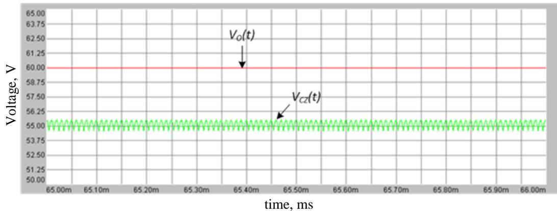
**Figure 3-13** Z-source network capacitor voltage and the output voltage in DCM-2 mode of operation
