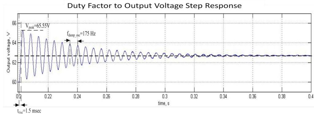
**Figure 3-8** Dynamic response of  $G_{v_o/d}^{CCM}(s)$ , duty factor to output voltage transfer function in CCM obtained by SIMULINK
