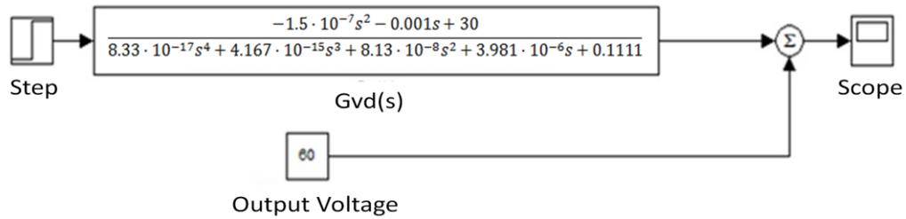
**Figure 3-7** Duty factor to output voltage transfer function in CCM simulated in SIMULINK
