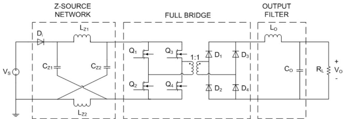
**Figure 2-1** Z-source full bridge dc/dc converter
