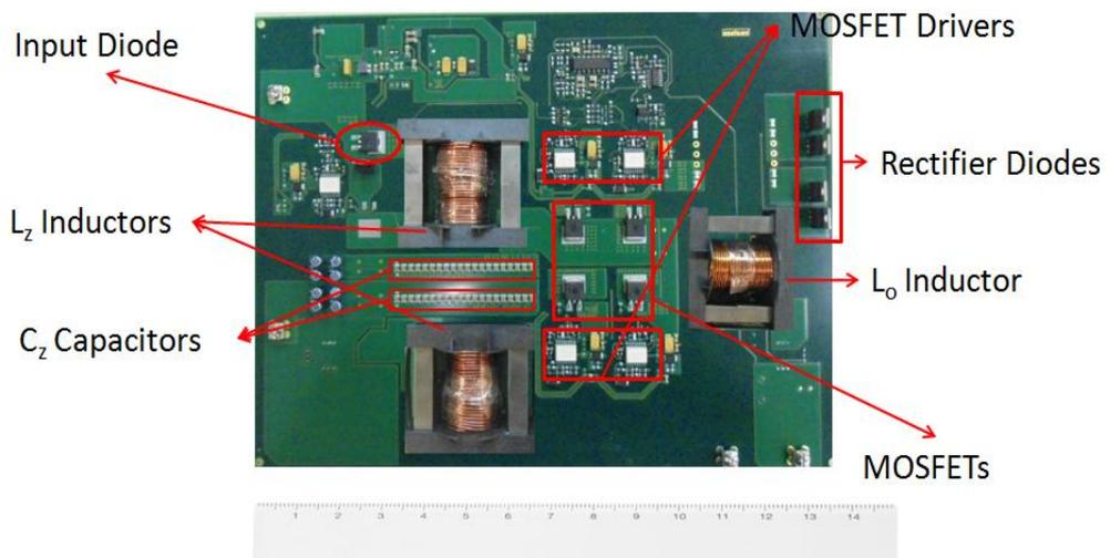
**Figure 5-1** Top view of the prototype converter
