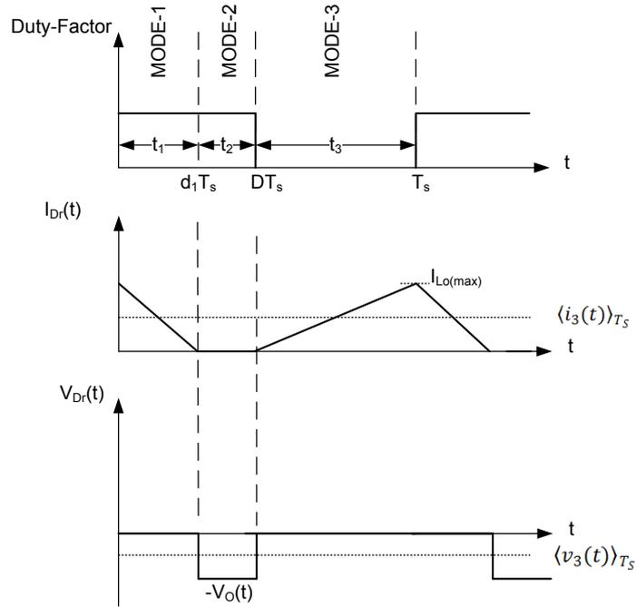
**Figure 2-17** Rectification diode waveforms over a period
