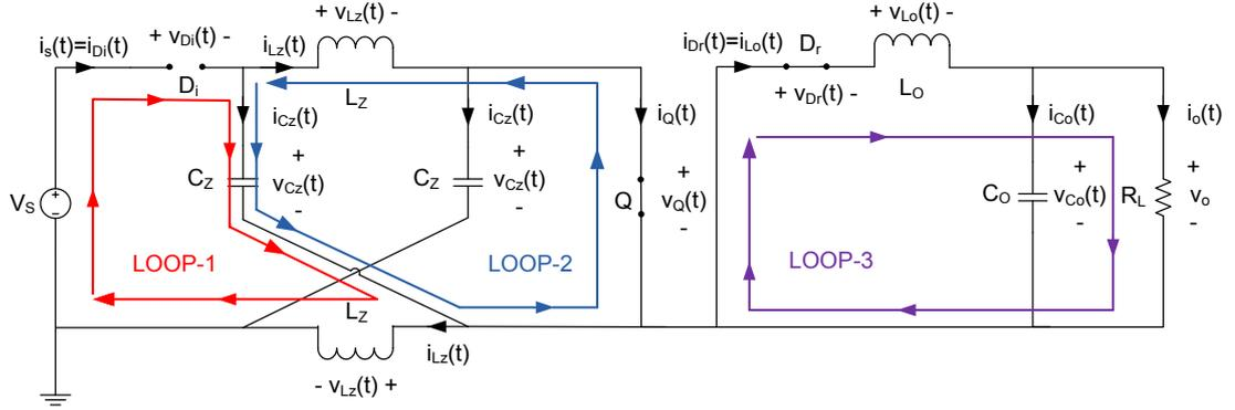
**Figure 2-4** Active loops during mode-1 in CCM operation of Z-source dc/dc converter
