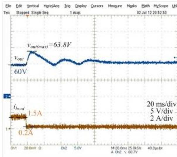
**Figure 5-15** The output voltage response of the converter against a step change of loading from 1.5 A to 0.2 A for  $V_s=20$  V
