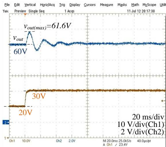
**Figure 5-26** The output voltage response of the converter against a step change of the input voltage from 20 V to 30 V for  $i_{Load}=1.5$  A
