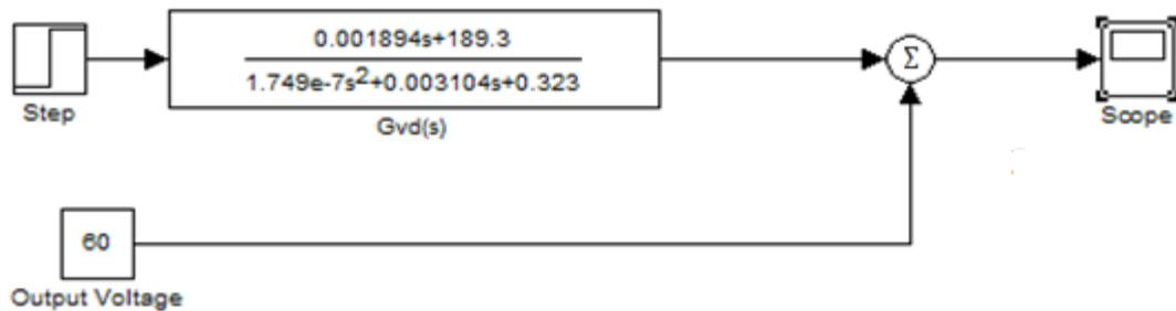
**Figure 3-17** Duty factor to output voltage transfer function in DCM-2 of operation simulated in SIMULINK
