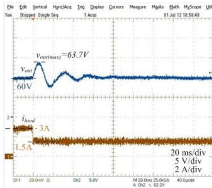
**Figure 5-19** The output voltage response of the converter against a step unloading from 3 A to 1.5 A for  $V_s=20$  V
