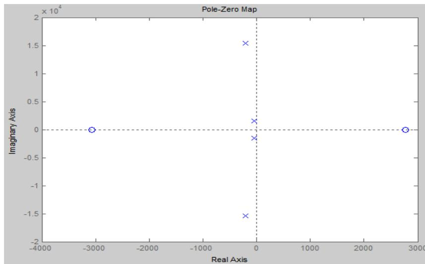
**Figure 4-7** Pole-zero map of  $G_{V_o/d}(s)$
