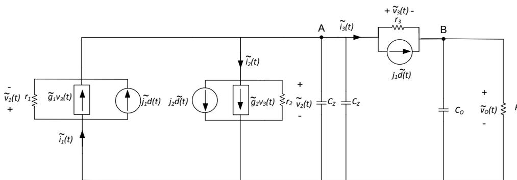
**Figure 2-23** Small signal ac model for determination of  $G_{v_o/d}^{DCM}(s)$  in DCM-2 operation
