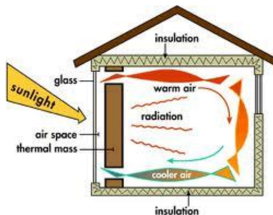
Figure 2.6 Trombe Wall Principle
