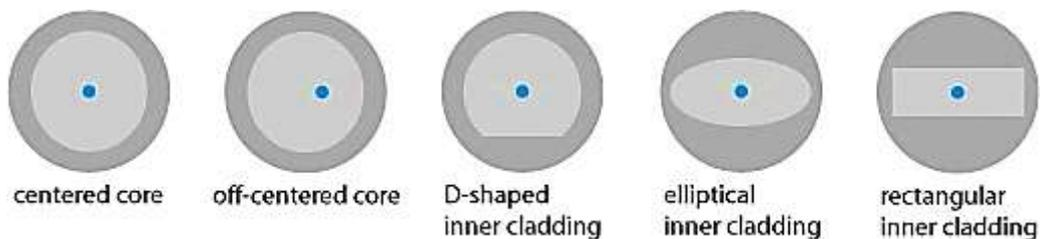
Figure 3.7: Various designs of double-clad fibers. The fiber core is shown in blue, the inner cladding in light gray, and the outer cladding in dark gray [54].
