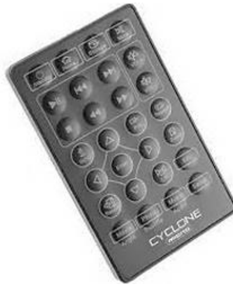
Figure 1.3: Example of a poor designed remote control with similar buttons only ( http://www.memorybits.org.uk/sumvision-cyclone-micro-remote-control/ retrieved 18 July 2012)
