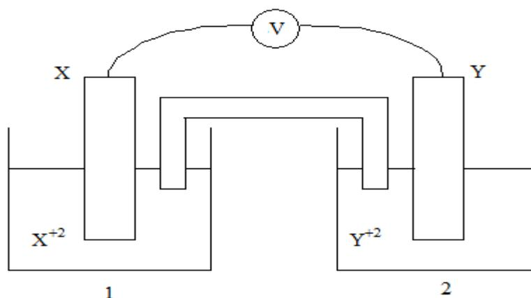
**Figure 20.** Drawing of electrochemical cell including X and Y electrodes and their solutions
