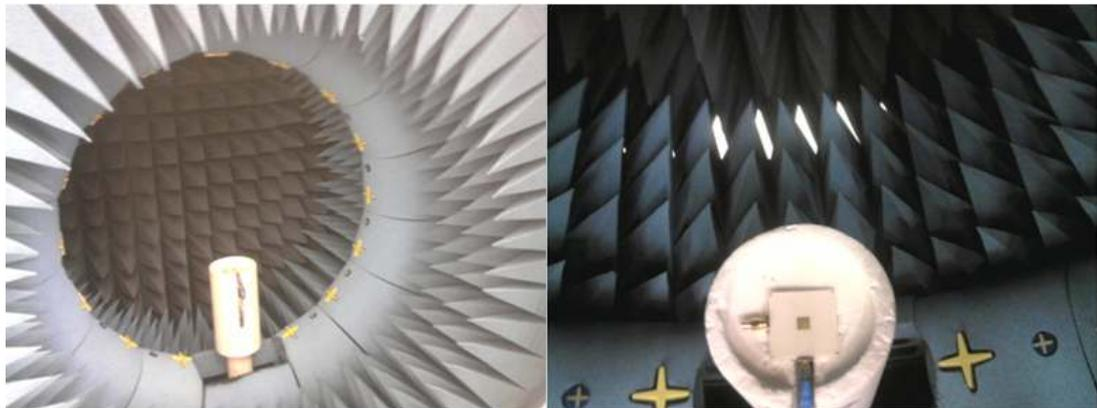
**Figure 4. 5 Far Field Pattern Measurement Set-up.**
