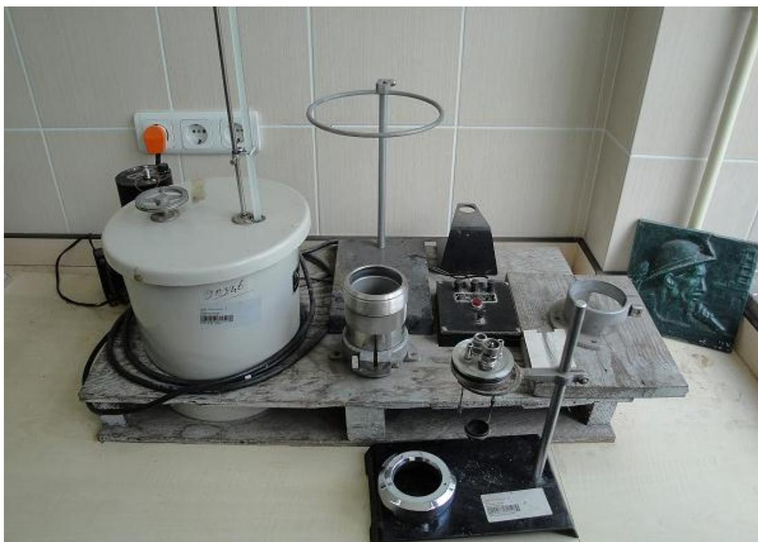
Fig. 3.17 Oxygen bomb calorimeter set up
