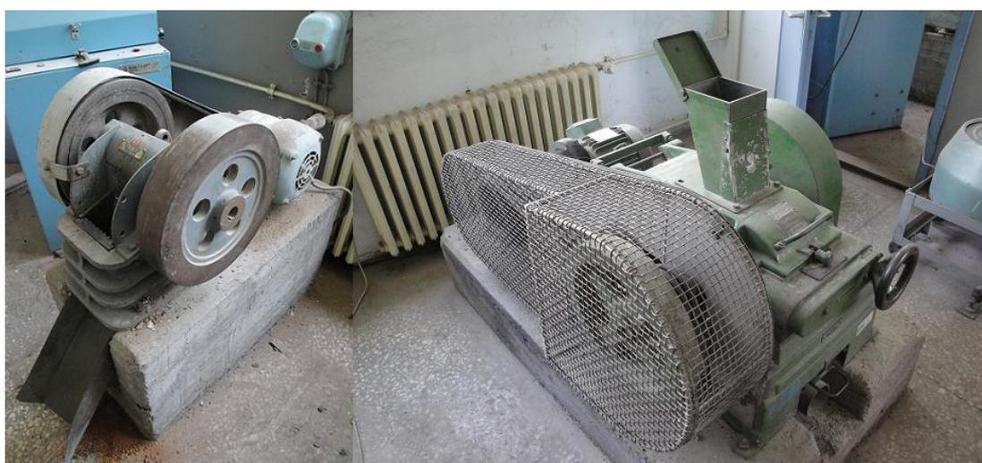
Fig. 3.2 Jaw (left) and roll (right) crushers
