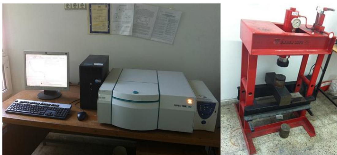
Fig. 3.14 X-ray Fluorescence SPECTRO iQ (left) and the hydraulic press (right)
