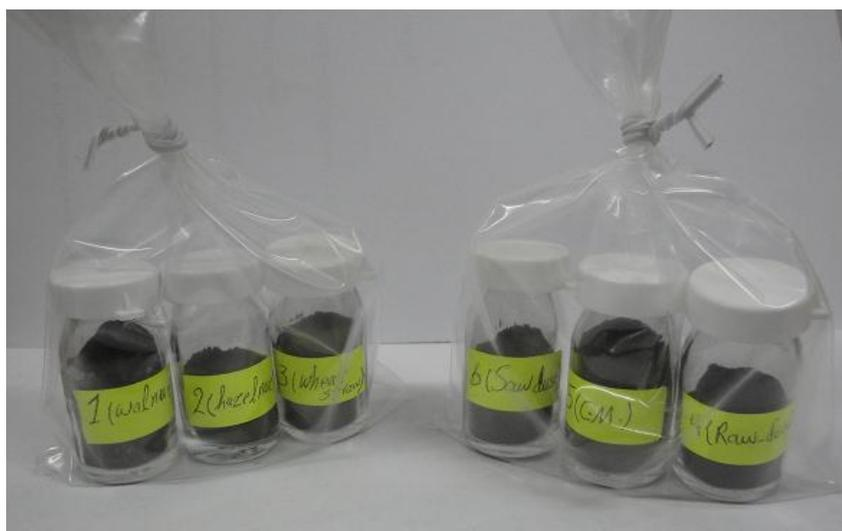
Fig. 3.4 Impregnated Kangal lignite samples with biomass ash used in TGA-FTIR tests
