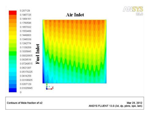
Figure 4.14 Contours of mole fraction of O<sub>2</sub> at the cathode-electrolyte surface
