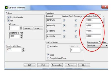
Figure A.15 A screen shot for determining the residuals
