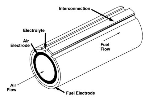
Figure 1.3 Tubular SOFC design configuration [14]
