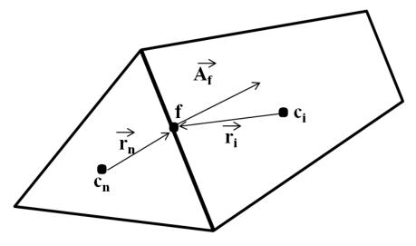
Figure 3.4 Schematic of 2-D control volume [53]
