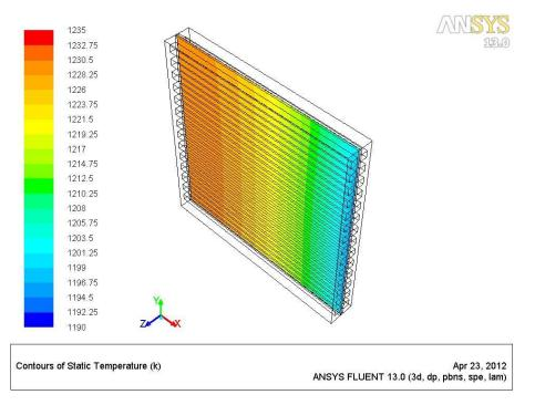
Figure 5.3 Temperature profile at the anode/cathode-electrolyte surface of Co-Flow design
