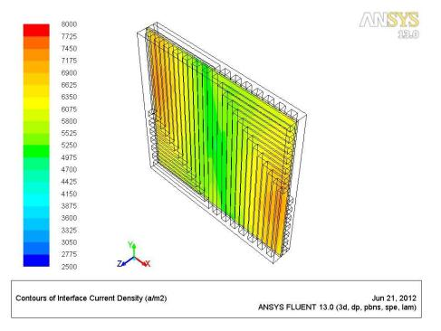
Figure 5.11 Interface current density at the anode/cathode-electrolyte surface for G-2 design
