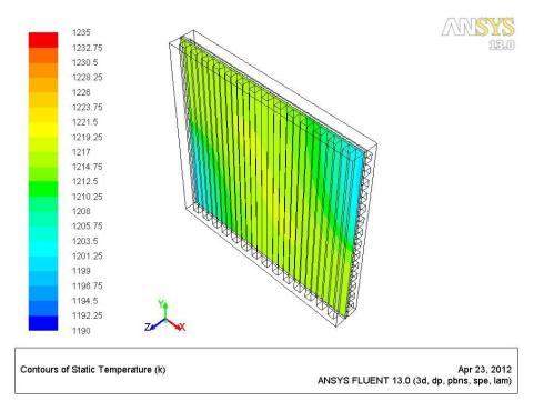
Figure 5.7 Temperature profile at the anode/cathode-electrolyte surface of G-3 design
