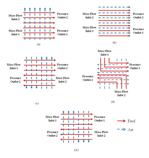
Figure 5.13 Traditional and developed geometries for recycling: (a) Cross-Flow, (b) Co-Flow, (c) G-1, (d) G-2, (e) G-3
