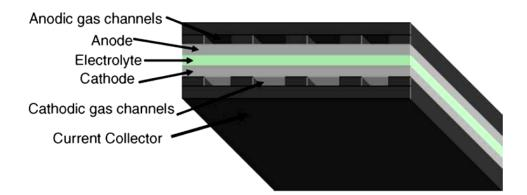
Figure 1.4 Flat planar SOFC design configuration [15]
