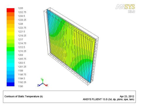
Figure 5.5 Temperature profile at the anode/cathode-electrolyte surface of G-1 design
