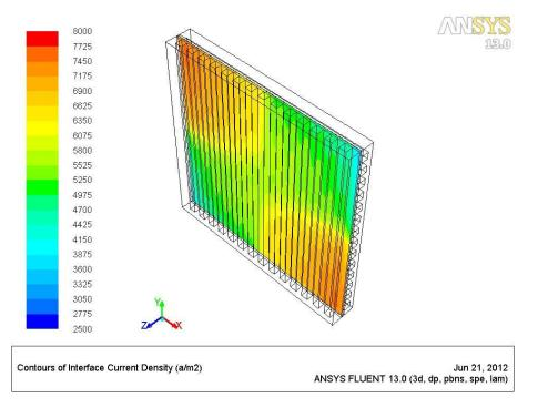
Figure 5.10 Interface current density at the anode/cathode-electrolyte surface for G-1 design
