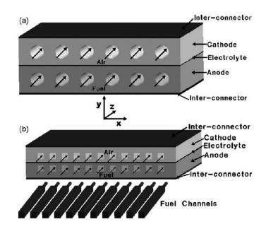
Figure 2.3 Schematic views of two types of planar PES-SOFC: (a) type-I (b) type-II [37]
