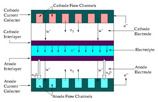
Figure 1.1 Schematic of a Solid Oxide Fuel Cell [5]
