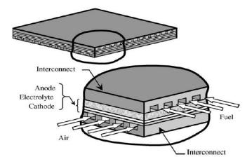
Figure 4.7 SOFC single cell Cross-Flow arrangements [54]
