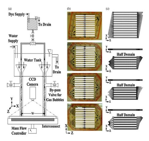
Figure 2.4 (a) Schematic of the hydraulic platform for flow visualizations and velocity measurements, (b) Four different designs, (c) Corresponding four numerical models [39]
