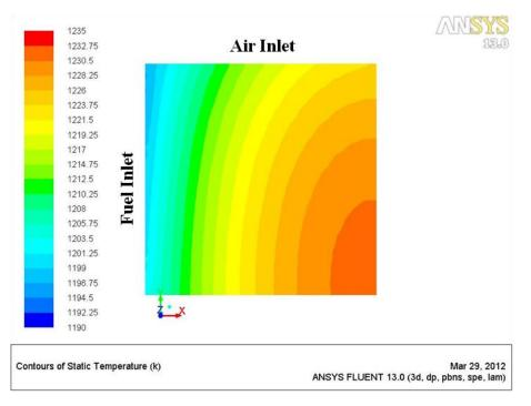
Figure 4.11 Contours of temperature at the anode/cathode-electrolyte surface
