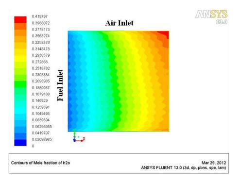
Figure 4.12 Contours of mole fraction of H<sub>2</sub>O at the anode-electrolyte surface
