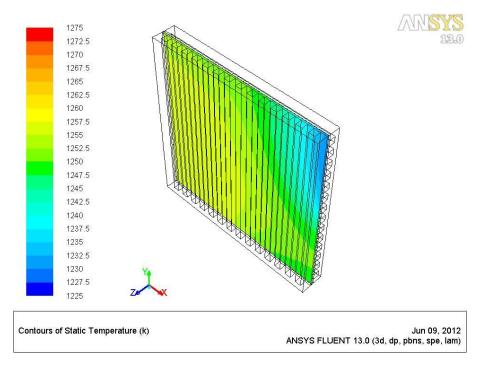
Figure 5.19 Temperature profile at the anode/cathode-electrolyte surface of G-3 stack design with recycling
