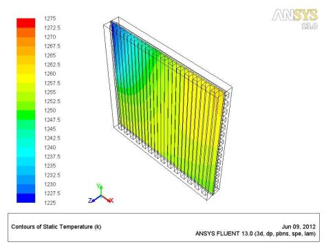
Figure 5.17 Temperature profile at the anode/cathode-electrolyte surface of G-1 stack design with recycling
