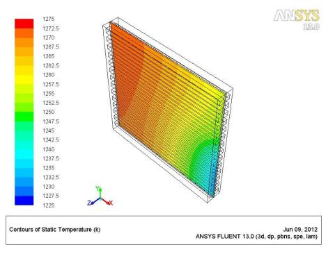
Figure 5.14 Temperature profile at the anode/cathode-electrolyte surface of Co-Flow stack design with recycling
