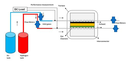
Figure 4.4 Schematic of experimental setup
