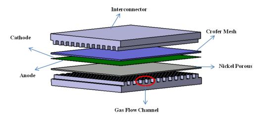
Figure 3.3 Schematic of SOFC
