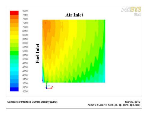
Figure 4.15 Contours of interface current density at the anode/cathodeelectrolyte surface
