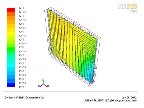
Figure 5.18 Temperature profile at the anode/cathode-electrolyte surface of G-2 stack design with recycling
