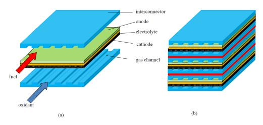
Figure 1.8 (a) SOFC single cell (b) SOFC stack with 3 cells [6]
