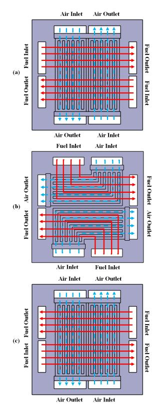
Figure 5.2 Interconnector designs for developed flow arrangements: (a) G-1, (b) G-2, (c) G-3
