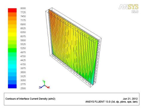
Figure 5.9 Interface current density at the anode/cathode-electrolyte surface for Cross-Flow design
