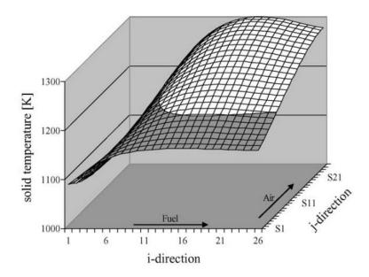
Figure 2.2 Temperature distributions on the cell active area for Cross-Flow arrangement [36]
