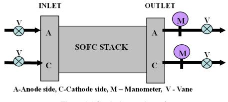
Figure 4.5 Gas leak test schematic
