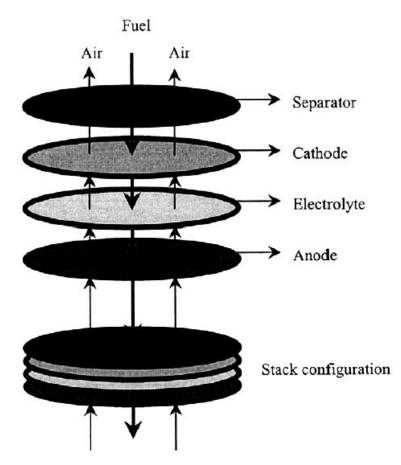
Figure 1.5 Radial planar SOFC design configuration [1]
