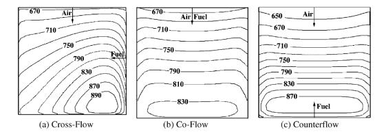
Figure 2.1 Temperature distributions on the cell active area for (a) Cross-Flow, (b) Co-Flow and (c) Counter-Flow arrangements [33]
