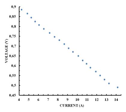
Figure 4.6 Current-voltage characteristic of the SOFC single cell
