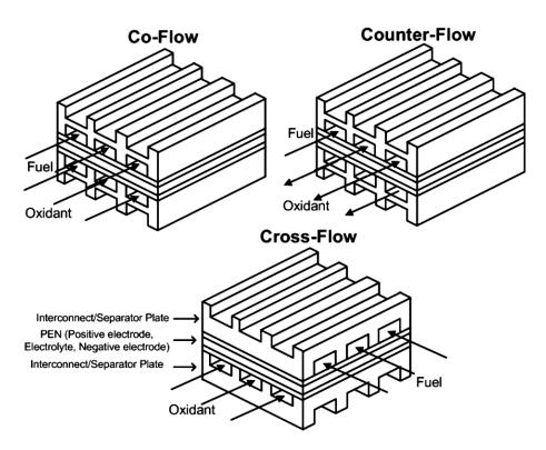
Figure 1.7 Different flow arrangements for flat-planar SOFC design [25]
