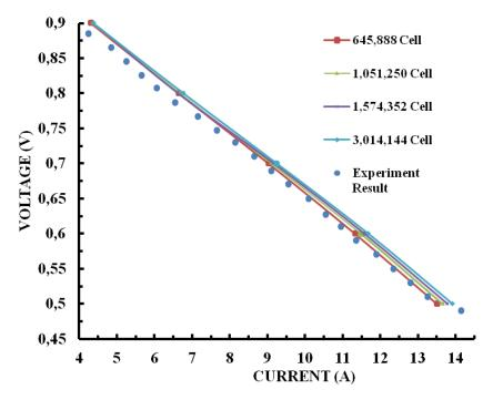
Figure 4.8 Comparison of the model and experimental results for different cell numbers
