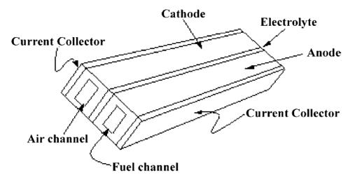
Figure 1.2 Monolithic SOFC design configuration [13]
