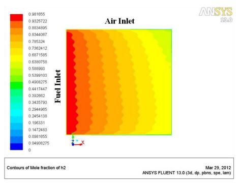
Figure 4.13 Contours of mole fraction of H<sub>2</sub> at the anode-electrolyte surface
