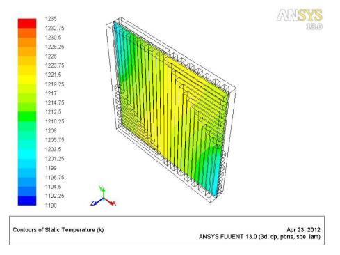
Figure 5.6 Temperature profile at the anode/cathode-electrolyte surface of G-2 design
