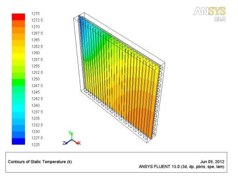
Figure 5.15 Temperature profile at the anode/cathode-electrolyte surface of Cross-Flow-1 stack design with recycling
