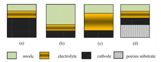
Figure 1.6 SOFC PEN structure configurations (a) cathode supported (b) anode supported (c) electrolyte supported (d) porous substrate supported [6]
