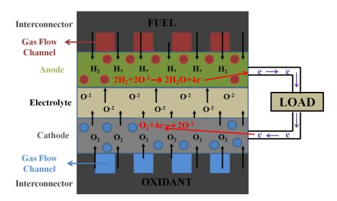
Figure 3.1 SOFC working principle
