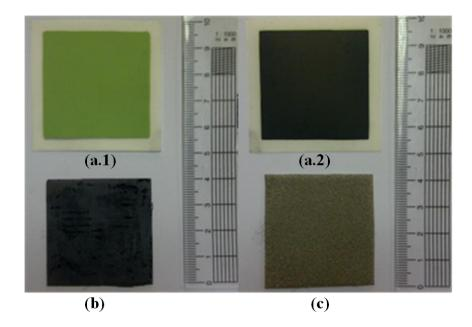
Figure 4.2 (a.1) and (a.2) SOFC membrane (b) crofer mesh (c) nickel porous
