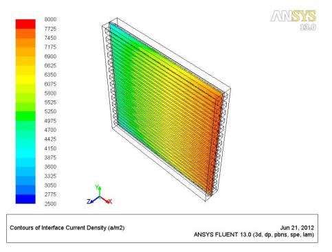
Figure 5.8 Interface current density at the anode/cathode-electrolyte surface for Co-Flow design
