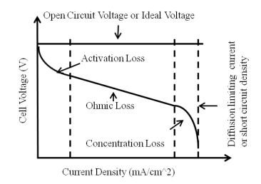
Figure 3.2 Polarization types
