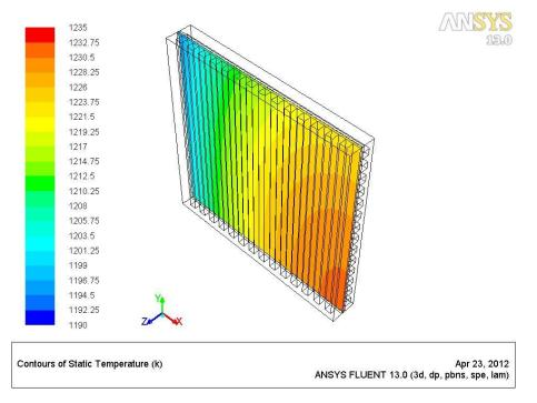
Figure 5.4 Temperature profile at the anode/cathode-electrolyte surface of Cross-Flow design
