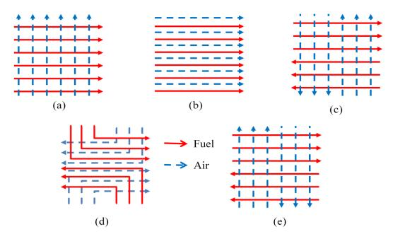
Figure 5.1 Traditional [(a) and (b)] and developed geometries [(c), (d) and (e)]: (a) Cross-Flow, (b) Co-Flow, (c) G-1, (d) G-2, (e) G-3
