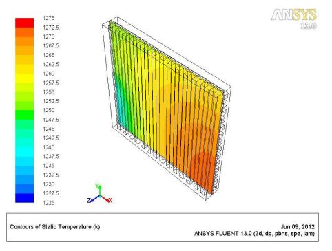
Figure 5.16 Temperature profile at the anode/cathode-electrolyte surface of Cross-Flow-2 stack design with recycling
