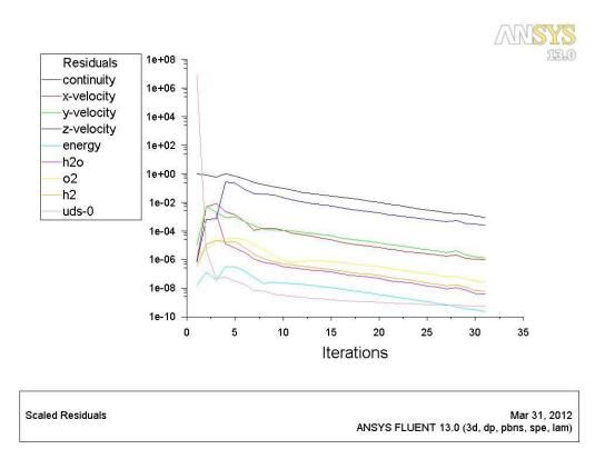
Figure 4.10 Scaled residuals for the selected equations
