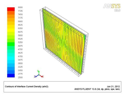
Figure 5.12 Interface current density at the anode/cathode-electrolyte surface for G-3 design
