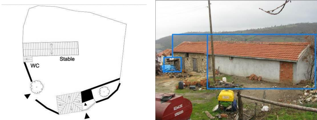
Figure 63. WC and stable addition at the courtyard of Hasbiye Akboğa House
