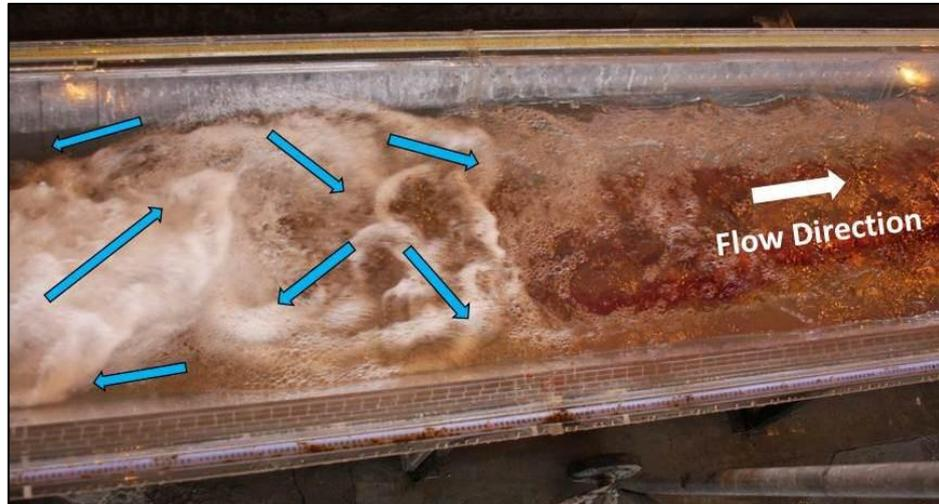
Figure 5-6: Flow Directions at Surface ( $F_1 = 6.87$ )
