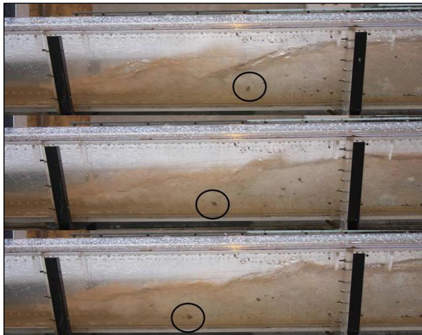
Figure 5-5: Side Flow Towards to Upstream ( $F_1 = 5.34$ )
