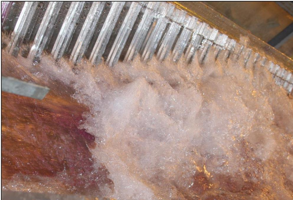
Figure 5-37: The Effect of Side Roughness on Hydraulic Jump
