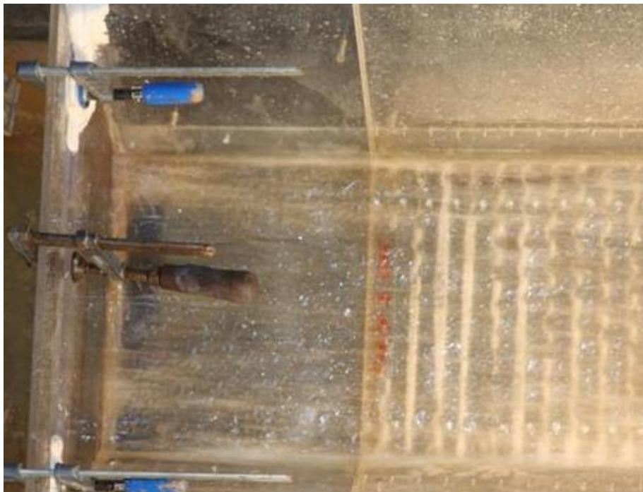
Figure 4-8: Dough at Sides to Improve Inlet Conditions
