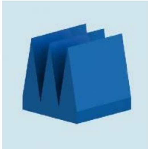
Figure 2.3 Geometry of wedge-shaped absorber material [24].
