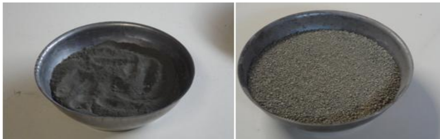
Figure 3.3 Air-dry tailing and sandy part of rock fill (Soil) ( D_{\max} < 2 mm) from storage part of Kastamonu Küre copper tailing dam.
