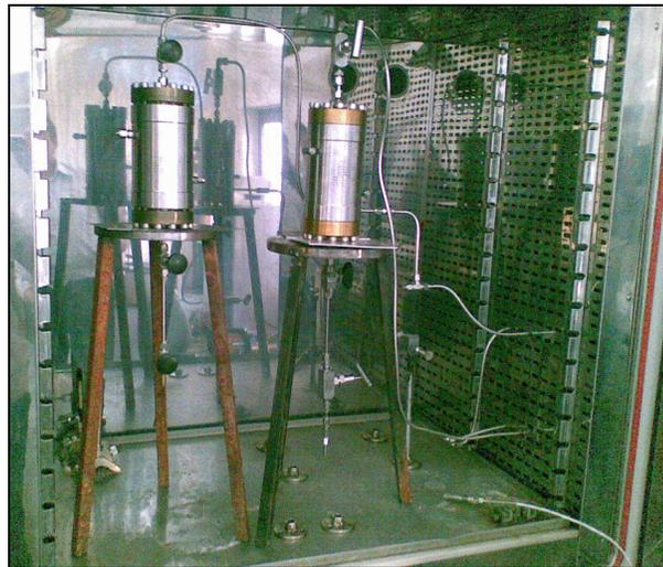
Figure 5. 6. Core Holders Used for the Experiments
