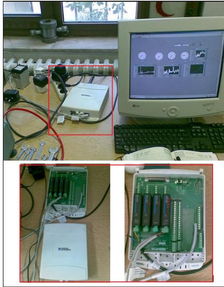
Figure 5.8. Data Logging System with Different Modules of Temperature and Pressure Measurements
