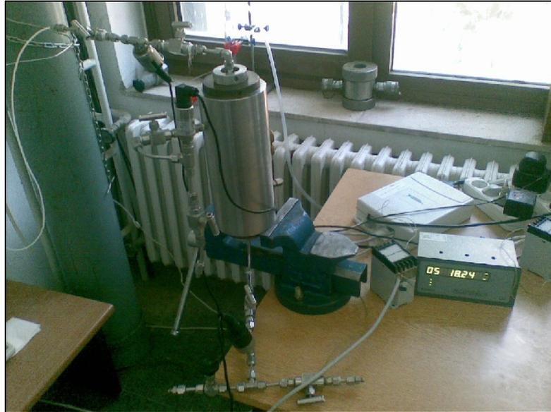
Figure 5. 4. Core Holder with its Pressure Transducers Used for Saturating the Core with n-decane
