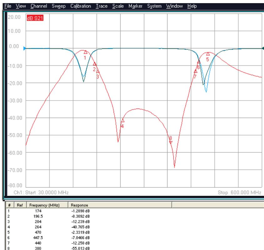
Figure 4.42: Response of Dual Band Filter When Tune Voltage is 4 V
