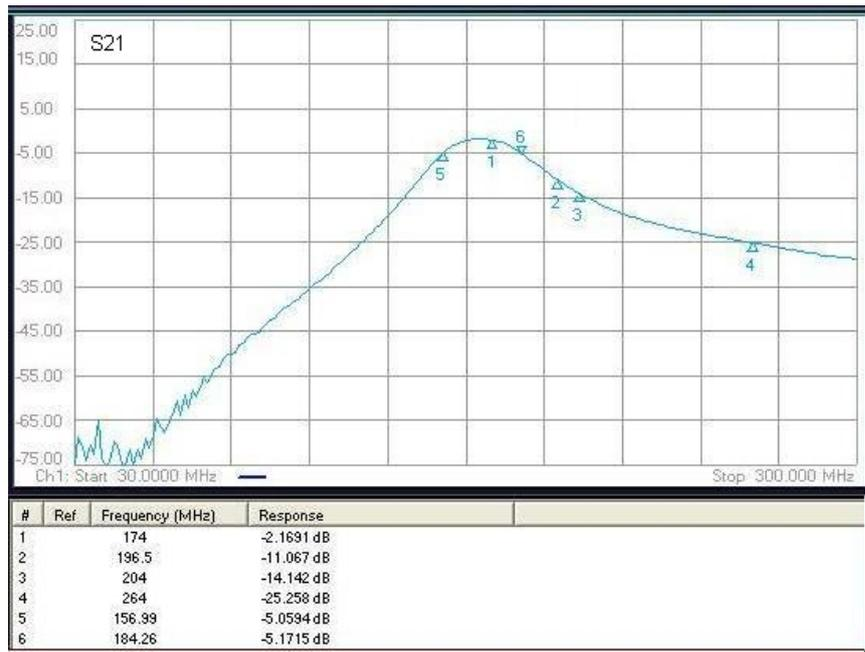
Figure 4.4: Response of Tunable Image Reject Filter at 174 MHz
