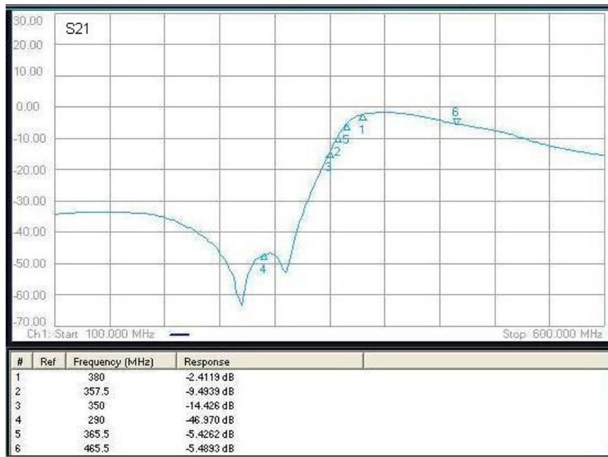
Figure 4.5: Response of UHF Pre-select Filter at 380 MHz
