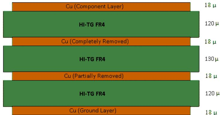
Figure 4.37: Layers of Designed PCB
