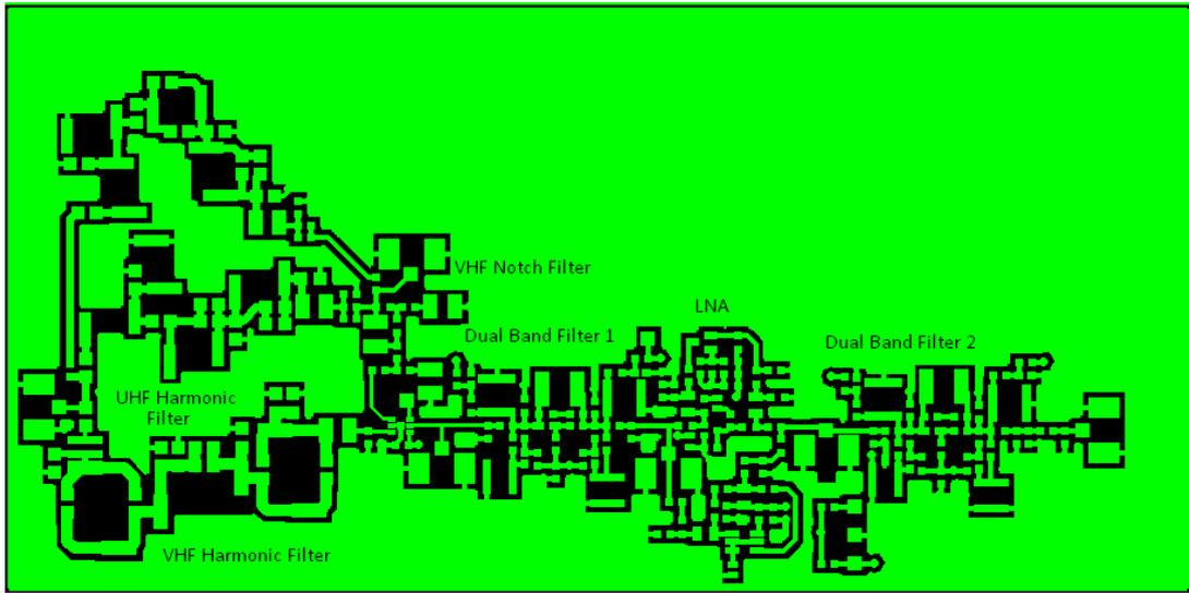
Figure 4.38: Component Layer of Designed PCB
