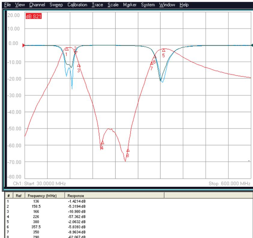
Figure 4.41: Response of Dual Band Filter When Tune Voltage is 1 V
