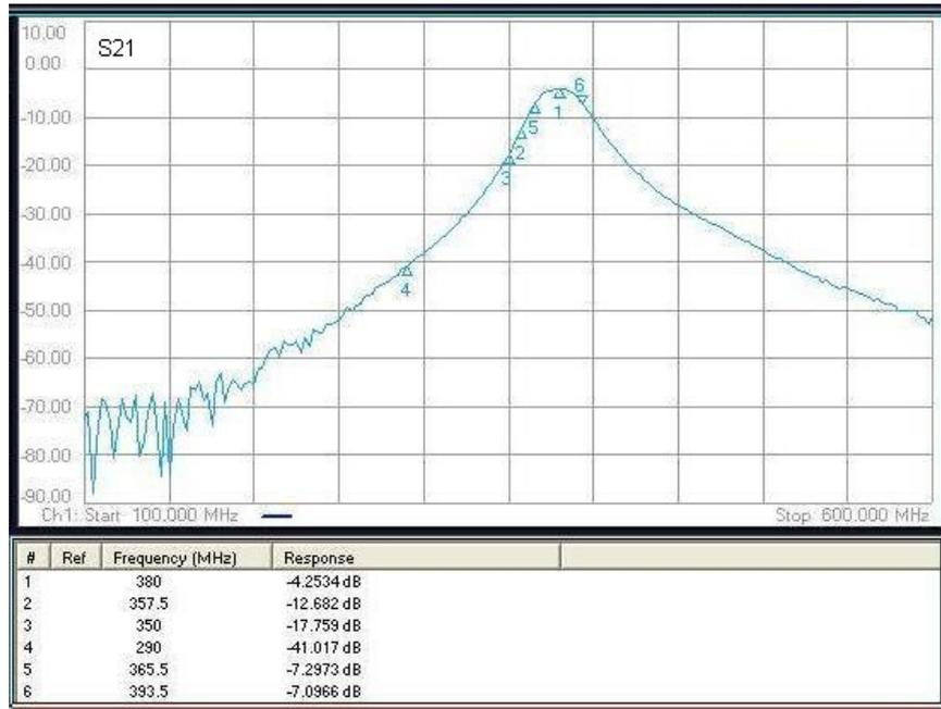
Figure 4.6: Response of UHF Image Reject Filter at 380 MHz
