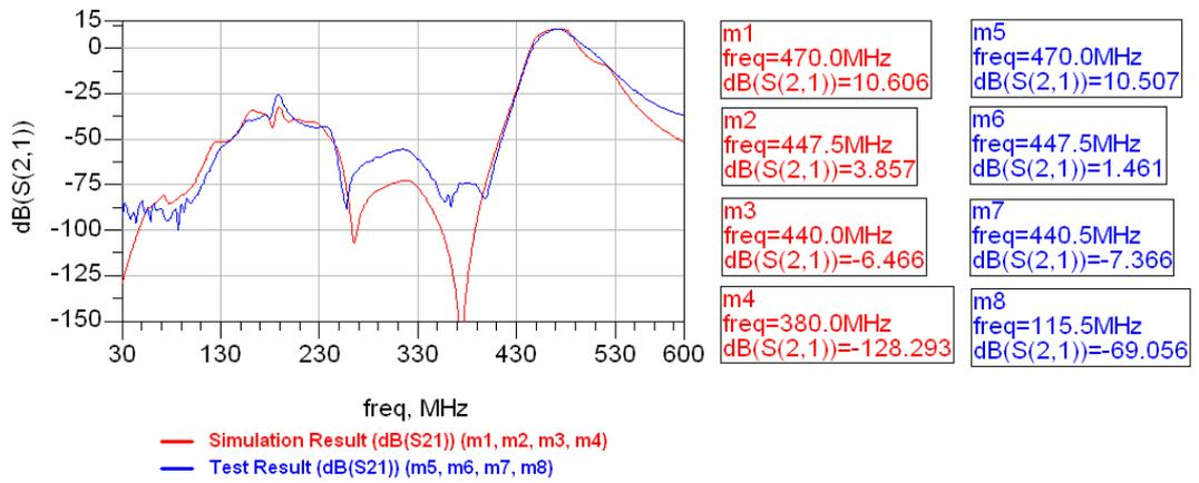
Figure 4.63: Comparison of Simulation and Test Results of Front-ends at 470 MHz
