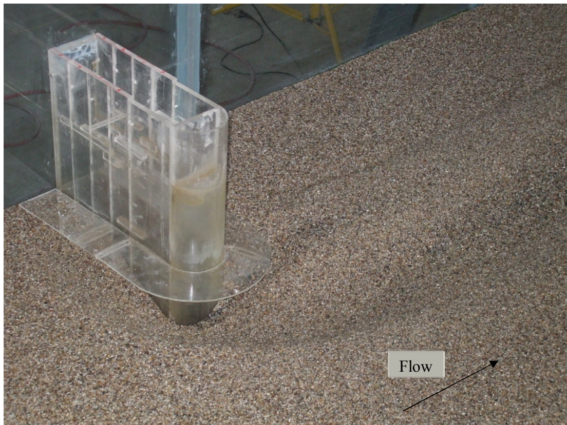
Figure 3.4 Abutment L_a=35 cm with collar B_c=7.5 cm at Z_c/y=0.00 , y=15.2 cm
