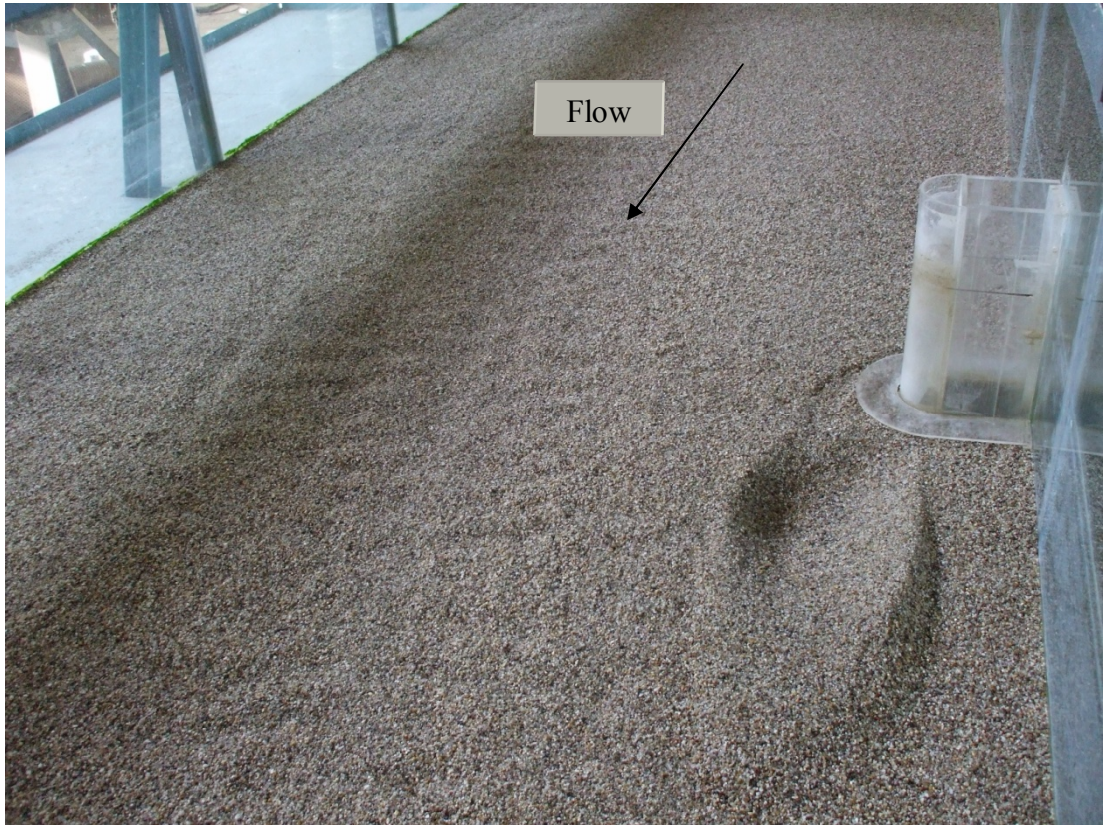
Figure 3.9 Abutment L_a=15 cm with collar B_c=5.0 cm at Z_c/y=0.00 , y=15.2 cm
