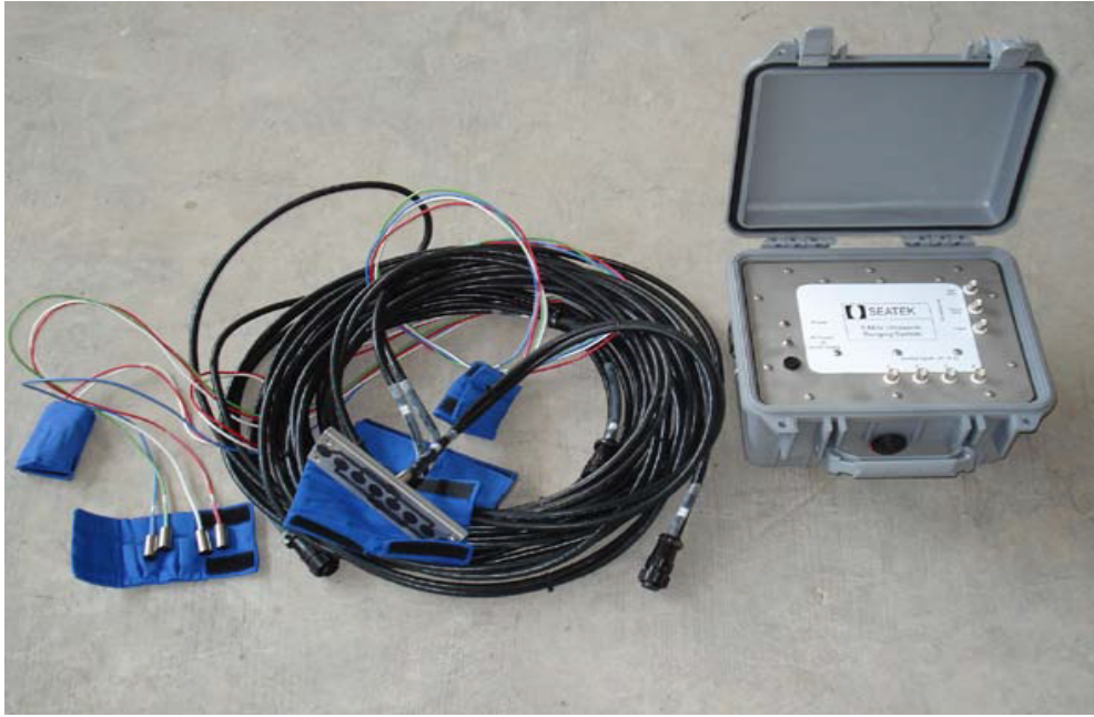
Figure 3.10 Seatek Ultrasonic Ranging System
