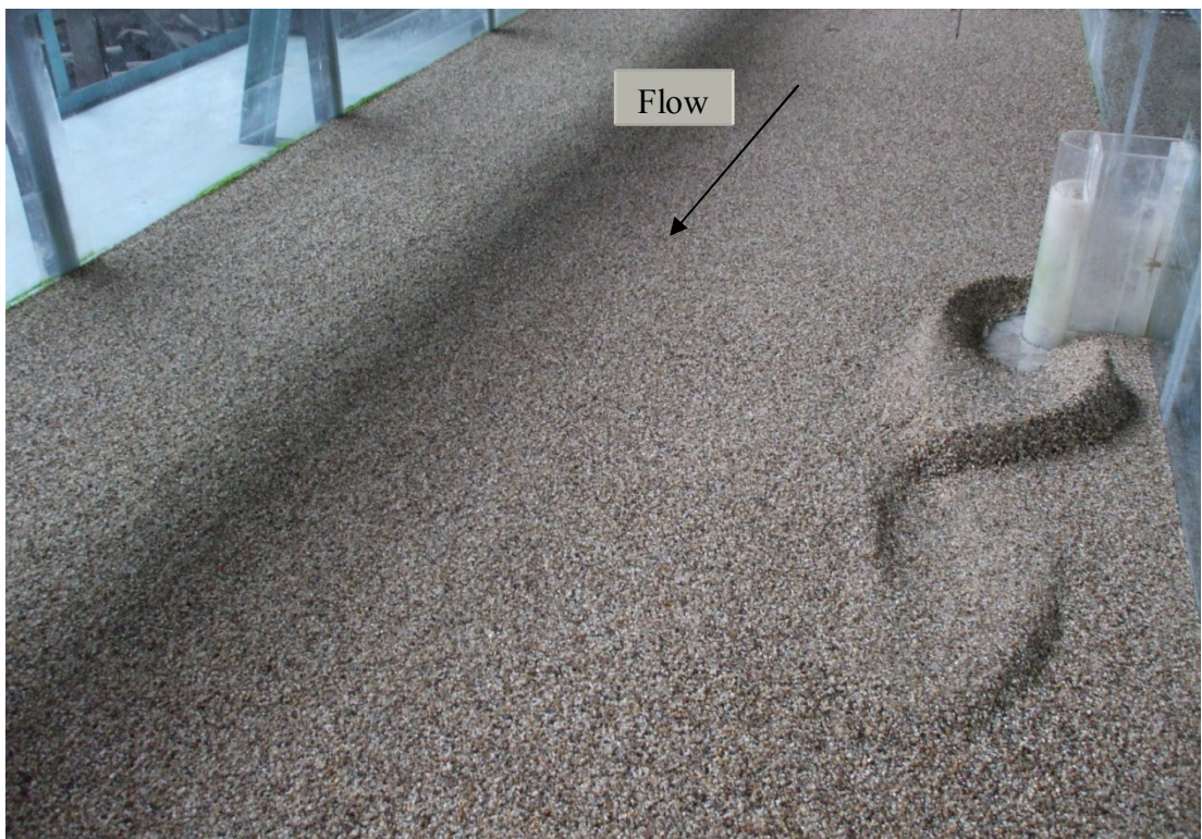
Figure 3.8 Abutment L_a=15 cm with collar B_c=7.5 cm at Z_c/y=-0.25 , y=15.2 cm
