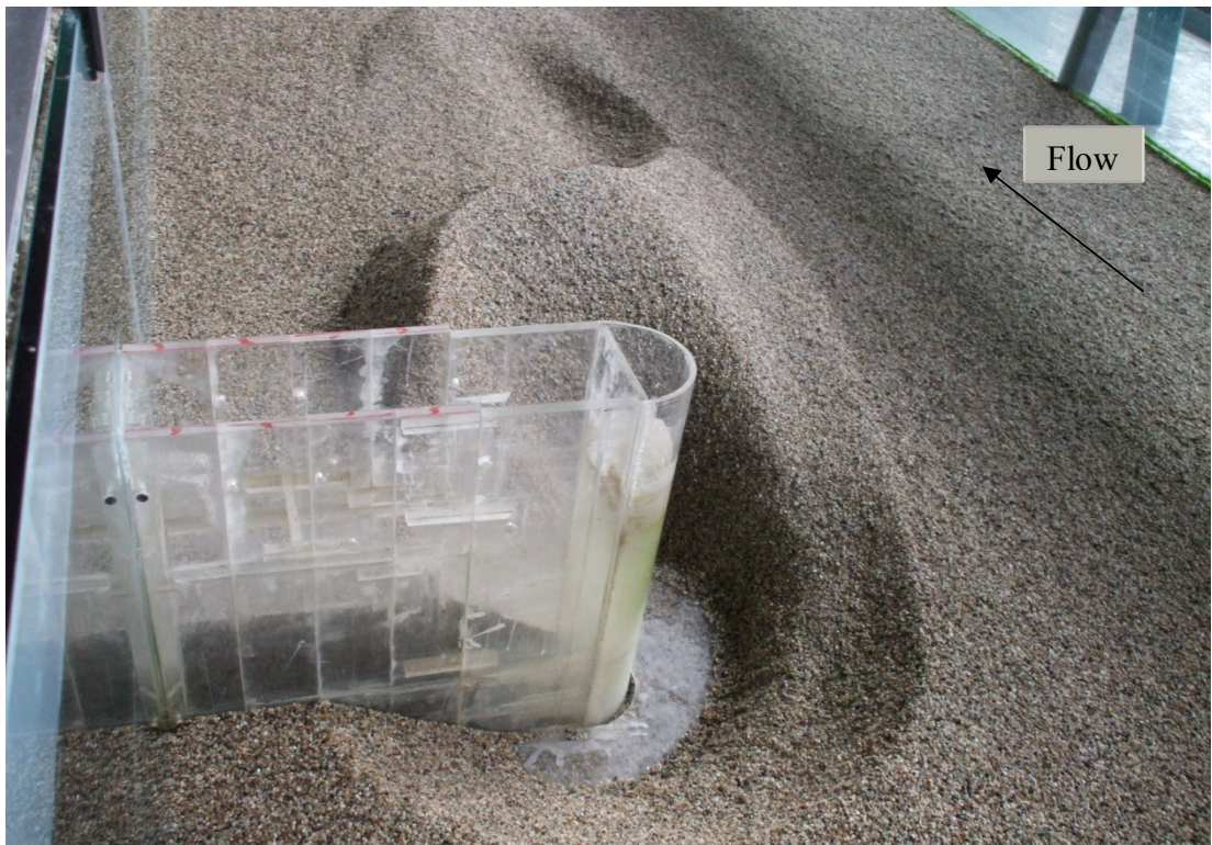
Figure 3.6 Abutment L_a=35 cm with collar B_c=10.0 cm at Z_c/y=-0.50 , y=17.4 cm
