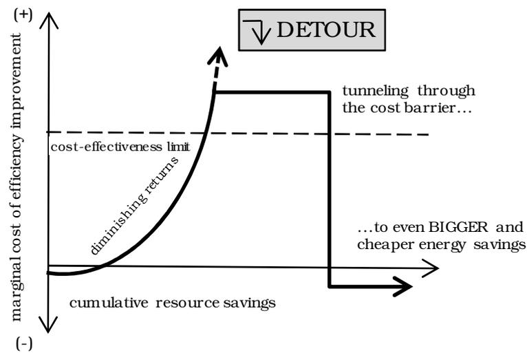
**Figure 2.6.** Tunnel through the cost barrier
