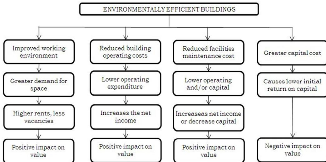
**Figure 2.4.** Value impact of environmentally efficient buildings (Source: Boyd and Kimmet, 2005)
