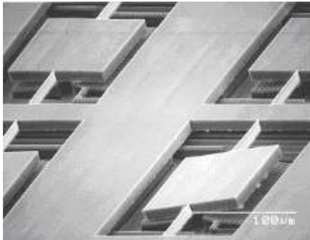
Figure 2-7: Titanium Mirrors Bulk Micromachined Using Deep Etching of a Titanium Substrate<sup>2</sup>
