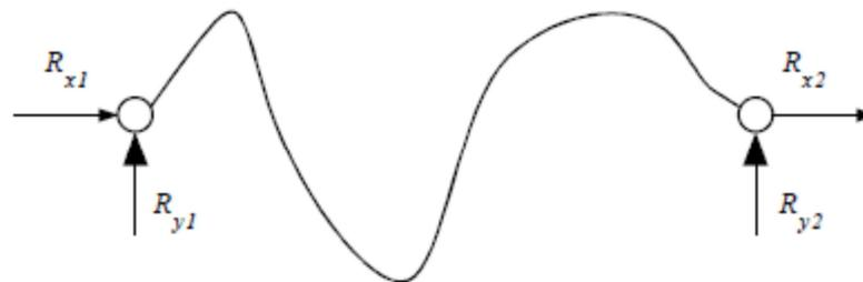
Figure 3-1: A Functionally Binary Pinned-Pinned (FBPP) Segment [27]
