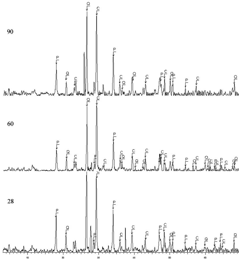
Figure 3.28 XRD traces of the mortar cubes RM-MC-Z (external surface) after 28, 60 and 90 days of curing time. C: Calcite, Q: Quartz, P: Portlandite
