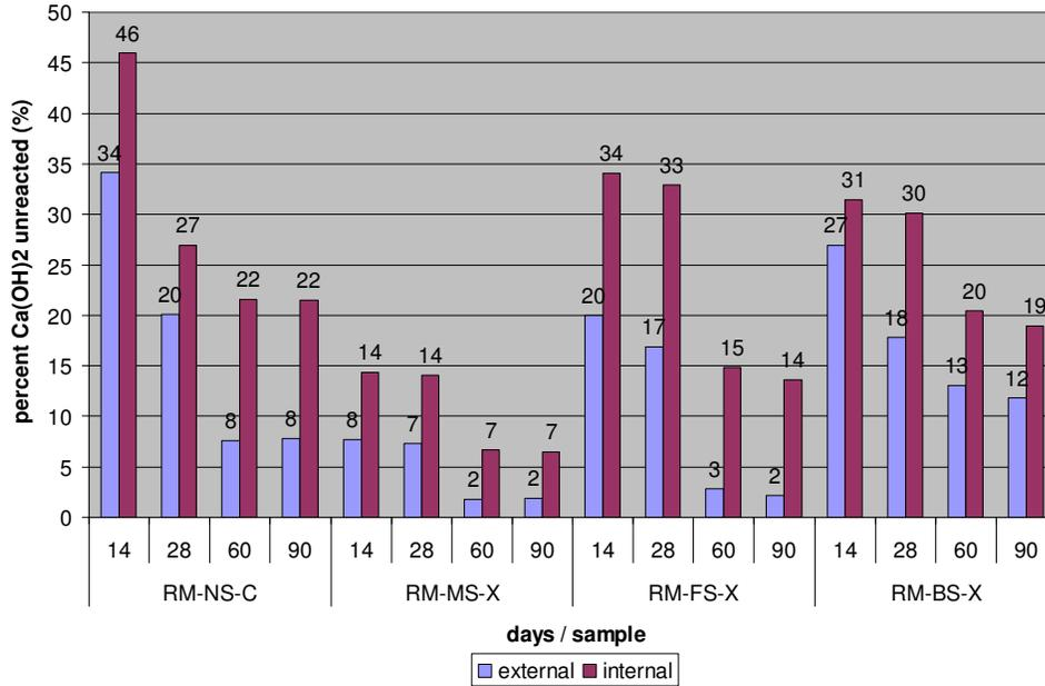
Figure 3.13 Free  $\text{Ca(OH)}_2$  content in the repair mortars after 14, 28, 60 and 90 days.
