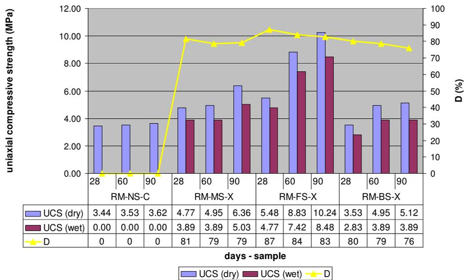
Figure 3.10 Uniaxial compressive strength of repair mortars (dry and water saturated), D:  $UCS_{wet}/UCS_{dry}$  ratio.
