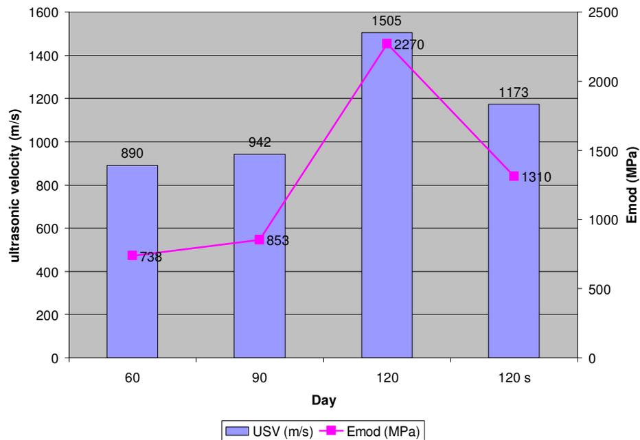
Figure 3.8 Ultrasonic velocity and modulus of elasticity values of prepared pozzolanic lime mortars RM-MC-Y from day 60 to day 120. 120 s denotes to mortars left outdoors on site.
