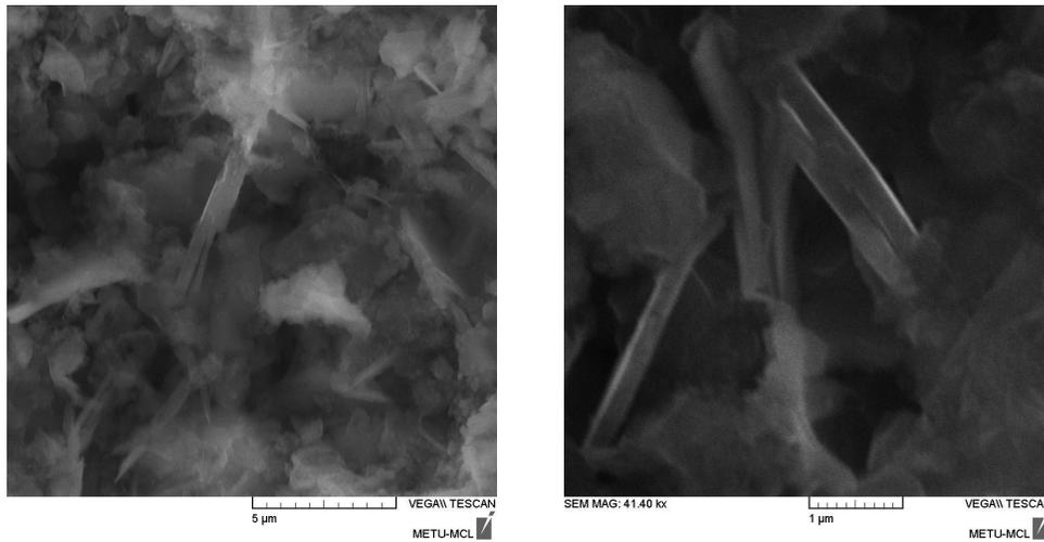
Fig 3.19 SEM image of needle like CASH formation from mortar prepared with added metakaolin (left).
