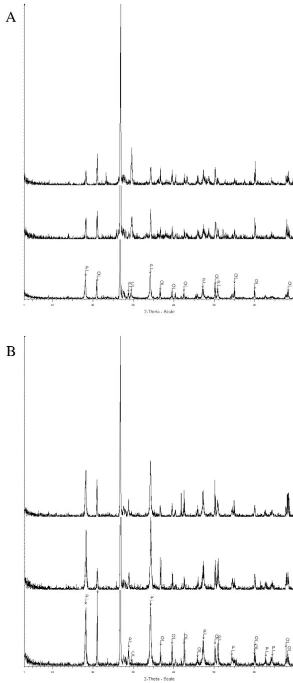
Figure 3.22 XRD traces of the mortar set, RM-NS-C after 28, 30 and 90 days (from bottom to top) of curing time (A external surface, B internal surface). C: Calcite, Q: Quartz, P: Portlandite
