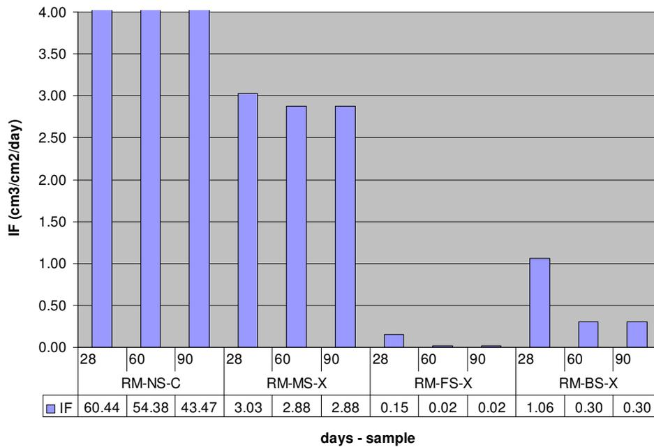
Figure 3.5 Impermeability coefficient of repair mortars, RM-MS-X, RM-FS-X, RM-BS-X and control, RM-NS-C.
