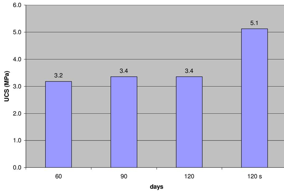
Figure 3.11 Uniaxial compressive strength of prepared pozzolanic lime mortars, RM-MC-Y from day 60 to day 120. 120 s denotes to mortars left outdoors on site.
