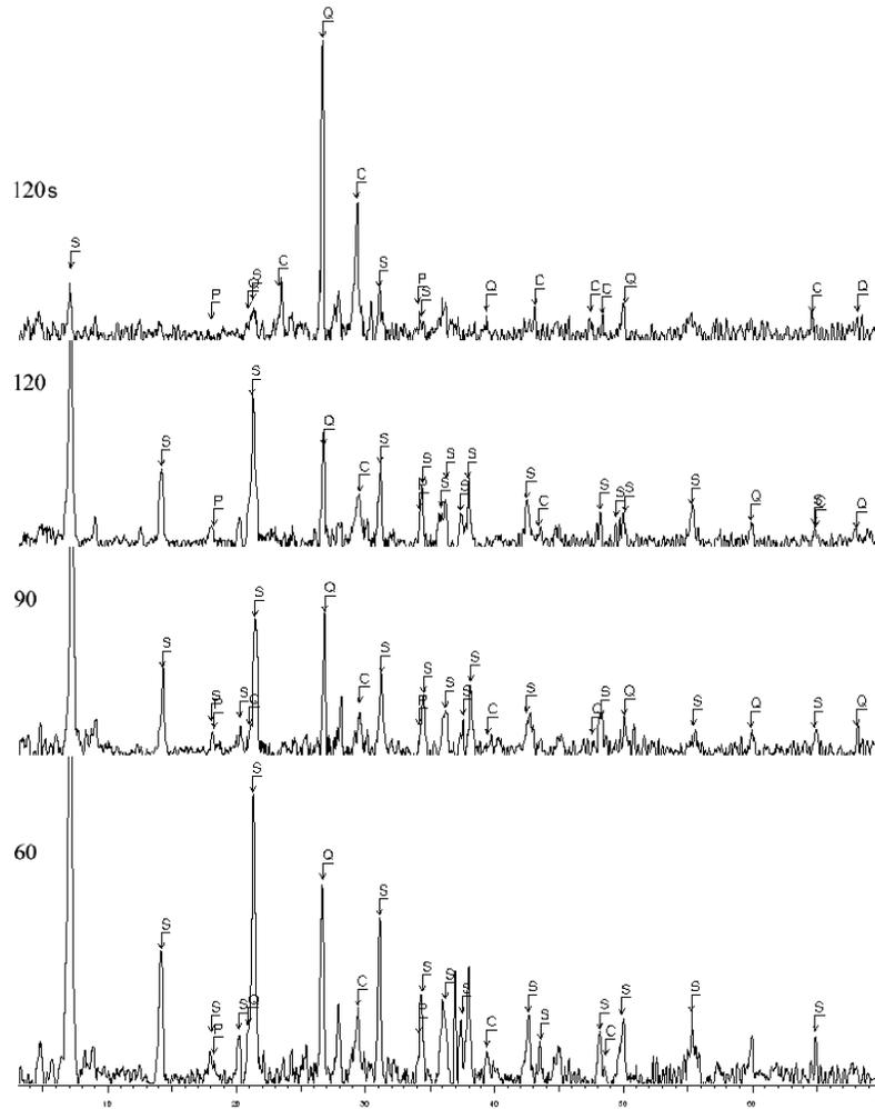
Figure 3.27 XRD traces of mortar cubes RM-MC-Y (internal surface) after 60, 90 and 120 days (from bottom to top) of curing time. 120 s denotes the XRD trace of mortar cube left on site for 120 days. C: Calcite, Q: Quartz, P: Portlandite, S: Stratlingite
