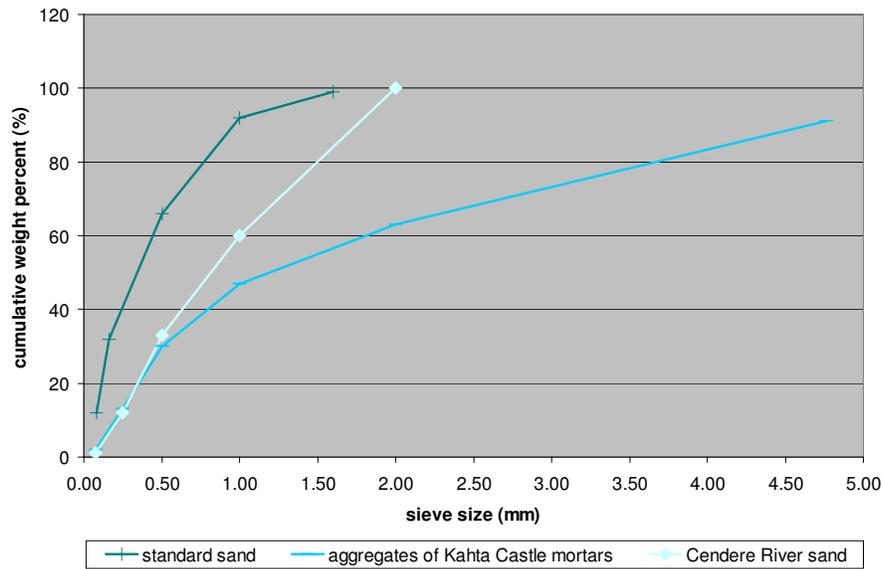
Figure 3.14 Particle size distributions of the acid insoluble parts of Kahta Castle mortars, standard sand and Cendere River sand used in the preparation of repair mortars
