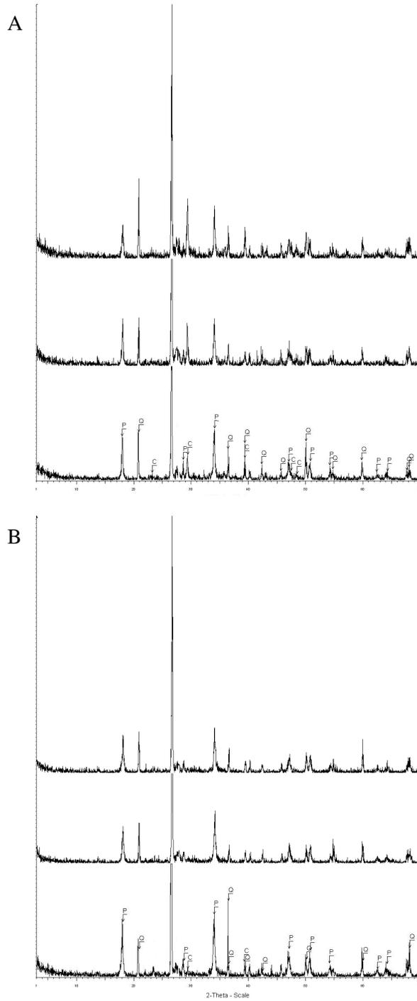
Figure 3.25 XRD traces of the mortar set RM-BS-X after 28, 30 and 90 days (from bottom to top) of curing time (A external surface, B internal surface). C: Calcite, Q: Quartz, P: Portlandite
