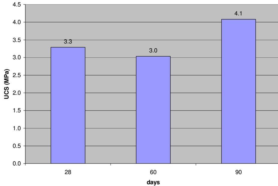
Figure 3.12 Uniaxial compressive strength of prepared pozzolanic lime mortars, RM-MC-Z from day 28 to day 90.
