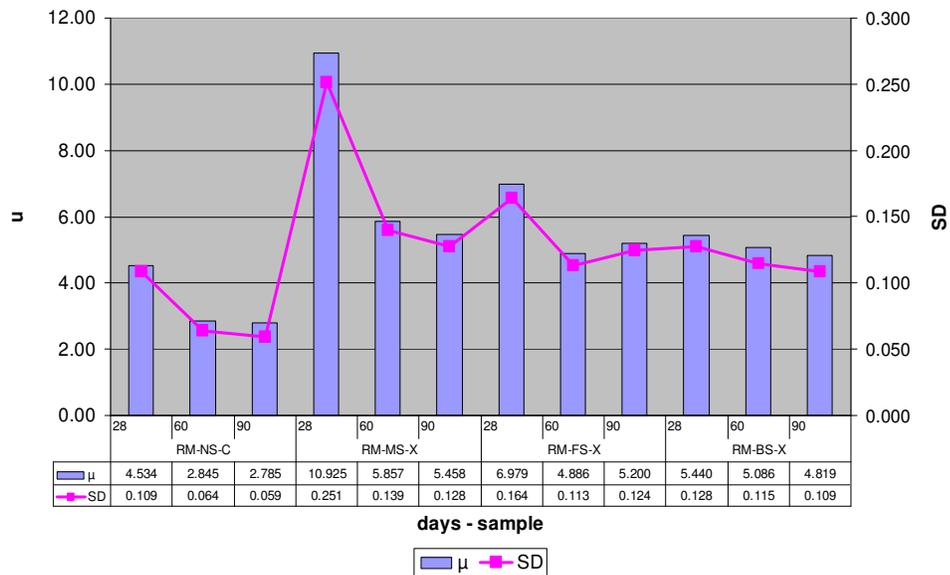
Figure 3.4 SD and  $\mu$  values of prepared repair mortars, RM-MS-X, RM-FS-X, RM-BS-X and control, RM-NS-C.
