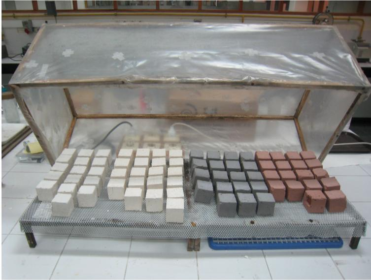
Figure 2.2 Some of the prepared pozzolanic lime mortars and the chamber.
