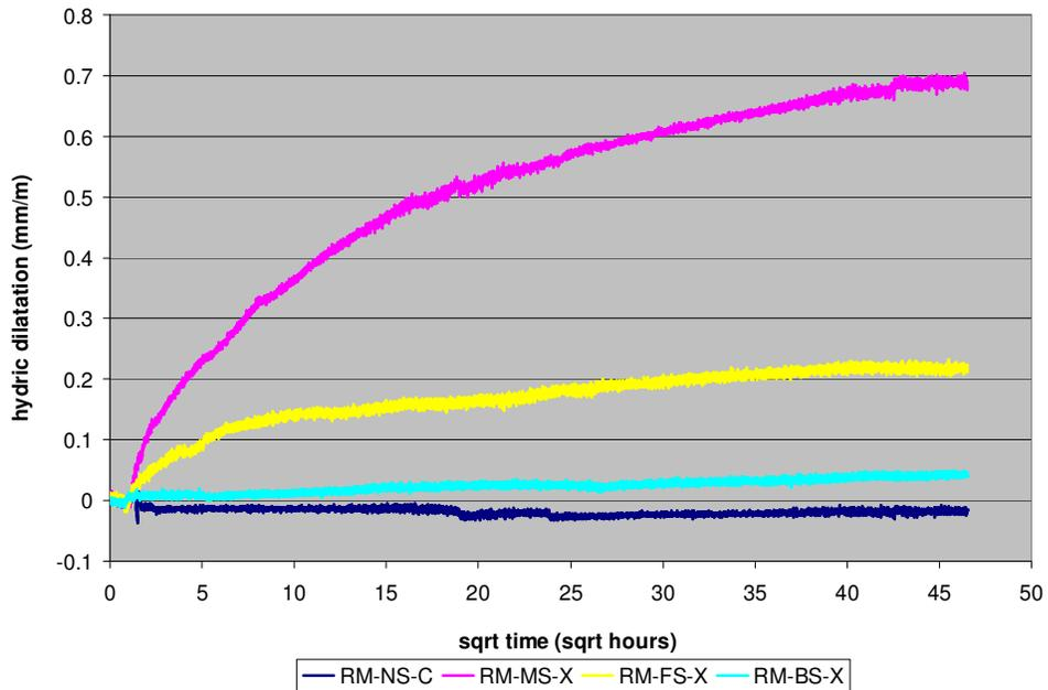
Figure 3.6 Hydric dilatation of repair mortars (RM-MS-X, RM-FS-X, RM-BS-X and control (RM-NS-C)).
