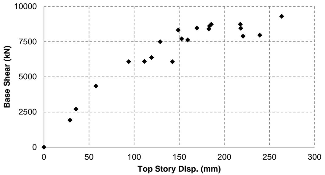
Figure 4.17 Base Shear vs Top Story Disp. Relationship
