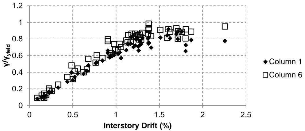
**Figure 4.19 Normalized Shear Strain vs Interstory Disp. for exterior columns**
