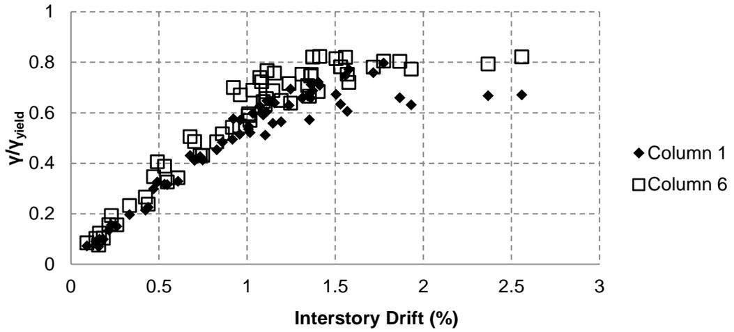
Figure 4.28 Normalized Shear Strain vs. Interstory Disp. for exterior columns
