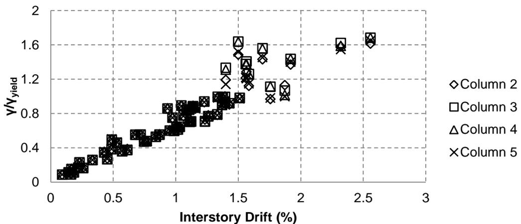
**Figure 4.26 Normalized Shear Strain vs. Interstory Disp. for interior columns**
