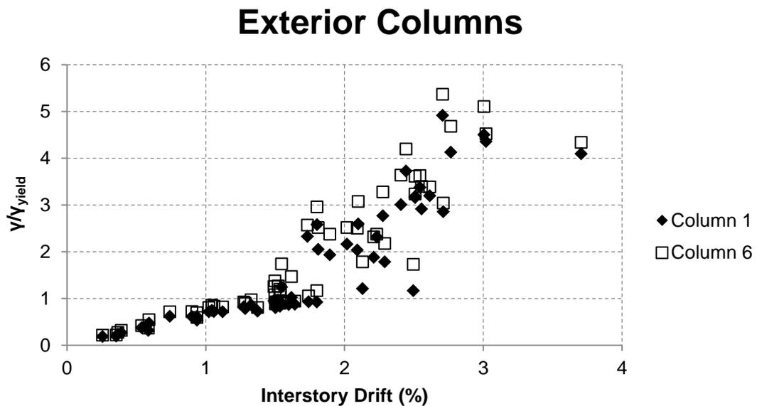
Figure 4.3 Analysis results of exterior columns with unreinforced panel zones
