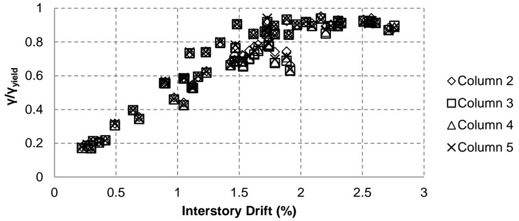
Figure 4.16 Normalized Shear Strain vs Interstory Disp. for interior columns
