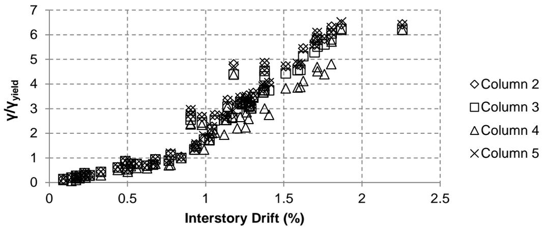
**Figure 4.20 Normalized Shear Strain vs Interstory Disp. for interior columns**
