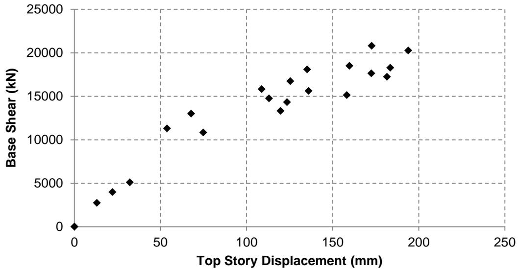
**Figure 4.21 Base Shear vs Top Story Disp. Relationship**
