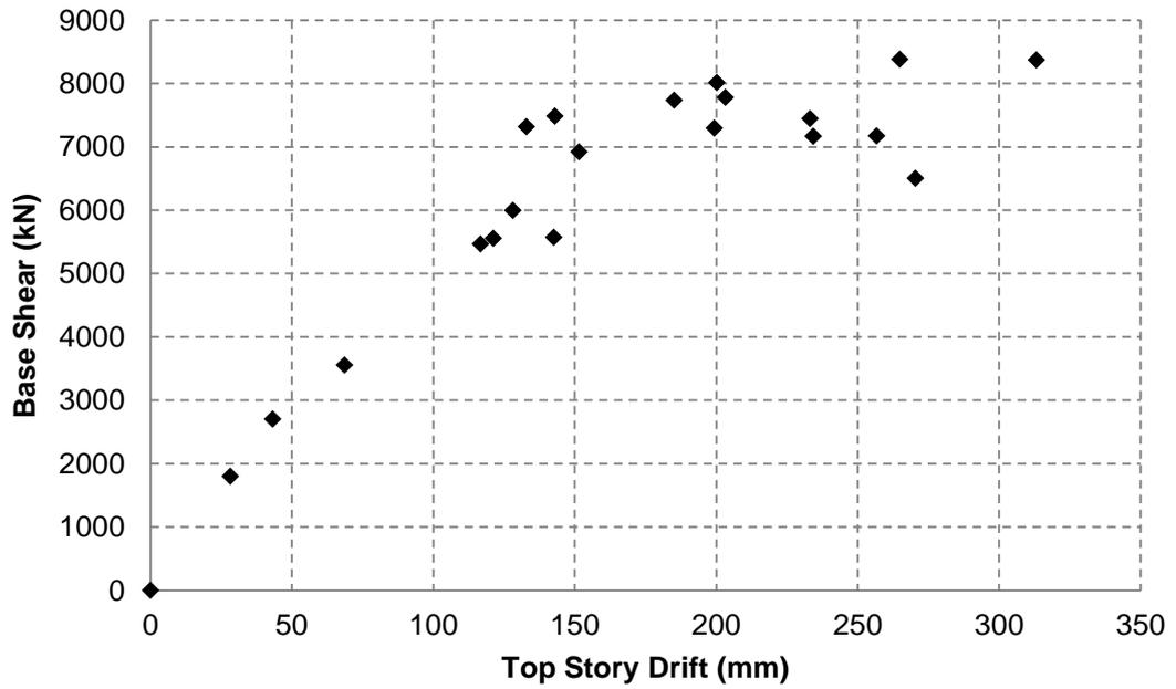
Figure 4.8 Base Shear vs Top Story Drift Relationship
