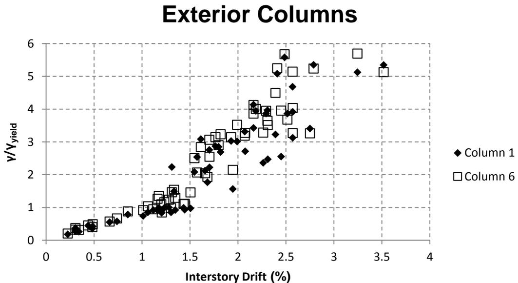
**Figure 4.6 Normalized Shear Strain vs Interstory Disp. for exterior columns**
