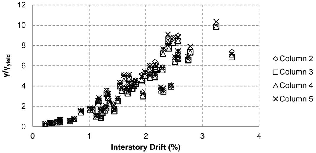
Figure 4.7 Normalized Shear Strain vs Interstory Disp. for interior columns
