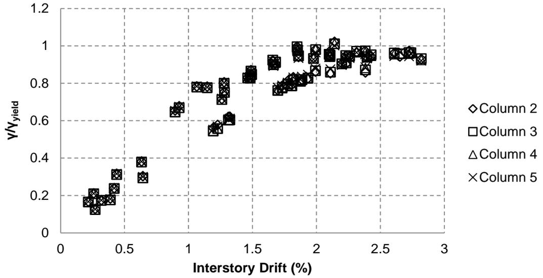
Figure 4.13 Normalized Shear Strain vs Interstory Disp. for interior columns
