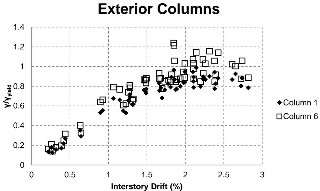
Figure 4.12 Normalized Shear Strain vs Interstory Disp. for exterior columns
