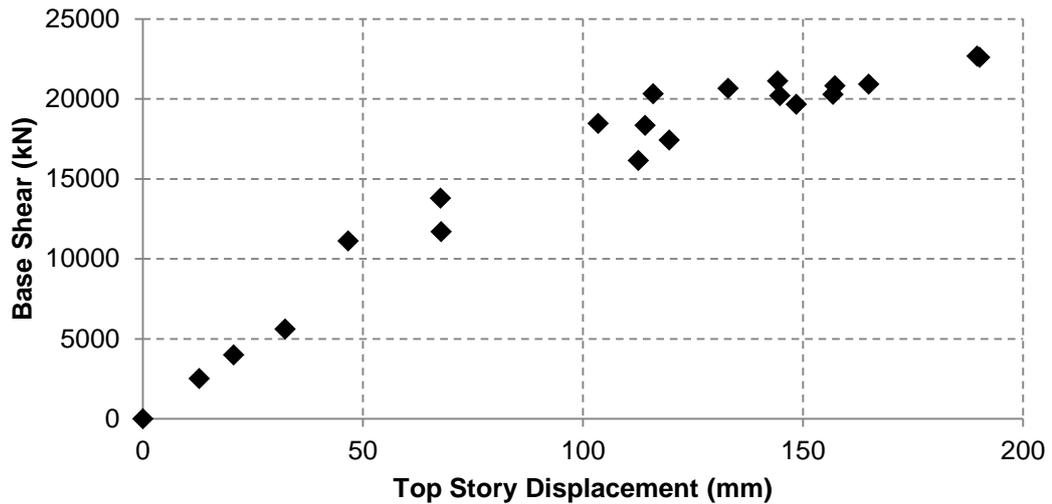
**Figure 4.30 Base Shear vs. Top Story Displacement relationship**
