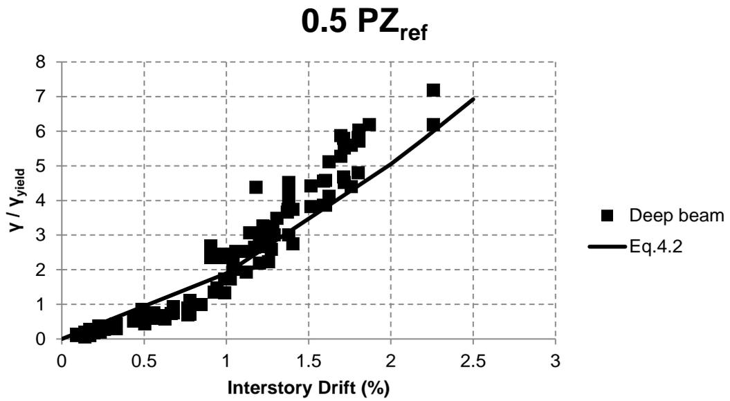
Figure 4.32 The 0.5  $PZ_{ref}$  Case Panel Zone Shear Deformation Demands Curve
