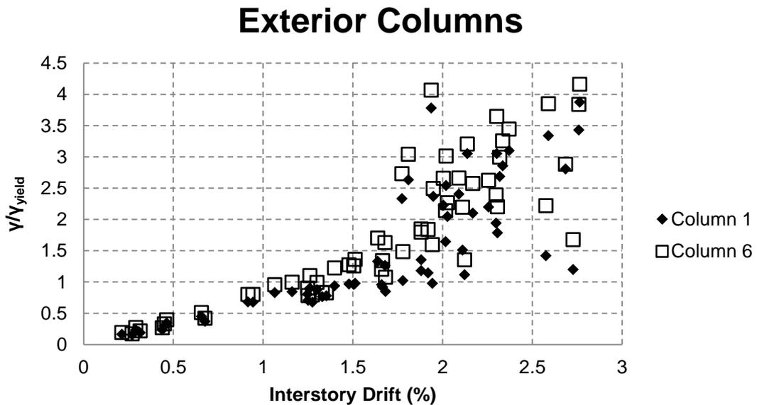
Figure 4.9 Normalized Shear Strain vs Interstory Disp. for exterior columns
