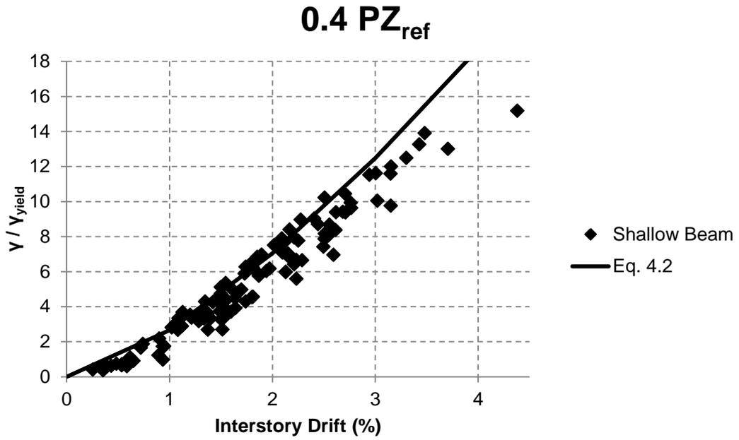
Figure 4.31 The 0.4 Case Panel Zone Shear Deformation Demands Curve
