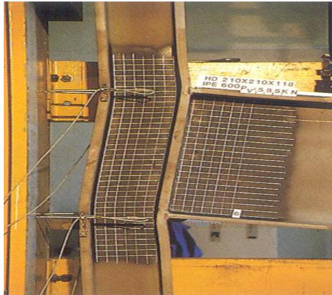
Figure 1.2 Excessive Joint Distortion (Adopted from AISC)
