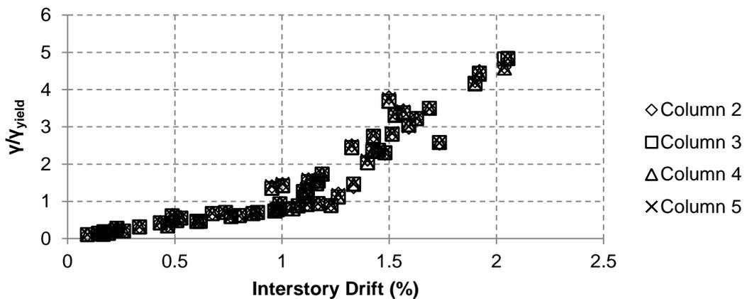
**Figure 4.23 Normalized Shear Strain vs Interstory Disp. for interior columns**
