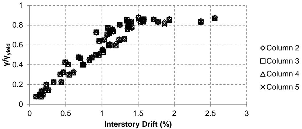
Figure 4.29 Normalized Shear Strain vs. Interstory Disp. for interior columns
