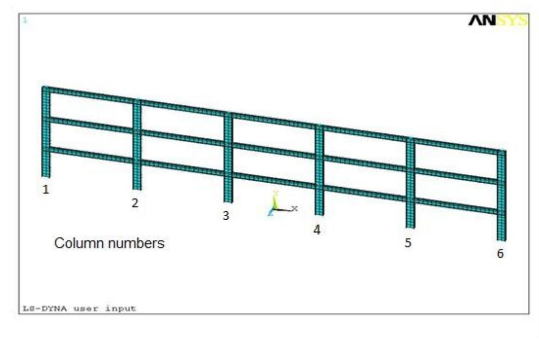
**Figure 4.1 A single bay steel moment frame model**
