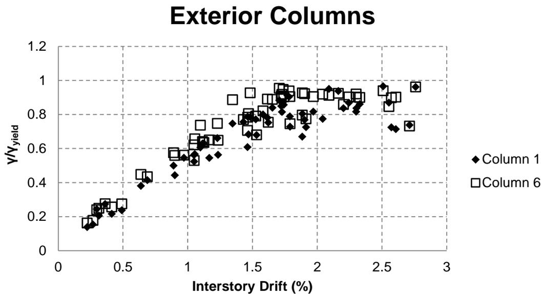
Figure 4.15 Normalized Shear Strain vs Interstory Disp. for exterior columns
