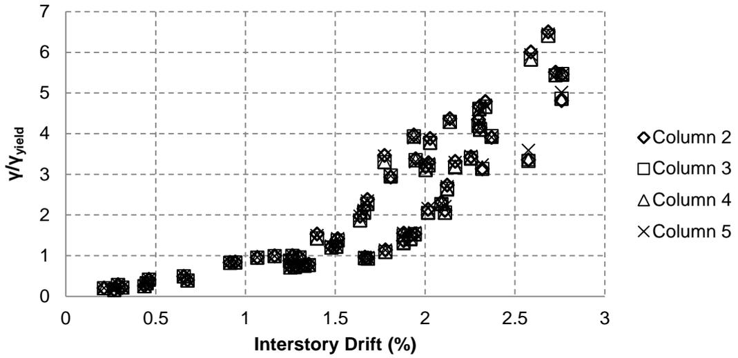
Figure 4.10 Normalized Shear Strain vs Interstory Disp. for interior columns
