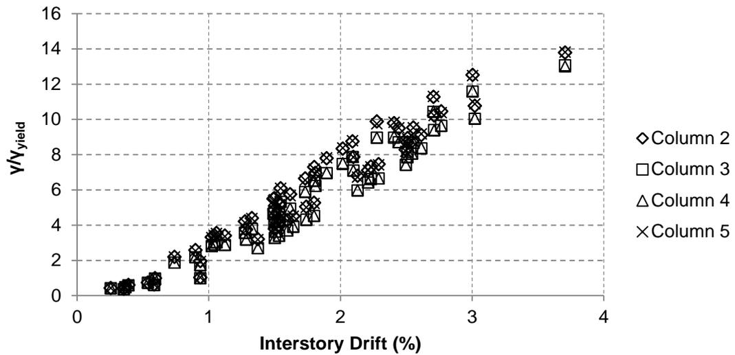
Figure 4.4 Normalized Shear Strain vs Interstory Disp. for interior columns
