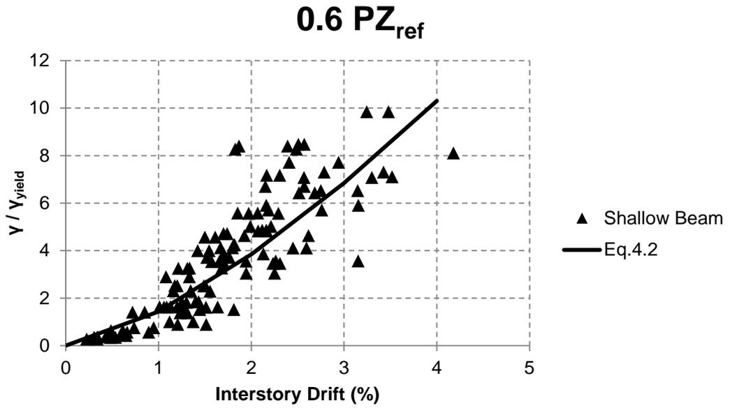
Figure 4.33 The 0.6  $PZ_{ref}$  Case Panel Zone Shear Deformation Demands Curve
