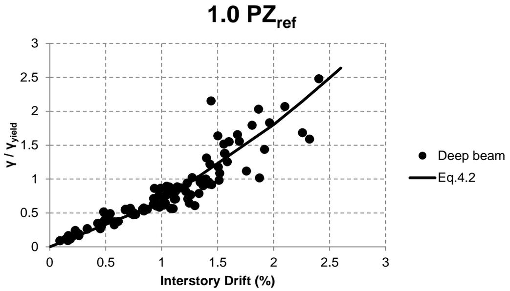
**Figure 4.35 The 1.0 PZ<sub>ref</sub> Case Panel Zone Shear Deformation Demands Curve**
