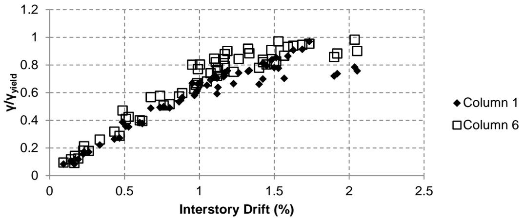
**Figure 4.22 Normalized Shear Strain vs Interstory Disp. for exterior columns**
