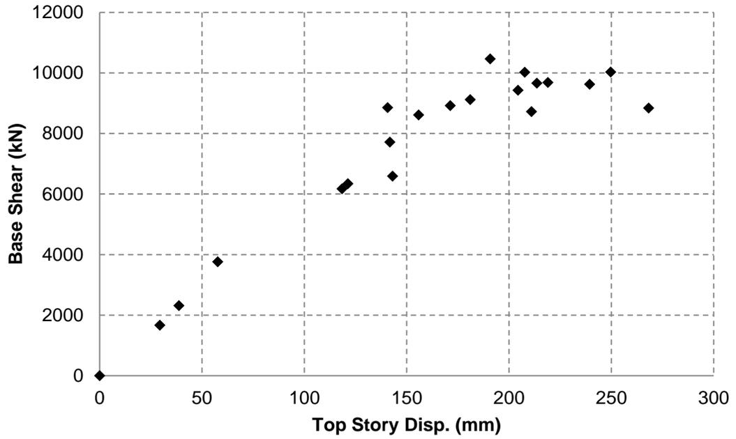
Figure 4.14 Base Shear vs Top Story Disp. Relationship
