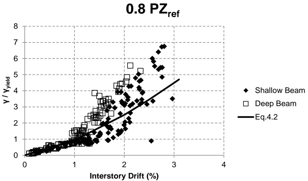
Figure 4.34 The 0.8  $PZ_{ref}$  Case Panel Zone Shear Deformation Demands Curve
