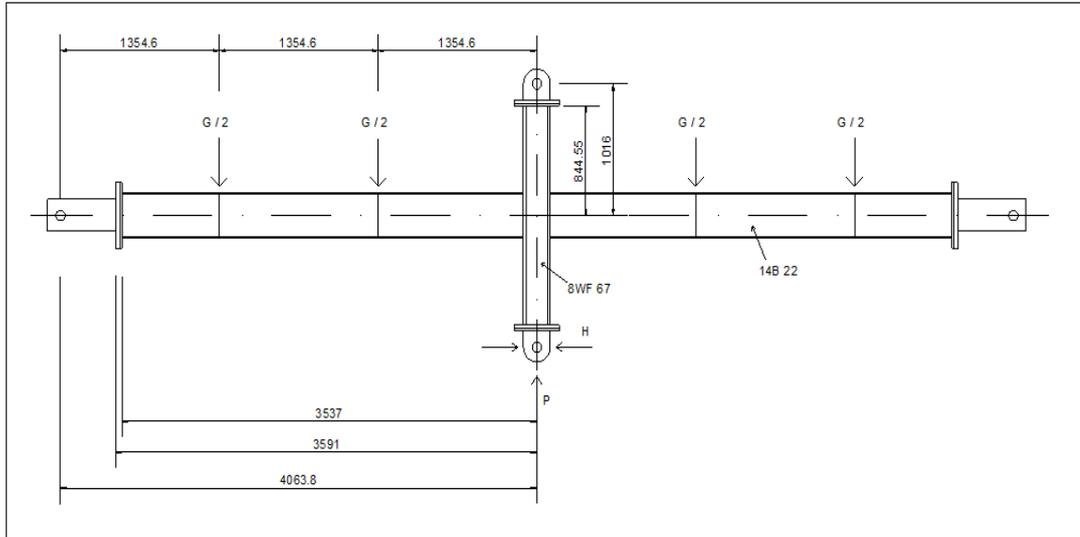
**Figure 3.1 The test set up (dimensions in mm)**
