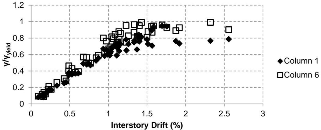
**Figure 4.25 Normalized Shear Strain vs. Interstory Disp. for exterior columns**
