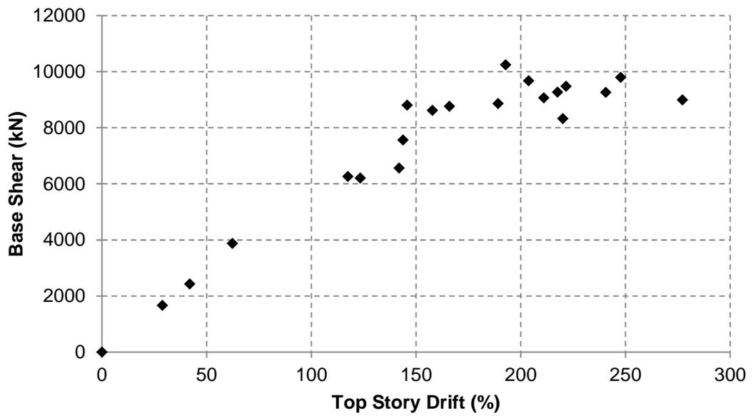
Figure 4.11 Base Shear vs Top Story Drift Relationship
