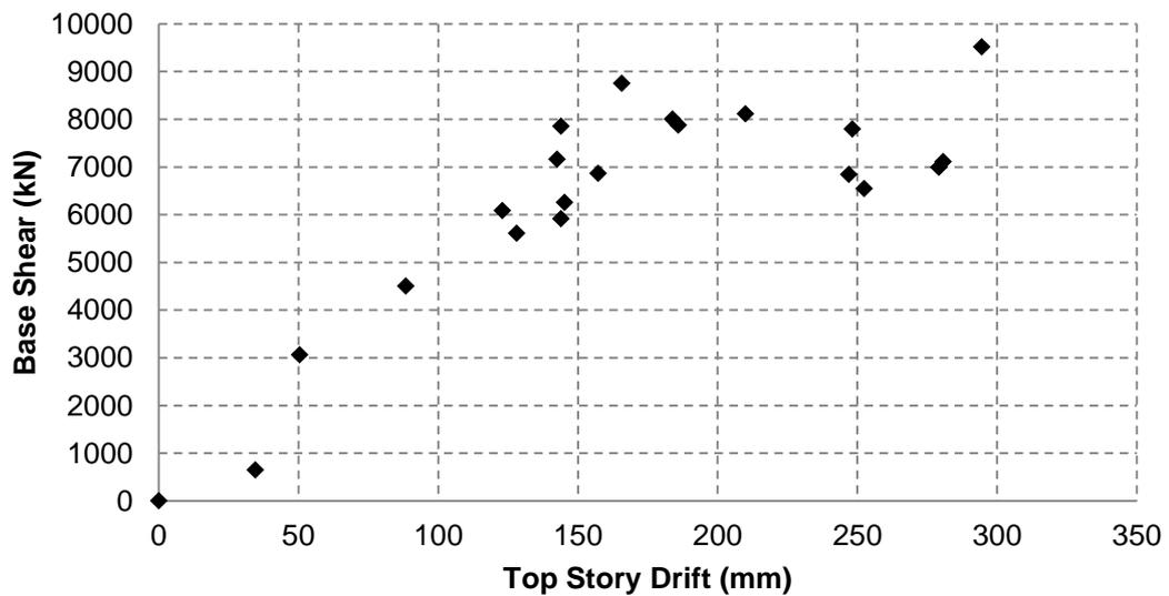
Figure 4.5 Base Shear vs Top Story Drift relationship
