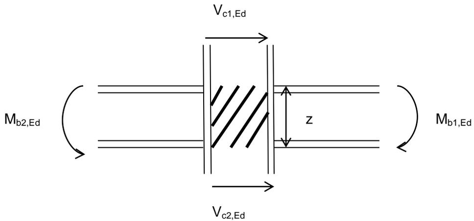
Figure 2.2 Shear forces and moments in web panel
