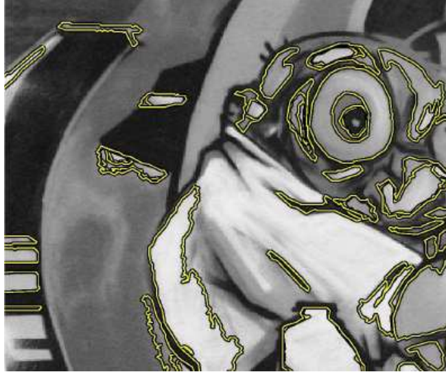
Figure 2.8: Maximally Stable Extremal Regions (MSER) Example Detections [71]
