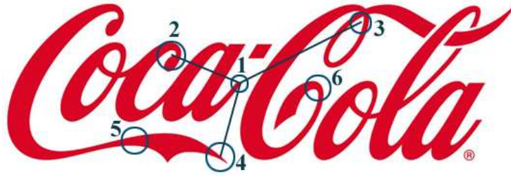
Figure 4.13: Example grouping according to Euclidean distance. Neighbors of interest point 1 are 2, 3, 4, 5 & 6. One of the triple combinations (2, 3, 4) is illustrated.
