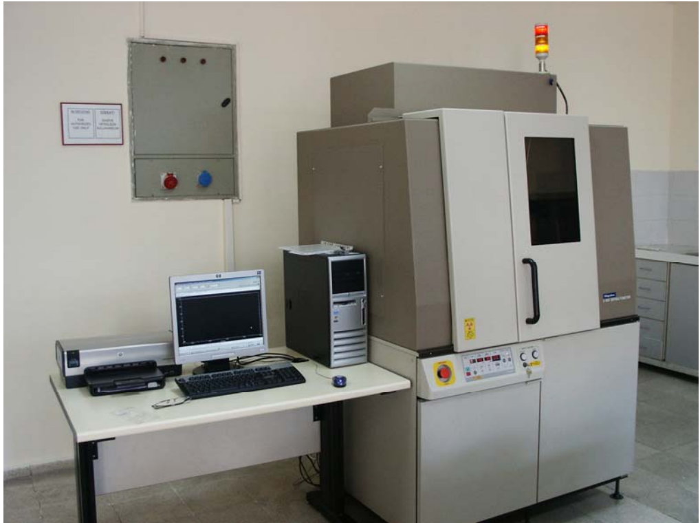
Figure 4.68 Rigaku brand X-Ray Diffractometer
