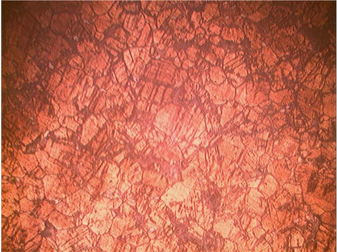
Figure 5.21 Worked again after annealed microstructure of sample Kt-49 (X300)
