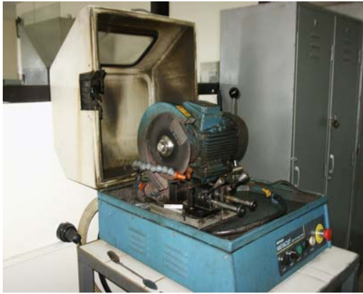
Figure 4.69 Abrasive cutoff machine
