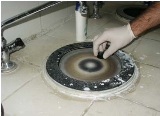
4.73 Fine polishing operation
