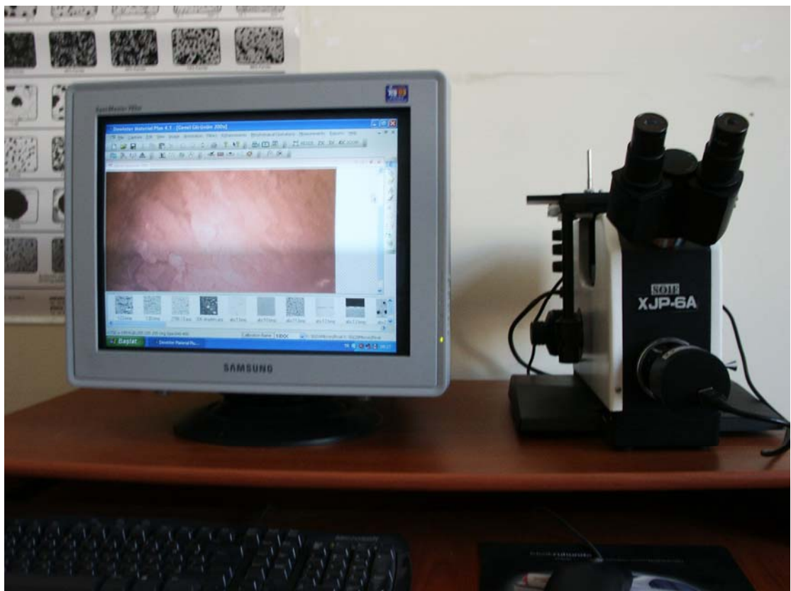
Figure 4.77 Metal Microscope and attached computer unit for image analyser
