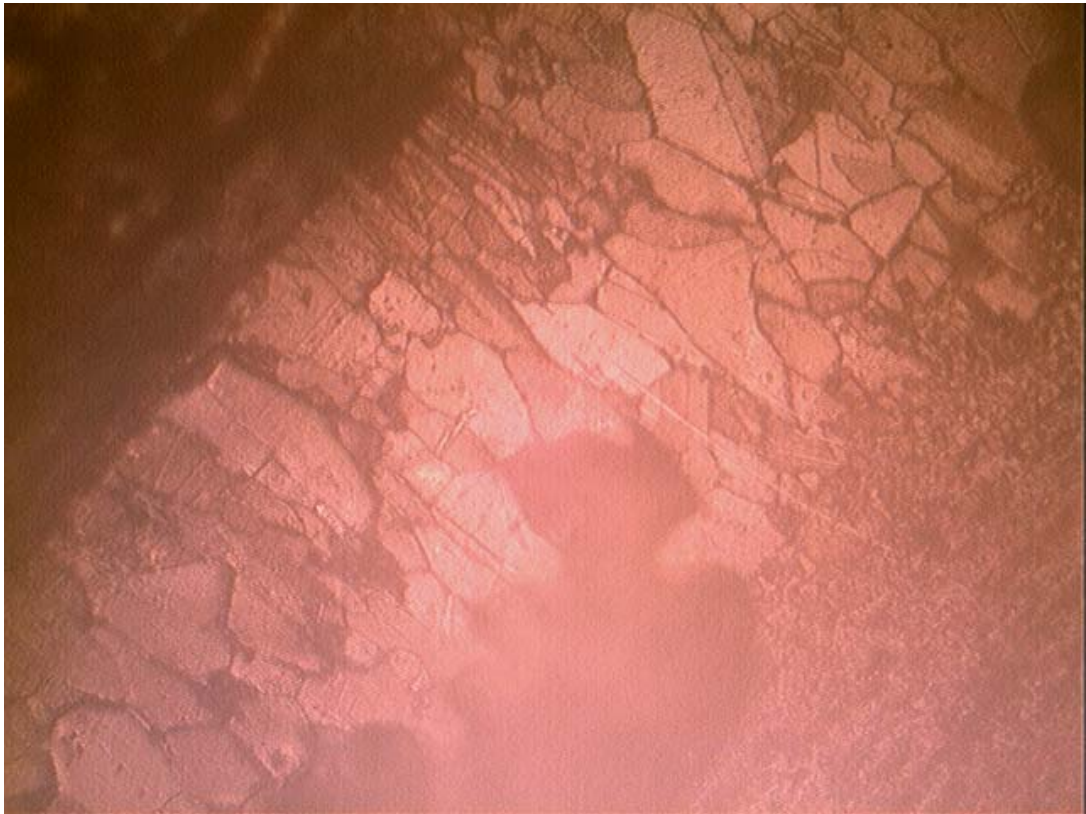
Figure 5.16 Elongated grains revealing the effects of hammering in Kt-39 (X200)
