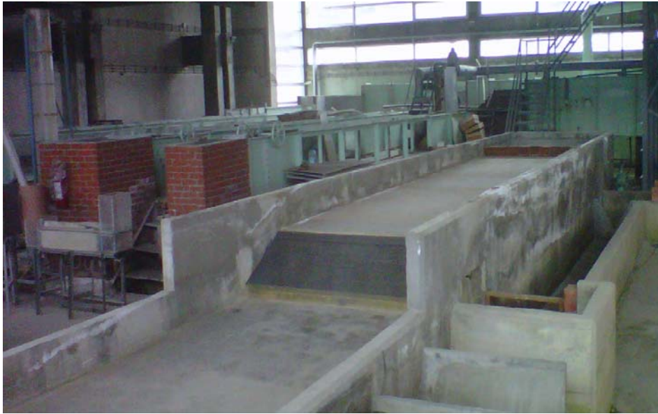
Figure 3.2 General view of the Tyrolean weir model
