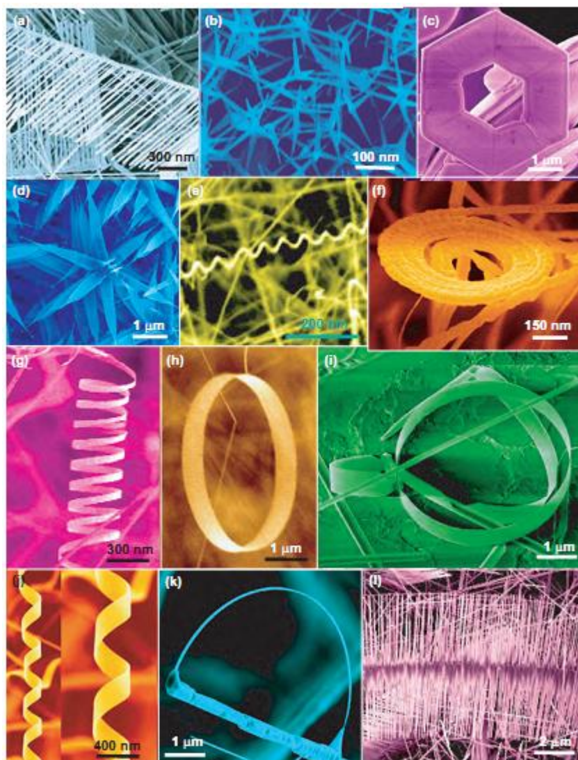
Figure 2.3. ZnO nanostructures in different morphologies types using VLS methods [49].
