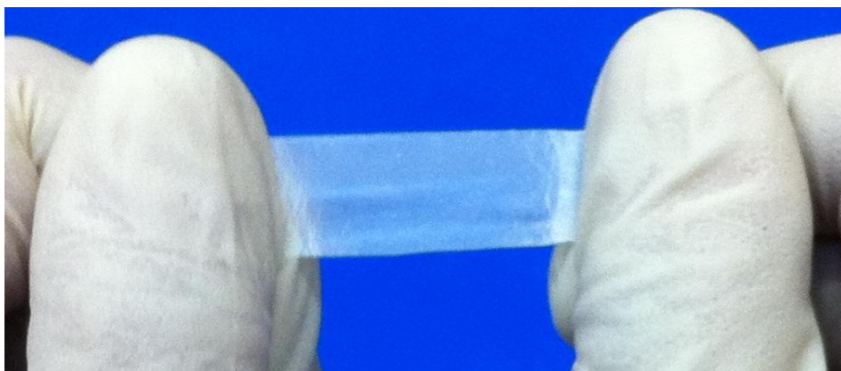
Figure 3.5 Bone regeneration membranes (PCL-30 \beta /G sample was used in this photograph).
