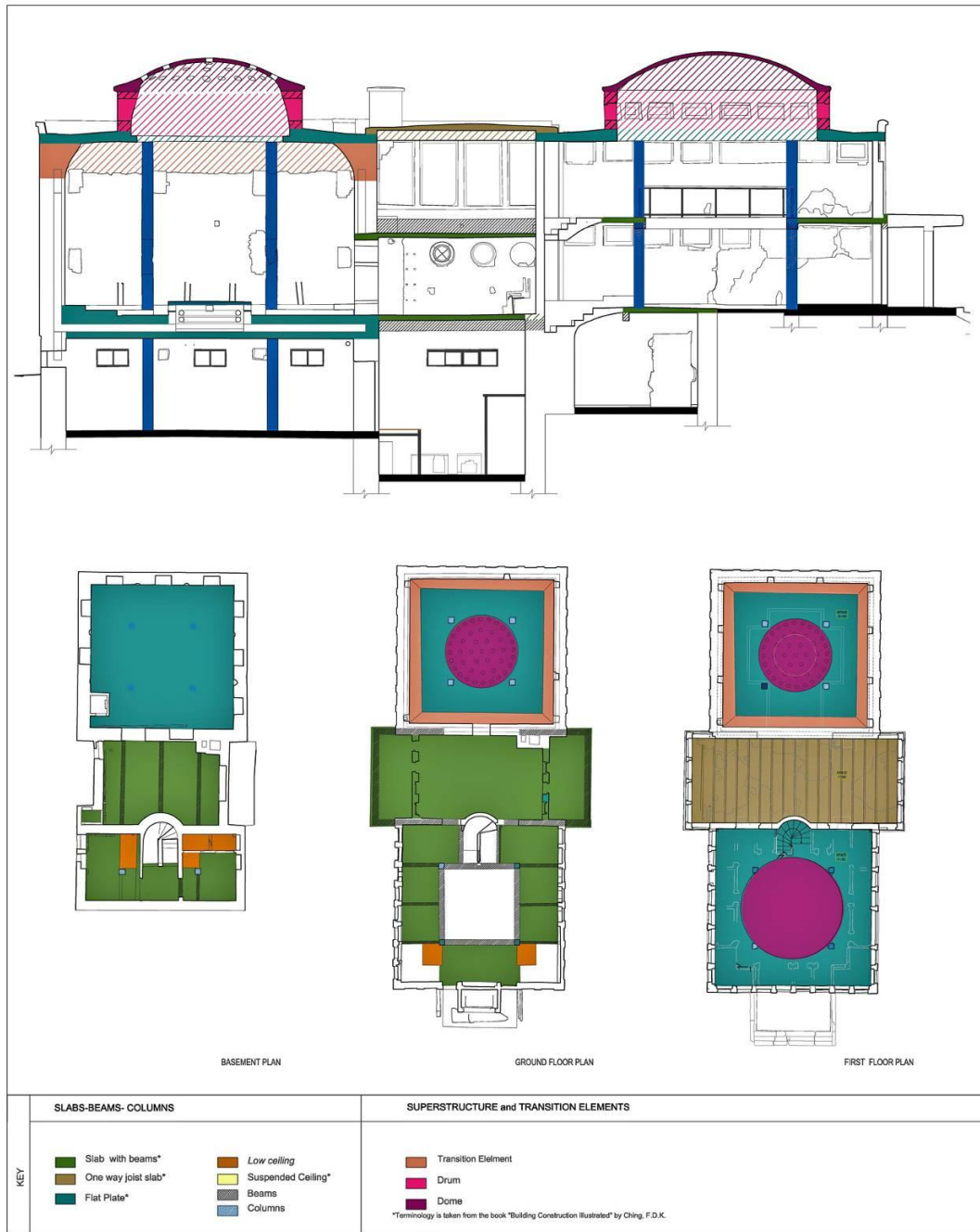
Figure 55- Reinforce Concrete System in AOÇ Hamam
