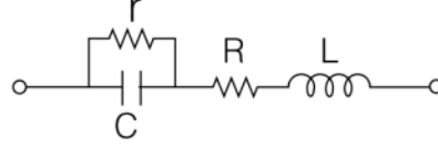
Figure 4.1 Capacitor equivalent circuit model [17]
