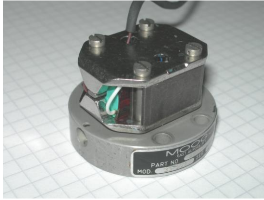
Figure 3-3 Electromagnetic torque motor of pitch trim actuator
