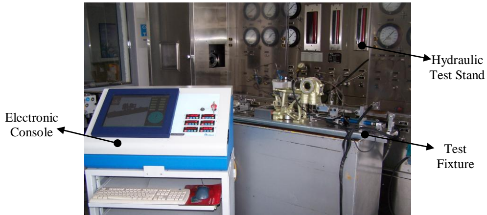
Figure 5-6 Electronic console and test fixture
