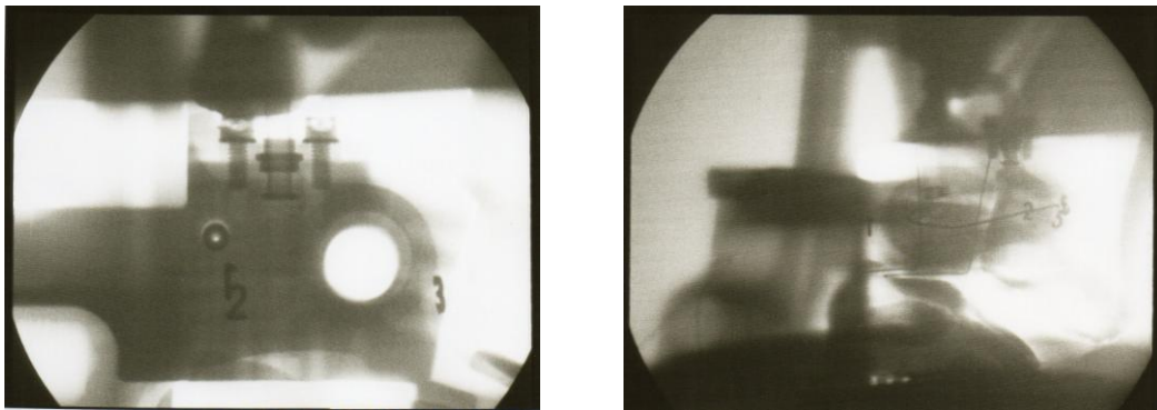
Figure 3-10 X-ray of pitch trim actuator
