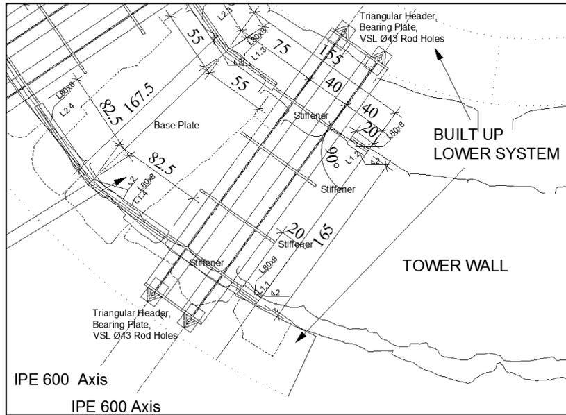
**Figure 4.17** View of Upper System: An Assembly composed of Two Beams and Base Plate
