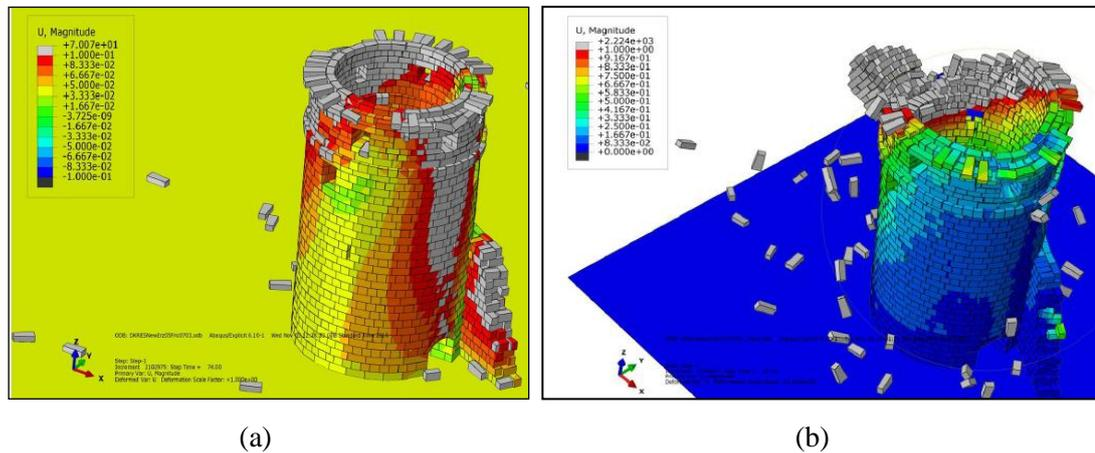
**Figure 3.9** a) Deformation at the Eastern Tower after being affect by the Erzincan ‘92 EQ with 0.5 Intensity Rate b) Deformation at the Eastern Tower during Excitation of the Erzincan ‘92 EQ with 1.0 Intensity Rate
