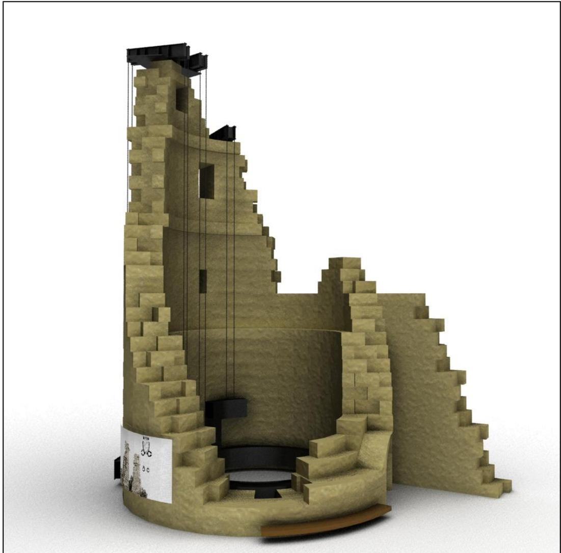
**Figure 4.24** 3D Max model representing possible form of the Eastern Tower after strengthening (model was made by Seray Türkay)
