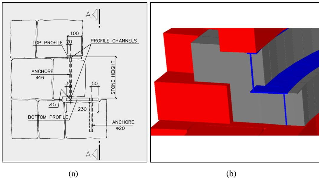
**Figure 2.26** (a) Side Section of Wall and Anchored-Lintel System Drawings SAYKA (2002). (b) 3D Side View of the Lintel System
