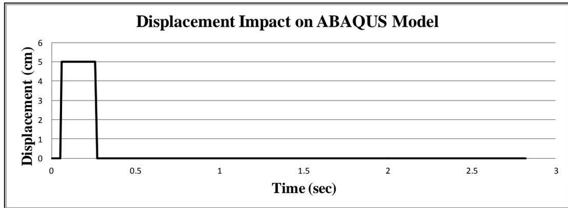
**Figure 3.21** Displacement Based Impact that was used to excite Analytical Model.
