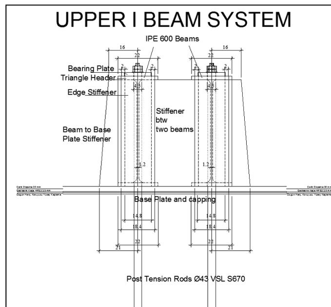
**Figure 4.16** Upper Beam System Assembly Front View
