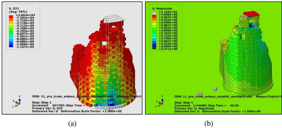
**Figure 4.9** Eastern Tower Model strengthened with Post-Tensioning System and loaded with the Synthetic EQ-02 a) S33 during PGA ( $t = 20$ ) of EQ b) Deformed Shape at the end of EQ
