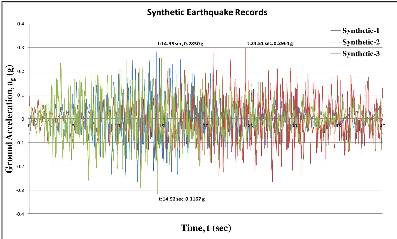
Figure 3.5 N-S Components of Synthetic EQs derived with RSCA Software
