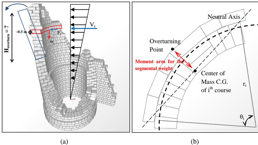
**Figure 3.14** a) Equivalent Earthquake Load affecting the Tower b) Calculation Assumptions for Each Stone Layer.
