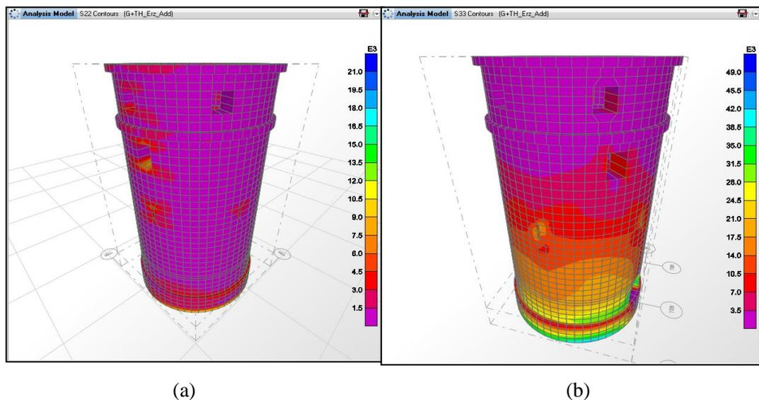
**Figure 3.7** Horizontal (S22) and Vertical (S23) tension stress distribution on linear modelling with effect of Erzincan Earthquake on the Eastern Tower; a) South-western View (S22 Distribution) b) Northeastern View (S33 Distribution)
