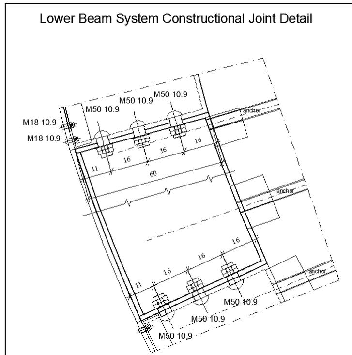
**Figure 4.12** Lower Beam System Constructional Joint Connection Detail (Plan Section)
