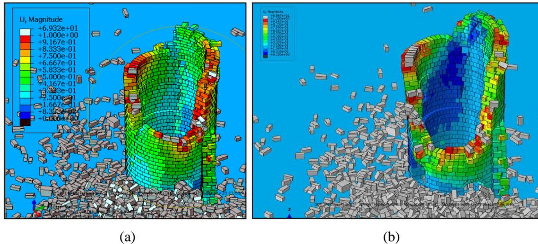
**Figure 3.10** a) Deformed Shape similar with Current One as a result of #5 analysis of Table 3.4 b) Result of the Analytical Model (#8 of Table 3.4) having same Analysis Parameters with #5 but addition of Later Period Eastern Gate (Existence of which is claimed by Mansel)
