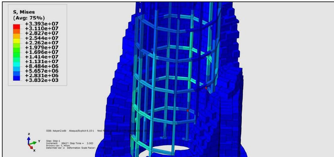
**Figure 4.4** Result of 2<sup>nd</sup> Model in which the Eastern Tower being strengthened: Von Mises Stress Distribution indicates High Stress Concentrations
