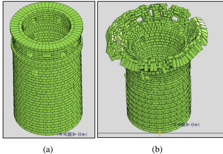
**Figure 3.8** DEM of the Eastern Tower formed by Non-Staggered Stone Blocks in Horizontal Plane, Representation of Tower during Seismic Excitation a) at the start of Erzincan EQ b) 5<sup>th</sup> sec of Erzincan '92 EQ
