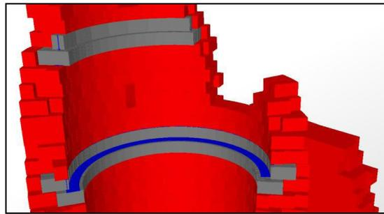
**Figure 2.23** 3D View of Lintel System and Eastern Tower (Lintels on 16<sup>th</sup> and 25<sup>th</sup> layers)
