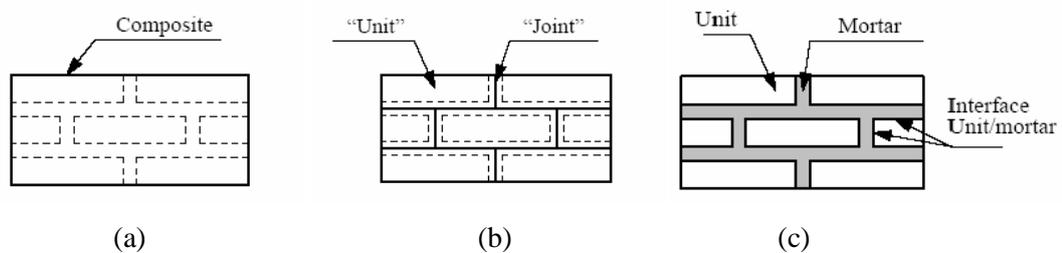
**Figure 3.1** a) Macro model b) Simplified Micro Model c) Detailed Micro Model
