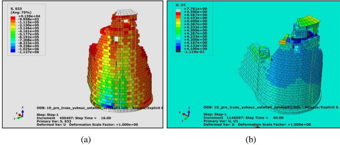
**Figure 4.8** Eastern Tower Model strengthened with Post-Tensioning System and loaded with the Synthetic EQ-01 a) S33 during PGA ( $t = 16$ ) of EQ b) Deformed Shape at the End of EQ
