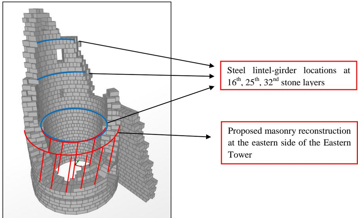
**Figure 4.20** The Reconstruction that was proposed in the Project of Strengthening with Lintel-Girder System.
