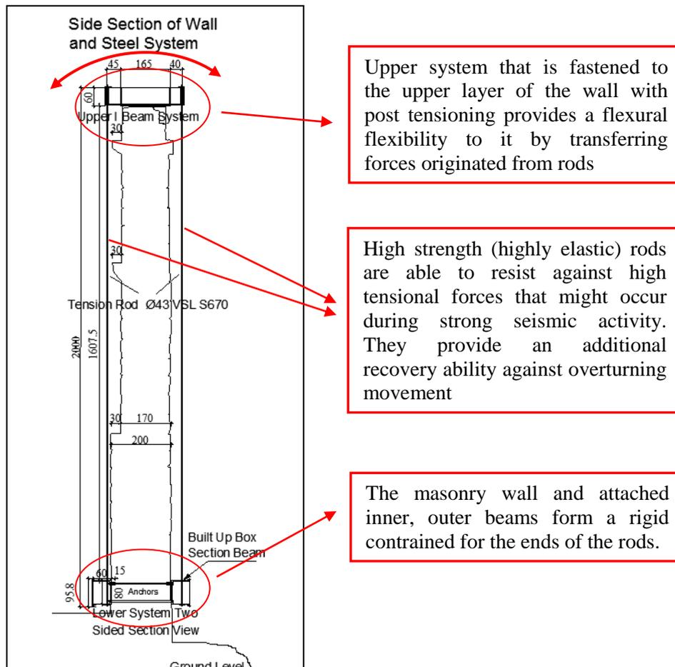
**Figure 4.19** Side Section of the Tower and the Strengthening System
