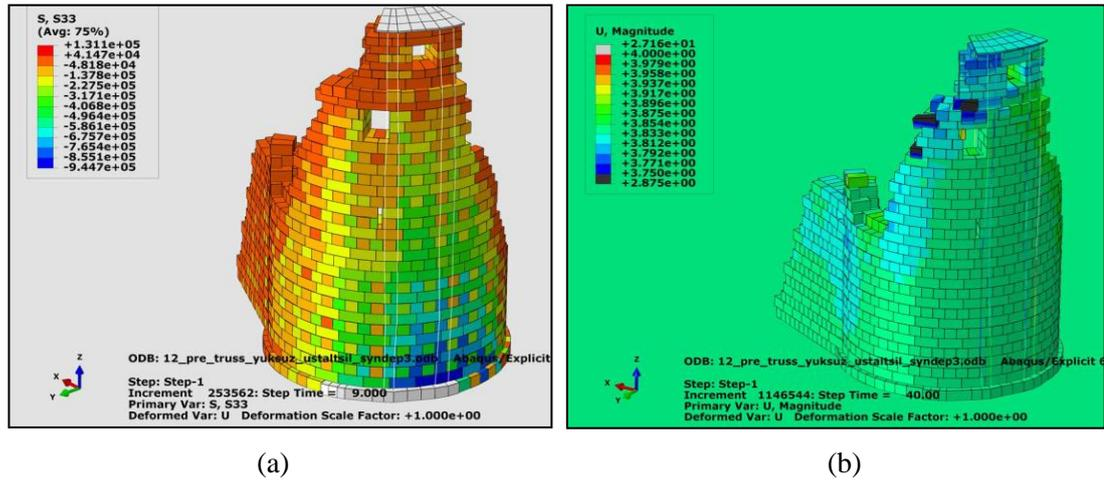
**Figure 4.10** Eastern Tower Model strengthened with Post-Tensioning System and loaded with the Synthetic EQ-03 a) S33 during PGA (t = 20 ) of EQ b) Deformed Shape at the end of EQ.
