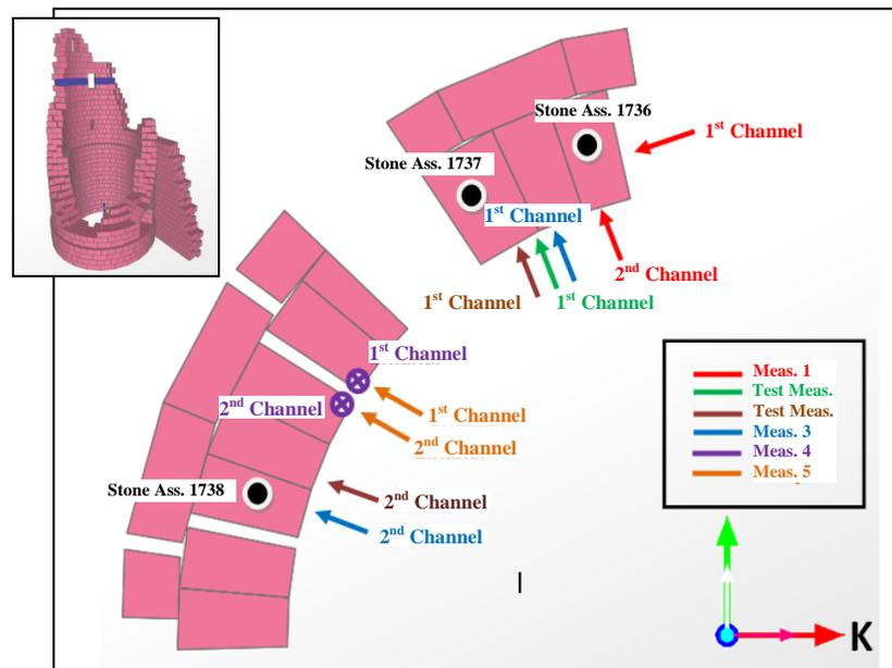
**Figure 3.16** Field-Dynamic Testing, Measurement Scheme
