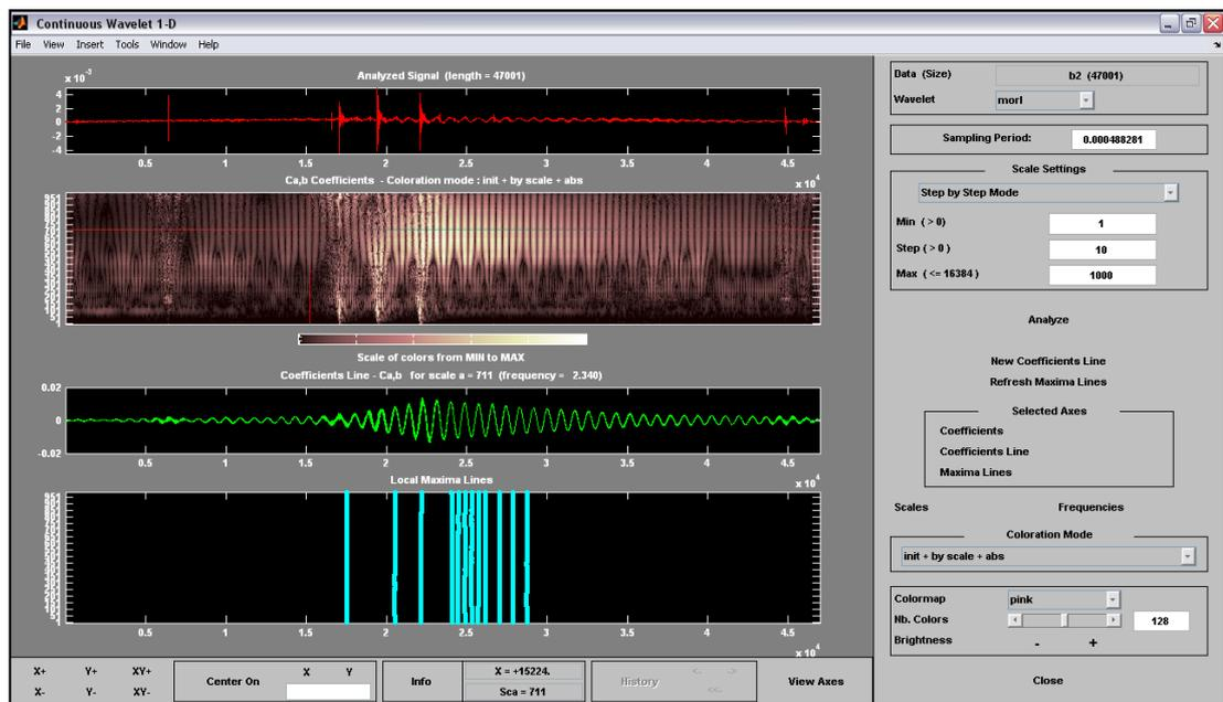
**Figure 3.20** Wavelet Analysis on Data of 4<sup>th</sup> Measurement 2<sup>nd</sup> Channel which was excited by wind (First Modal Frequency Value corresponding to Flexural Behaviour was found as 2.340 Hz)
