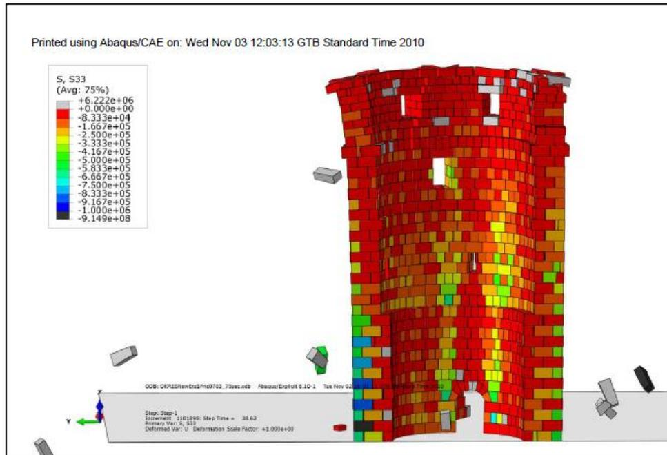
**Figure 3.12** Vertical Compressive Stress Distribution during 3<sup>rd</sup> sec of #5 Analysis.
