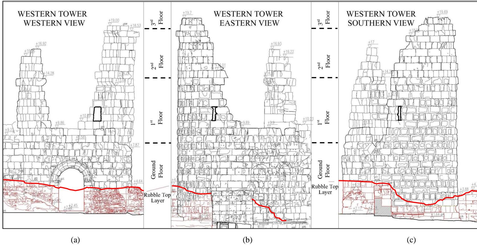
**Figure 2.10** Drawings of the Western Tower a) Western View b) Eastern View c) Southern View - SAYKA (2002, Revised in 2010)
