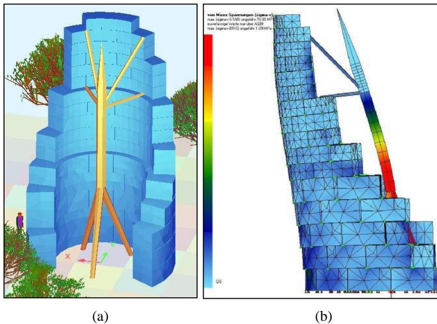
**Figure 2.27** (a) Tripod System 3D View. (b) Discrete Analytical Modelling, Pushover Analysis - Limit State Result Representation.
