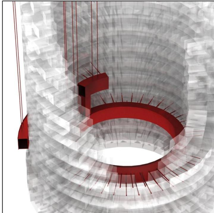
**Figure 4.15** 3D Max representation of the Eastern Tower post-tensioning system lower part view made by Seray Turkey.
