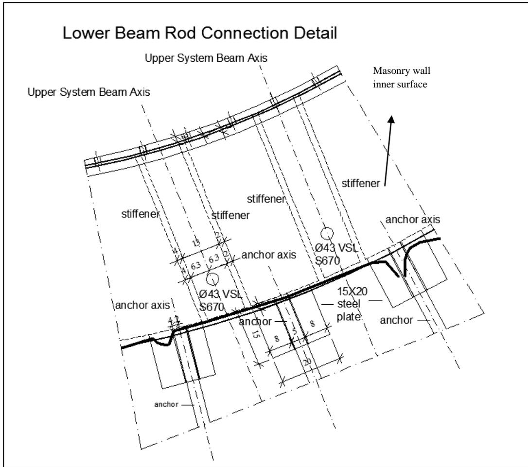
**Figure 4.14** Lower Beam System – Post Tension Rod Connection Detail (Plan Section)
