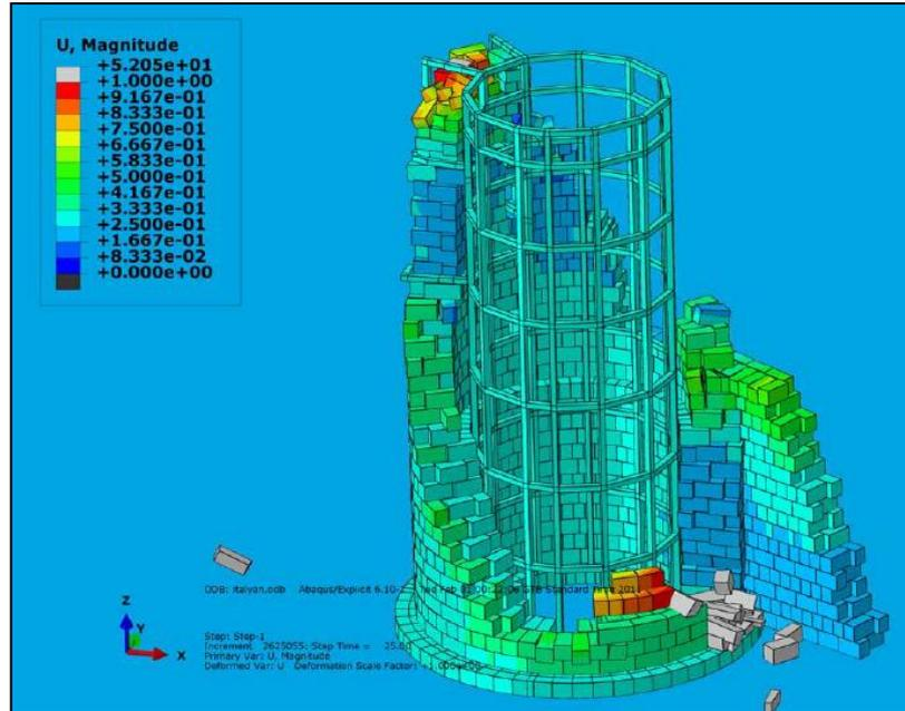
**Figure 4.3** Deformation of the Eastern Tower with Pipe Steel System during PGA of Erzincan '92 EQ
