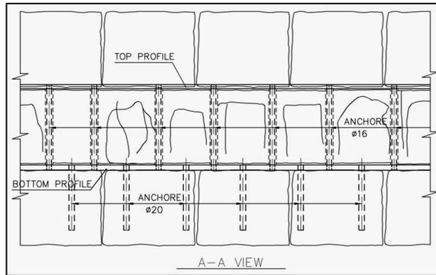
**Figure 2.25** Frontal View, Drawing of the Lintel System SAYKA (2002)
