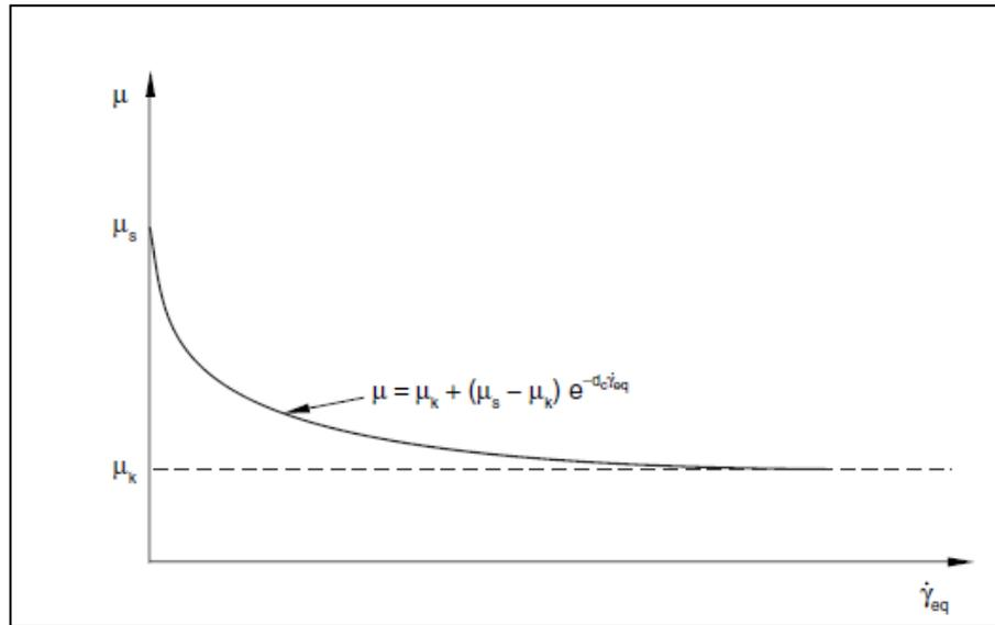
**Figure 3.3** Transition Behaviour Between Static and Kinetic Frictional Coefficients
