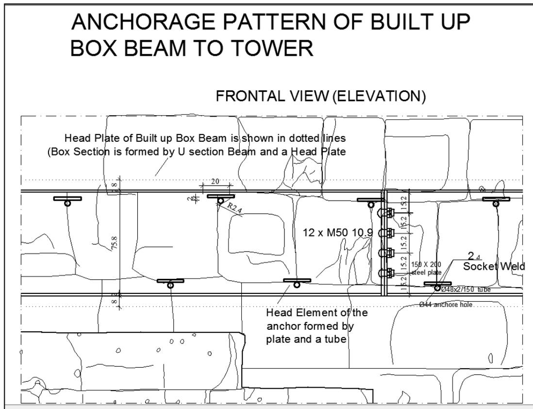
**Figure 4.13** Anchorage Pattern View of Lower Box Beam System to the Tower
