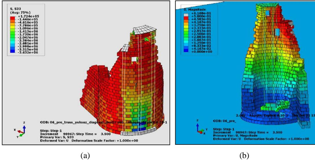
**Figure 4.7** Results of the Eastern Tower Model strengthened with Post-Tensioning System including Additional Diagonal Rods : The Moment of PGA of Erzincan ‘92EQ a) S33 (Vertical) Stress Distribution b) Displacement Distribution
