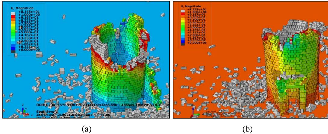
**Figure 3.11** a) Result of Analyses #9 having same Parametric and Geometric Condition with #5 except, Lack of Loopholes and Windows at City Side of the Tower b) Results of Analyses #10 made on the Western Tower. Analysis having the same Parametric Conditions with #5
