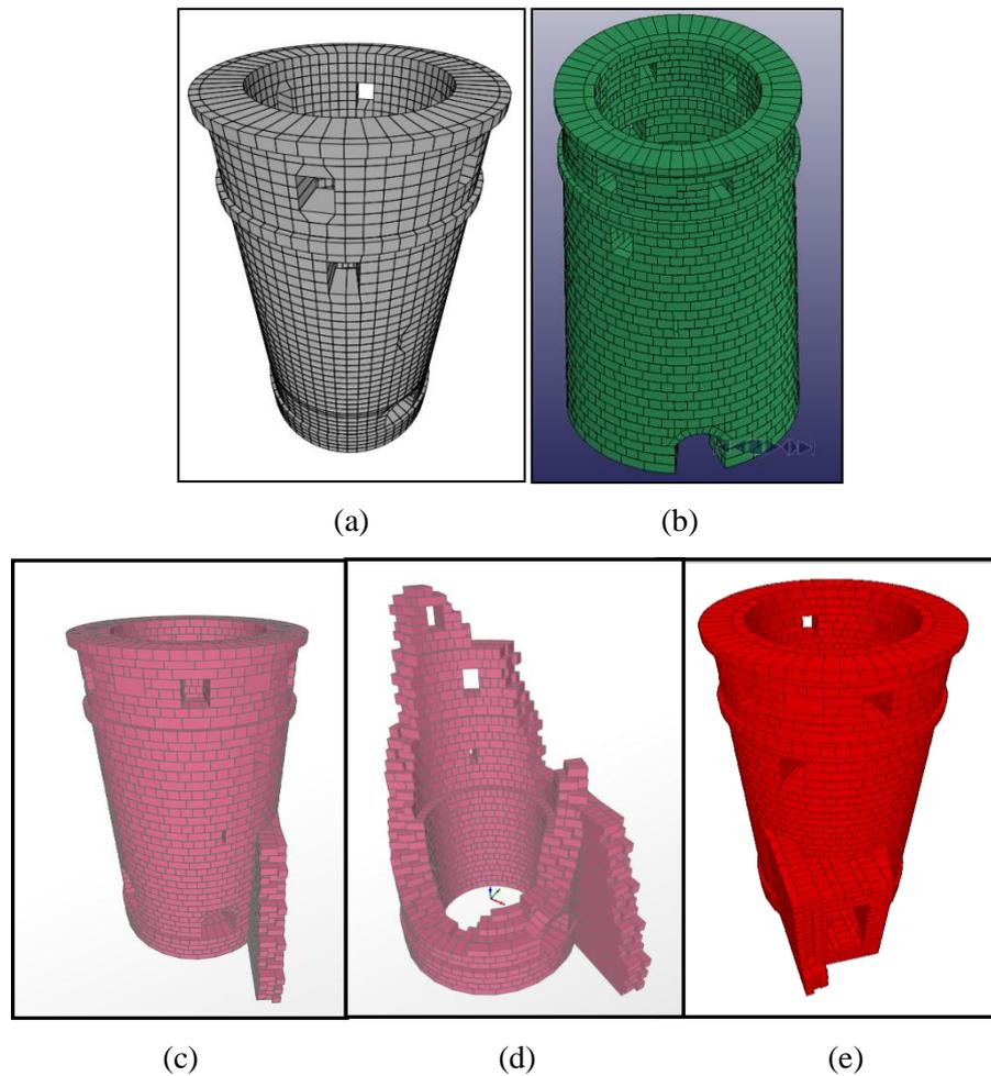
**Figure 3.2** a) SAP2000 Model of the Original Eastern Tower b) Ls-DYNA DEM of the Original Eastern Tower c) ABAQUS DEM of the Original Eastern Tower d) ABAQUS DEM of the Ruined Eastern Tower e) ABAQUS DEM of the Original Western Tower
