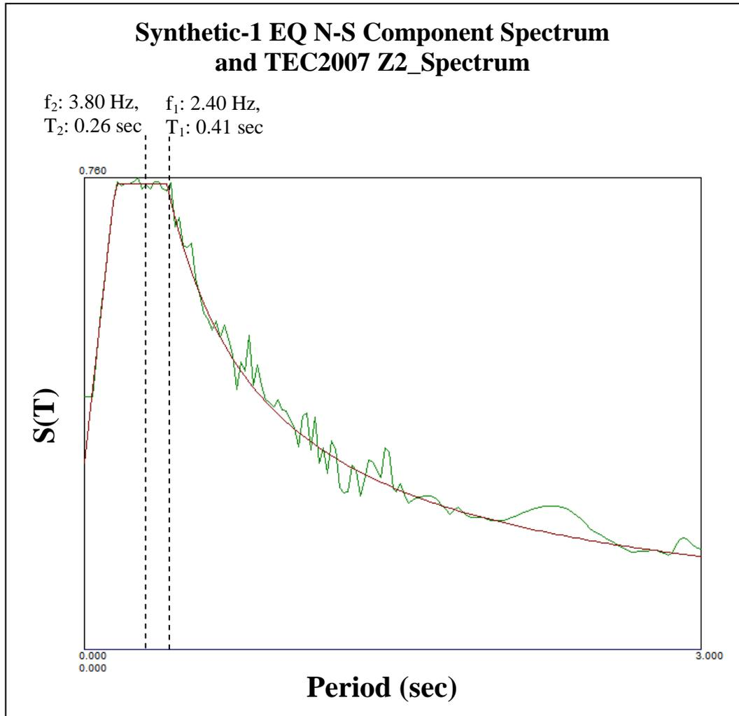
**Figure 3.6** Response Spectrum of Synthetic-1 EQ N-S Direction. Correlation between TEC2007 Z2 Spectrum and Synthetic one
