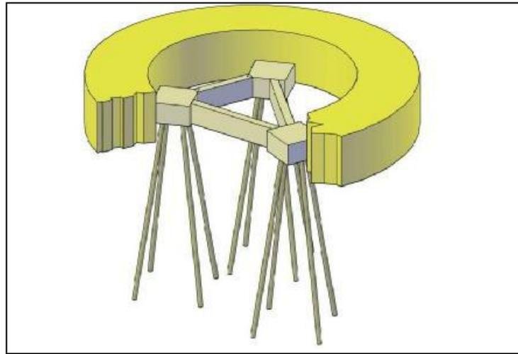
**Figure 4.21** Foundation System that was suggested by German Team to carry Tripod Structure
