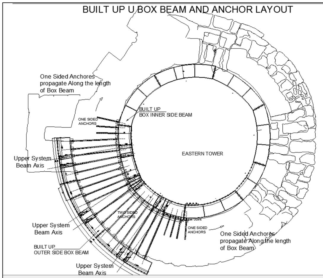
**Figure 4.11** Lower System Anchorage Pattern
