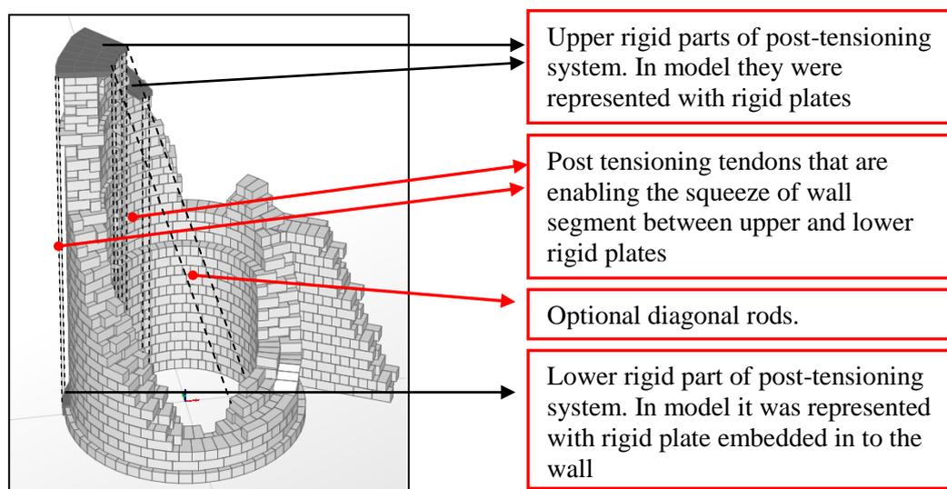
**Figure 4.5** Eastern Tower Strengthening Model: Post-Tensioning System
