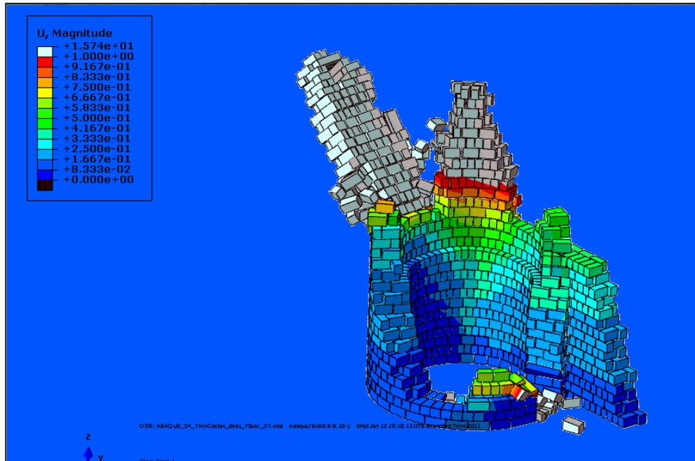
**Figure 3.13** Overturning of Upper Part of the Current Eastern Tower under Seismic Action.
