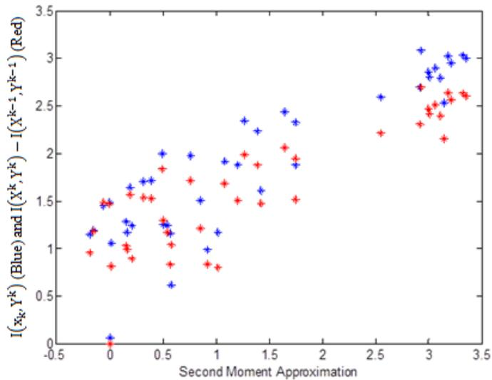
Figure 4.11 Correlation plot of the second moment approximation and the observability measures for Case 3. Blue:  $I(x_k, Y^k)$  vs. the Second Moment Approximation. Red: Difference  $I(x^k, Y^k) - I(x^{k-1}, Y^{k-1})$  vs. the Second Moment Approximation
