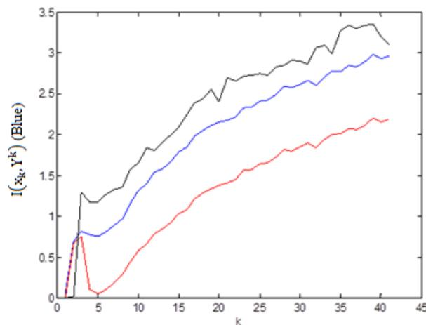
Figure 4.8 The observability measures between the last state and the measurements: The blue line is  $I(x_k, Y^k)$ ; Red line is  $I(X^k, Y^k) - I(X^{k-1}, Y^{k-1})$ ; Black line is the Second Moment Approximation for Case 2
