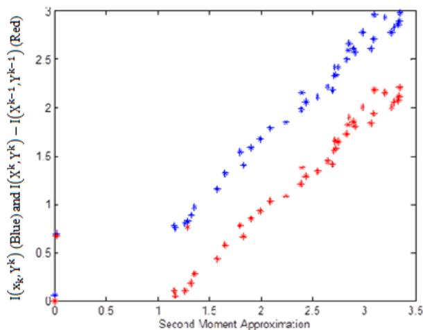
Figure 4.9 Correlation plot of the second moment approximation and the observability measures for Case 2. Blue:  $I(x_k, Y^k)$  vs. the Second Moment Approximation. Red: Difference  $I(X^k, Y^k) - I(X^{k-1}, Y^{k-1})$  vs. the Second Moment Approximation
