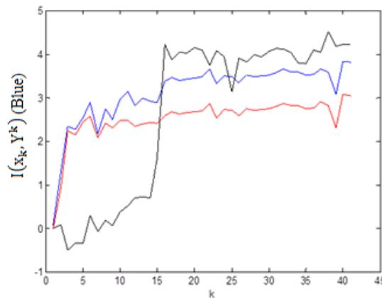
Figure 4.6 The observability measures between the last state and the measurements: The blue line is  $I(x_k, Y^k)$ ; Red line is  $I(X^k, Y^k) - I(X^{k-1}, Y^{k-1})$ ; Black line is the Second Moment Approximation for Case 1
