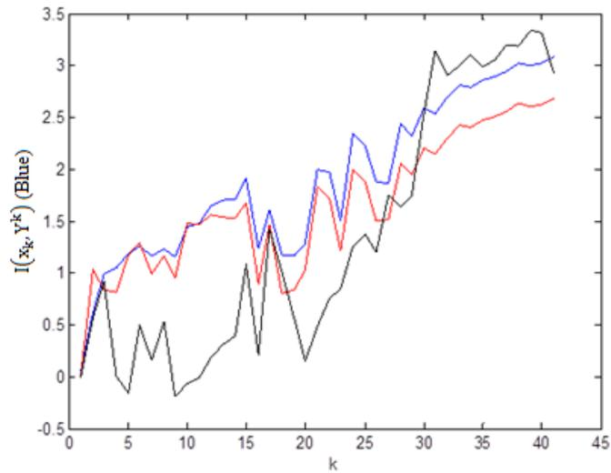
Figure 4.10 The observability measures between the last state and the measurements: The blue line is  $I(x_k, Y^k)$ ; Red line is  $I(x^k, Y^k) - I(x^{k-1}, Y^{k-1})$ ; Black line is the Second Moment Approximation for Case 3
