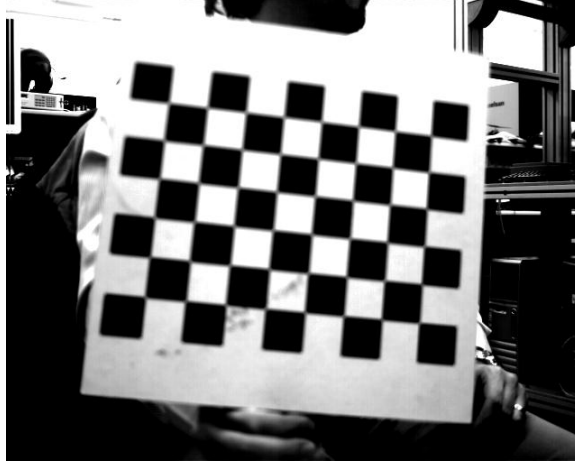
Figure 4 Calibration Pattern utilized during simulations
