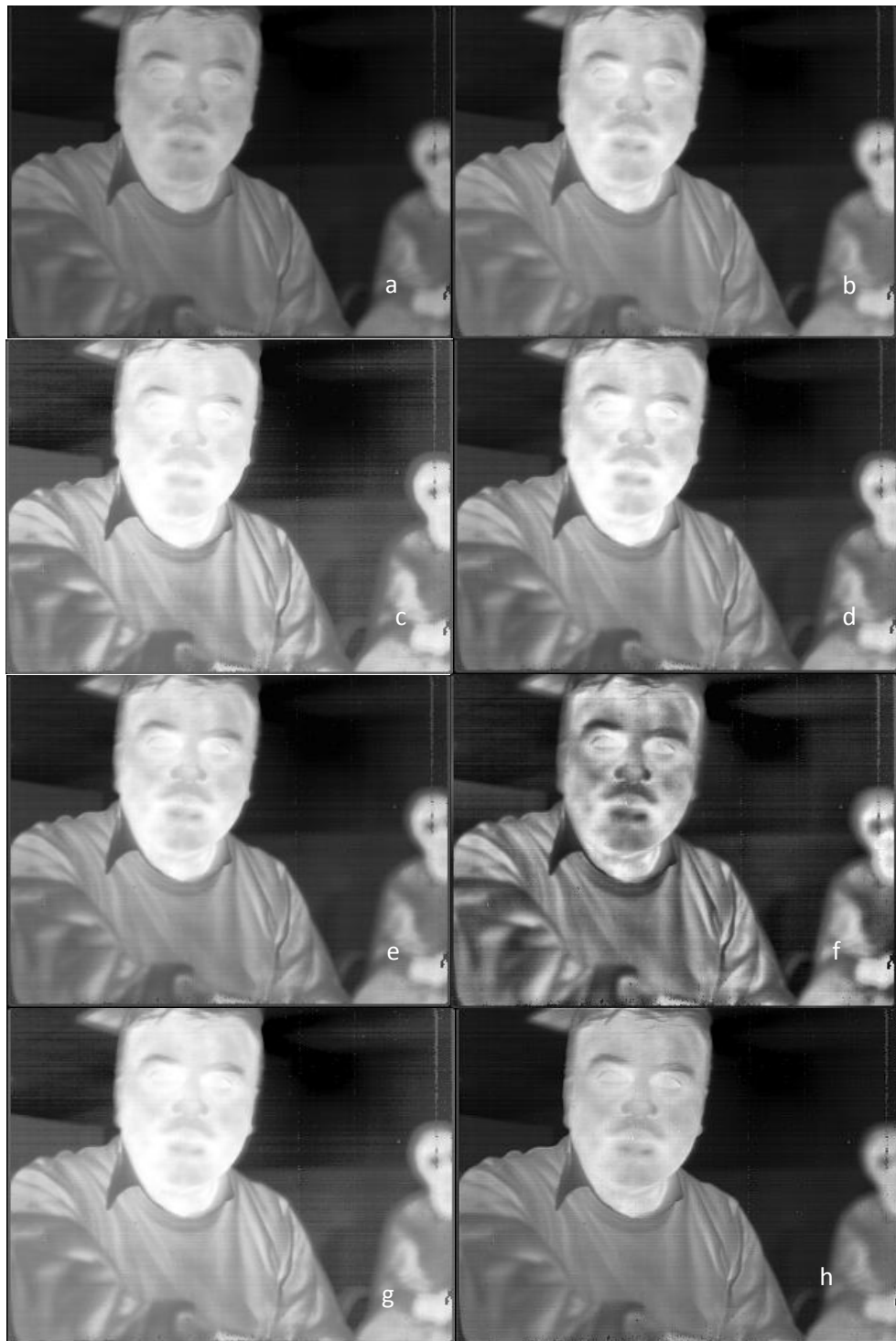
Figure 4.13 Results of contrast enhancement methods a) raw image, b) image result of contrast stretching c) image result of histogram equalization, d) image result of plateau method proposed by Wang et al., e) image result of plateau method proposed by Lai et al., f) CLAHE, g) SMQT, and h) Unsharp masking.
