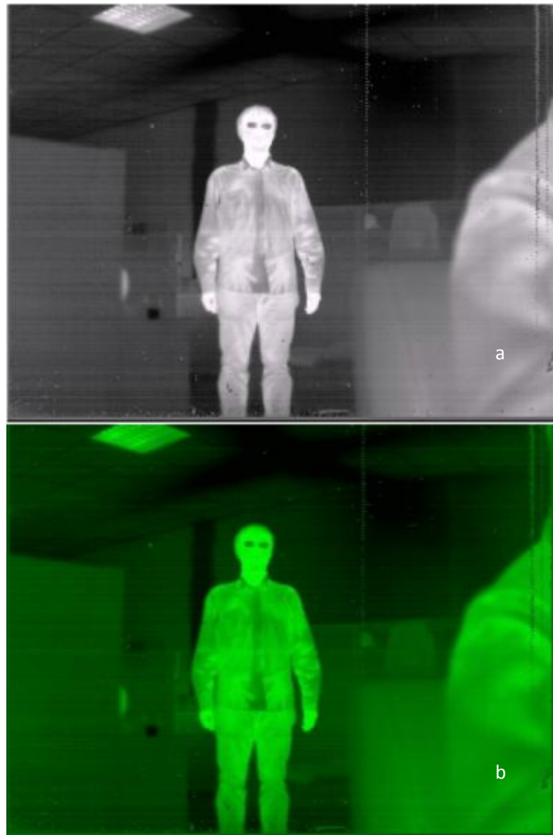
Figure 6.3 a) Raw image, b) Pseudo colored image by directly mapping gray levels to green channel.
