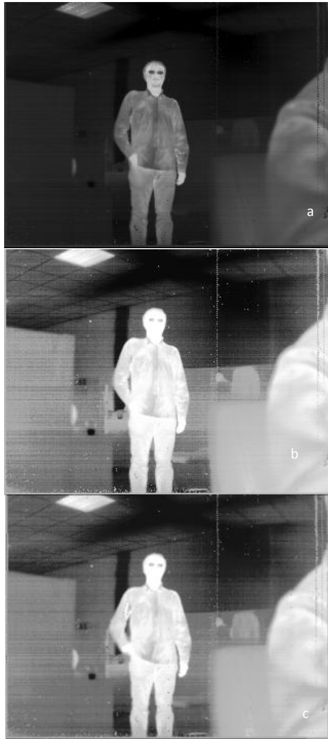
Figure 7.4 Histogram equalization results: a) Original image, b) MATLAB prototype, c) Output of the device.
