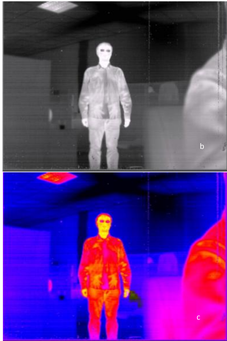
Figure 6.4 Hot-metal scale pseudo coloring with a linearly interpolated palette: a) The palette used for transformation, b) Raw image, and c) Pseudo colored image.
