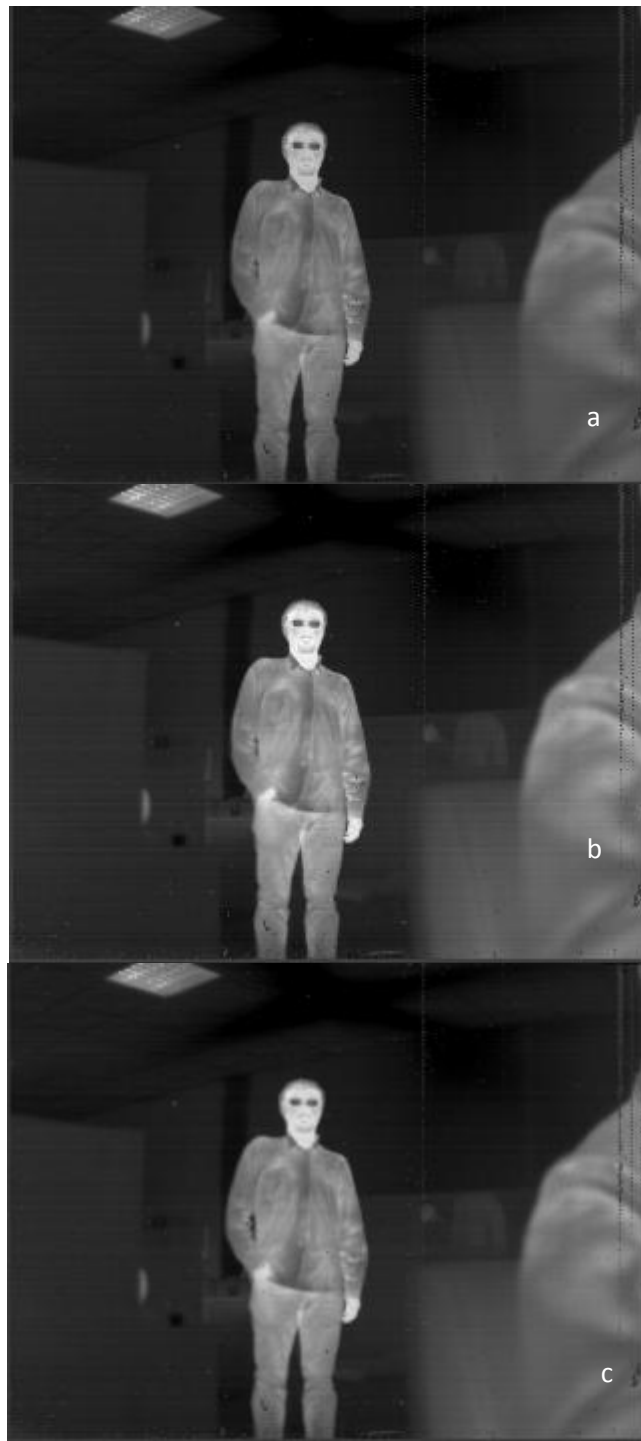
Figure 7.3 Contrast stretching method results: a)Original image, b) MATLAB prototype, c) Output of the device.
