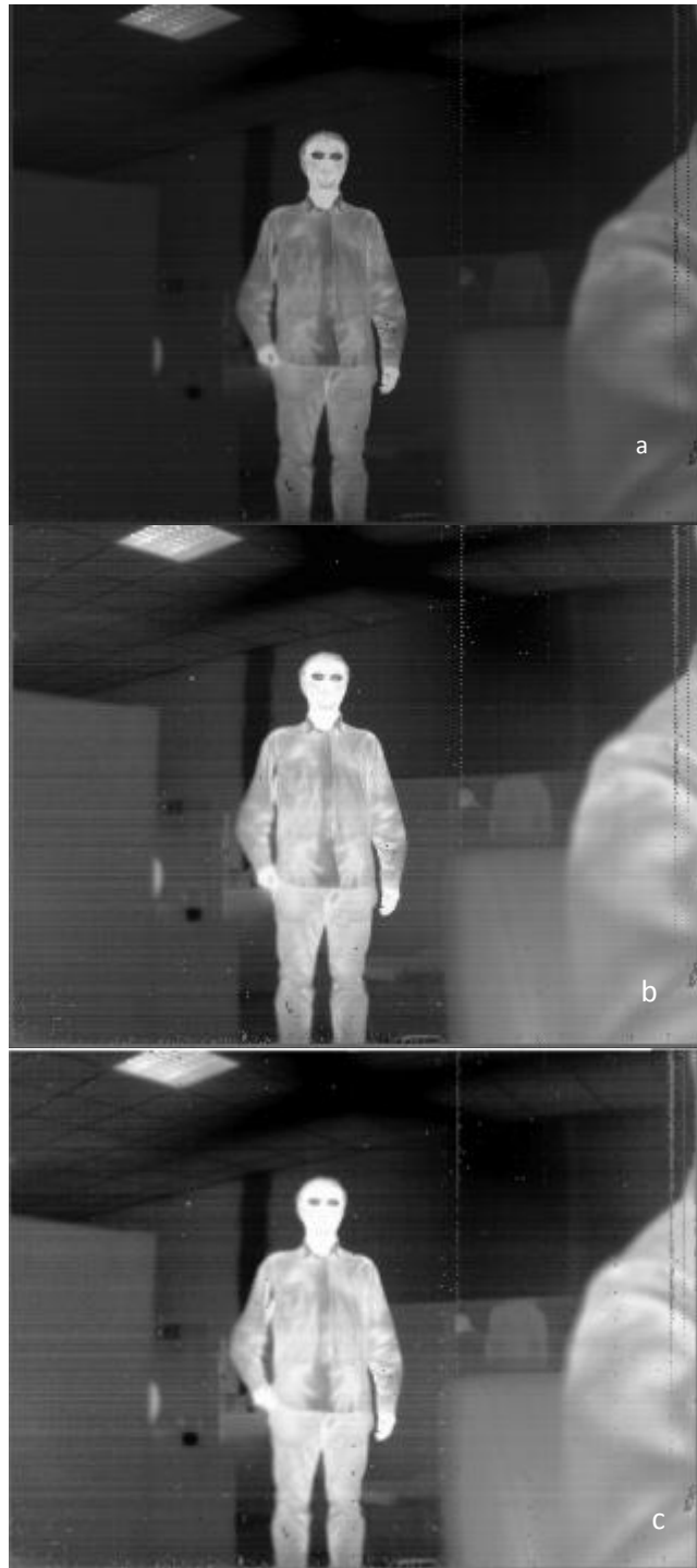
Figure 7.6 Results of plateau method proposed by Lai et al.: a) Original image, b) MATLAB prototype, c) Output of the device.
