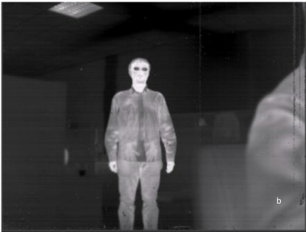
Figure 4.1 a) Raw image, b) Image enhanced with contrast stretching.
