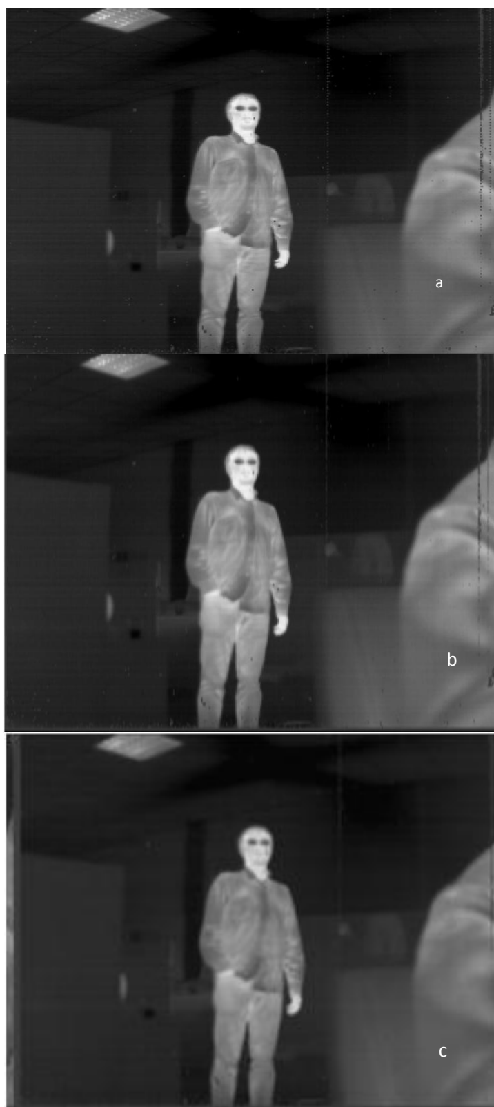
Figure 7.7 Noise reduction method results: a) Original image, b) MATLAB prototype, c) Output of the device.
