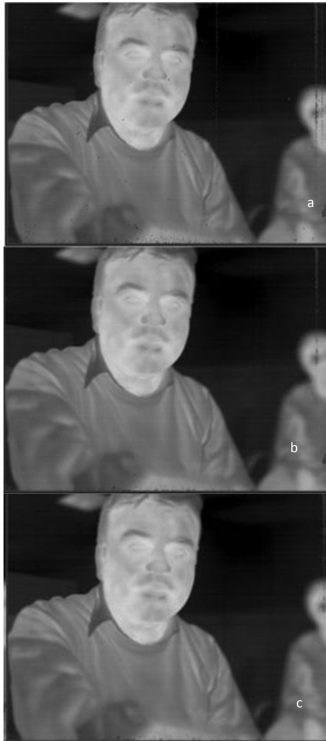
Figure 7.2 Defective pixel correction results: a) Original image, b) MATLAB prototype, c) Output of the device.
