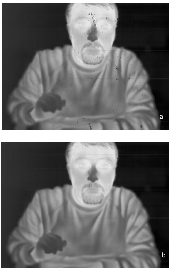
Figure 8.2 a) Raw image, b) Image result of improved defective pixel correction algorithm.
