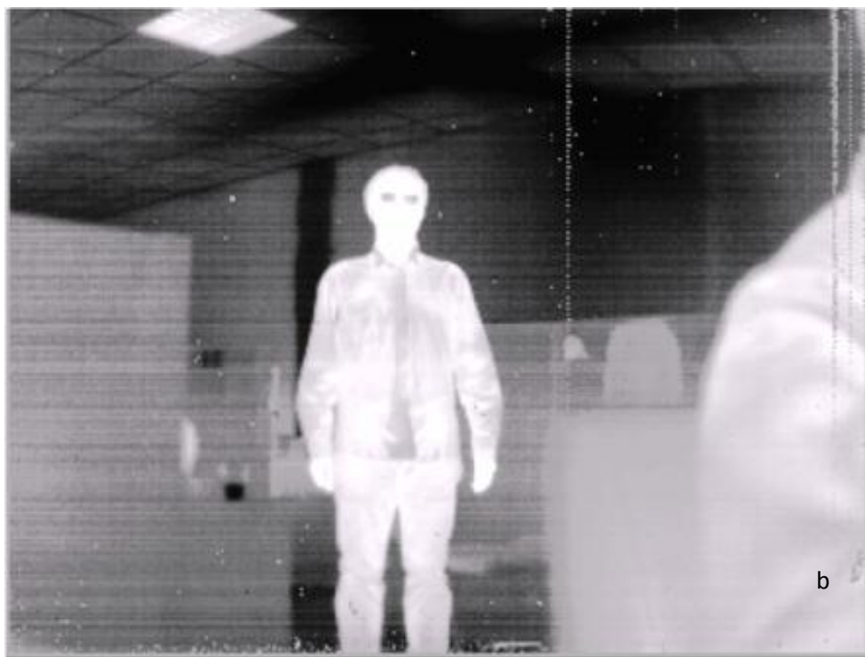
Figure 4.2 a) Raw image, b) Image enhanced with histogram equalization.
