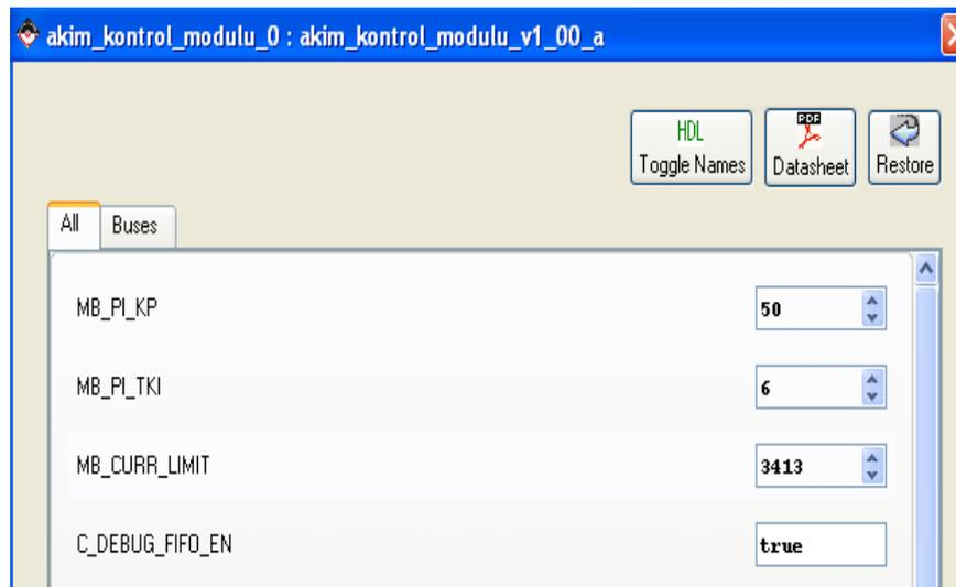
Figure 3.3: Configurable parameters window of the current controller on the EDK platform
