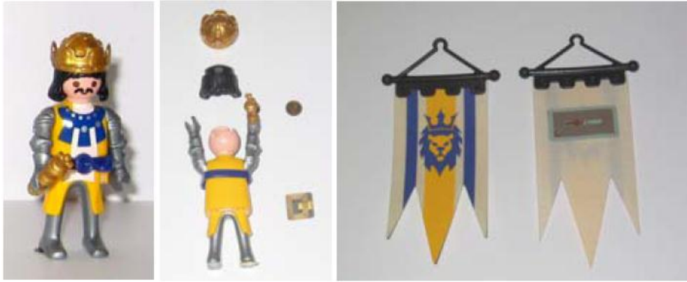
Figure 2.13 Unobtrusive Integration of RFID Technology into Elements
