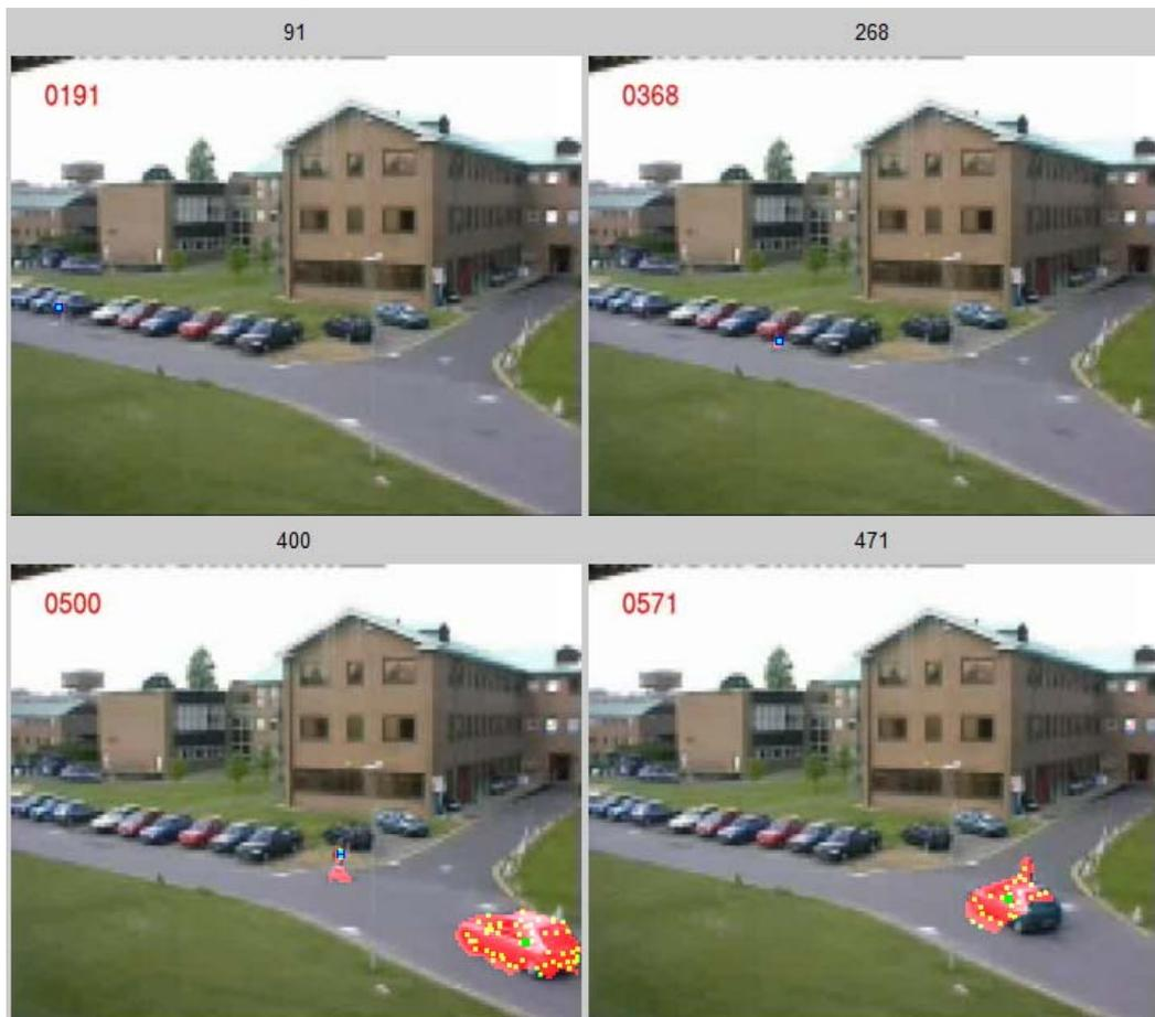
Figure 57 – Tracking results of PETS 2001 sequence with PF2D-OF
