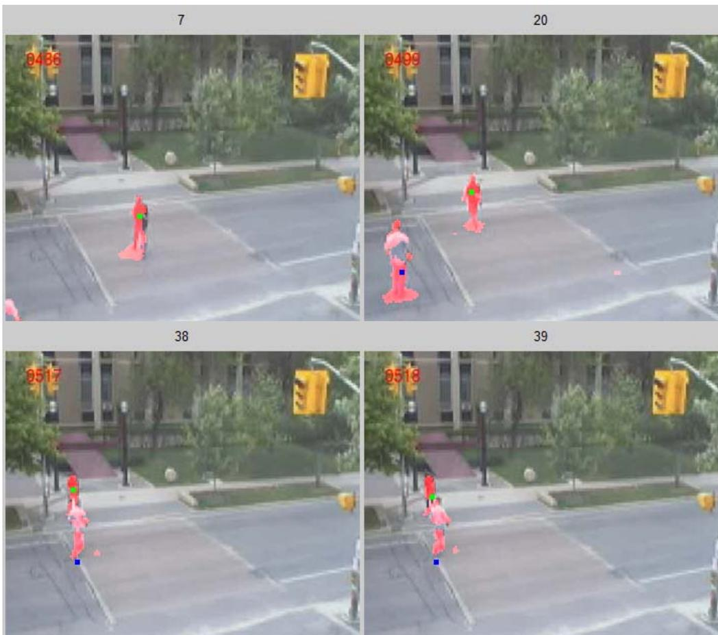
Figure 43 – Tracking results of St. George sequence with KF4D
