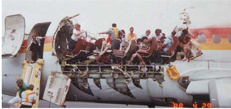
Figure 1.1: Aloha Airlines Boeing 737-200 experienced explosive decompression after 89,681 flight cycles [2]
