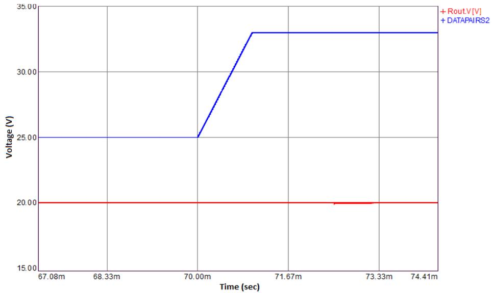
Figure 62 Input Voltage Change from 25V to 33V (Blue Line) and Output Voltage Response (Red Line)
