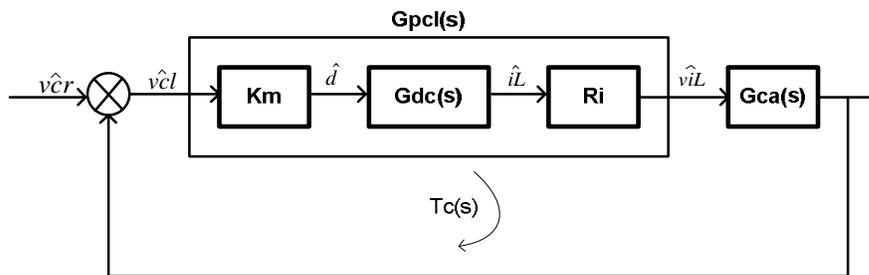
Figure 32 Current Loop Block Diagram
