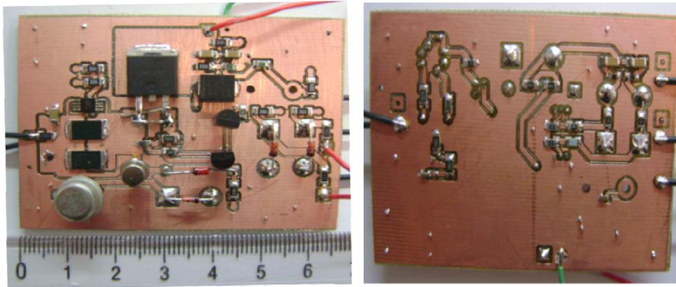
Figure 94 Foldback Current Limiter Top and Bottom View
