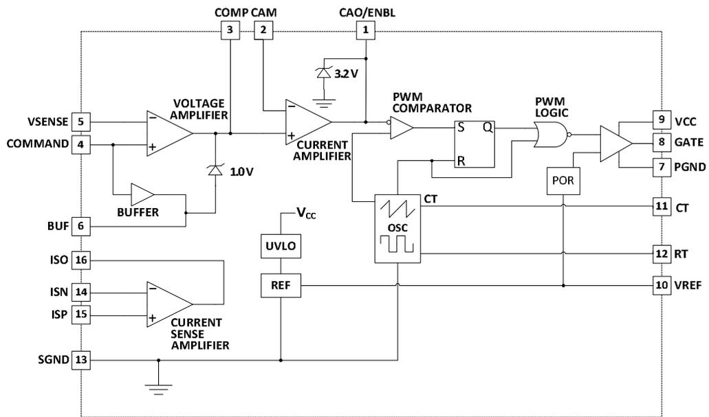
Figure 42 Block Diagram of UC3886 [70]
