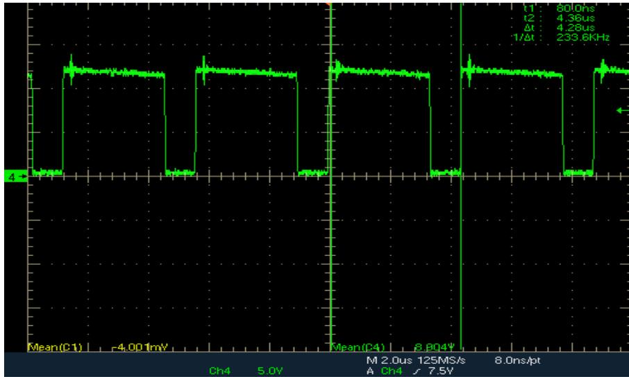
Figure 78 PWM waveform (CH4-Green) for  $V_{in}=28V$  and  $V_{out}=20\Omega$
