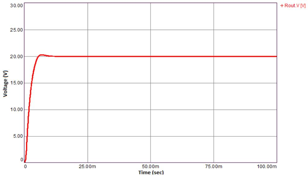
Figure 53  $V_{out}$  for  $V_{in}=28V$  and  $R_{out}=20\Omega$
