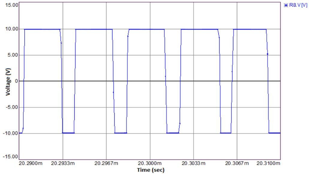
Figure 56 PWM Output (R8.V)
