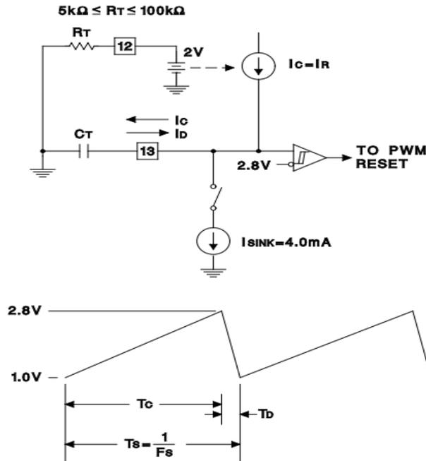
Figure 44 UC3886 Oscillator Waveform [24]
