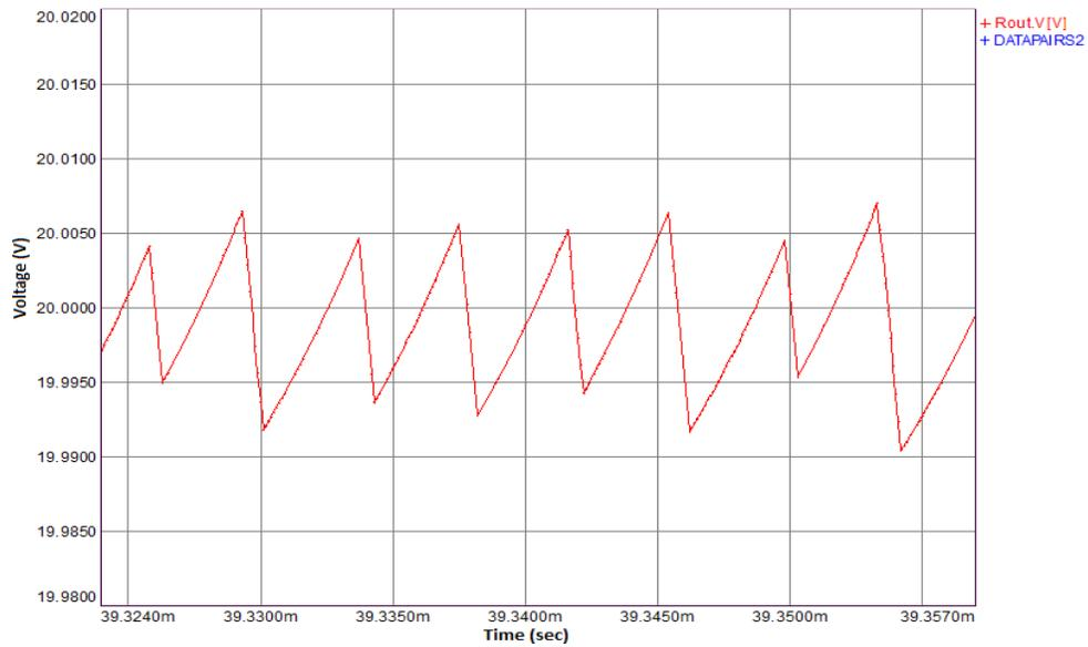
Figure 63 Output Voltage Ripple at  $V_{in}=25V$
