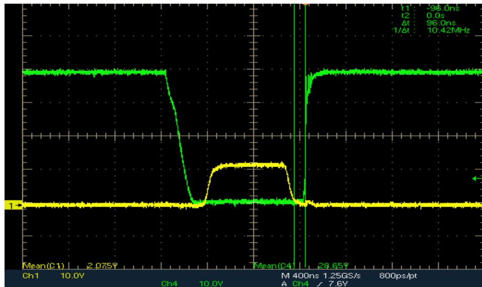
Figure 83 Delay between Low Side (CH1-Yellow) and High Side (CH4-Green) Switch Drive Pulses
