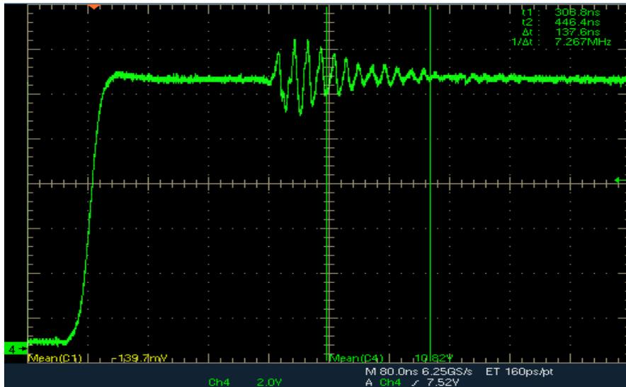
Figure 79 Zoomed View for the Ringing in the PWM waveform (CH4-Green)
