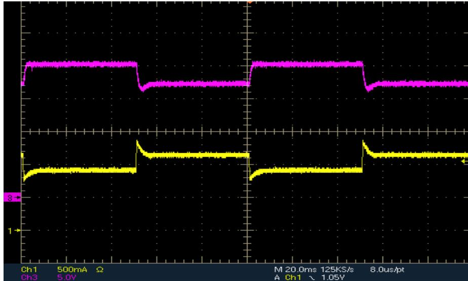
Figure 87 Output Voltage (CH3-Purple) and Current Waveforms (CH1-Yellow) for Rout Change from 22Ohm to 12Ohm
