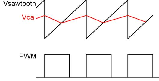
Figure 34 PWM Pulses and Control Voltage Waveforms
