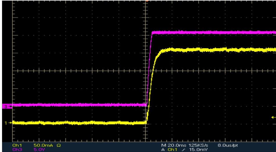
Figure 84 Output Voltage (CH3-Purple) Rise from 0V to 20V and Output Current (CH1-Yellow) Rise from 0A to 200mA
