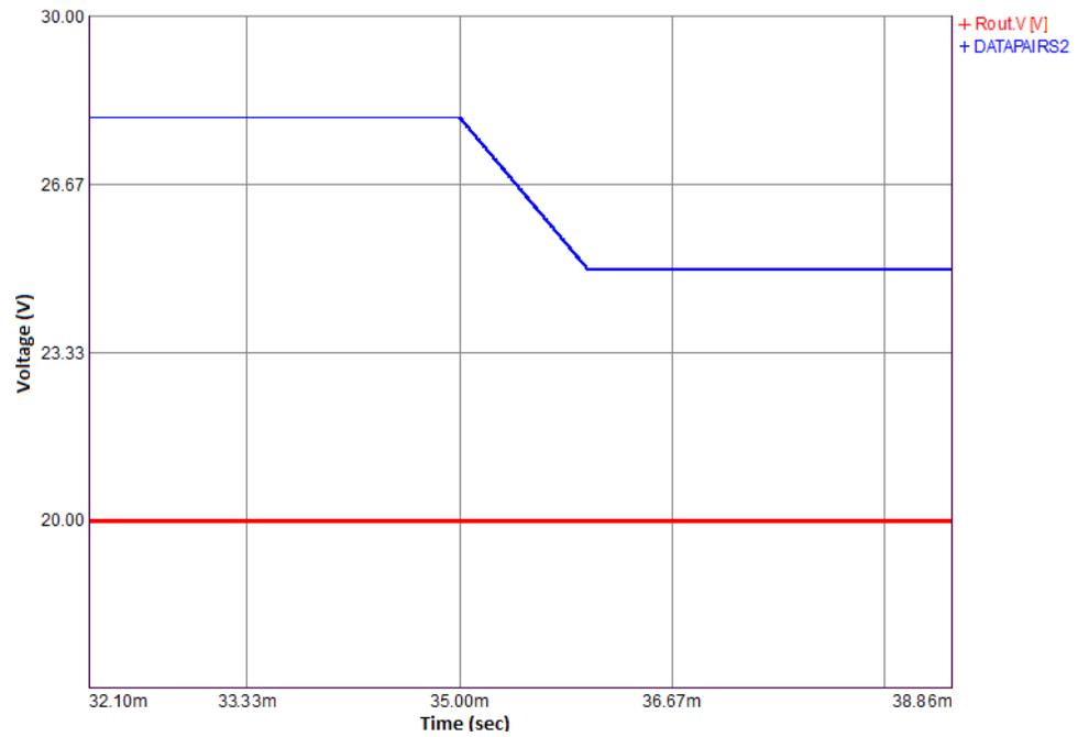
Figure 61 Input Voltage Change from 28V to 25V (Blue Line) and Output Voltage Response (Red Line)
