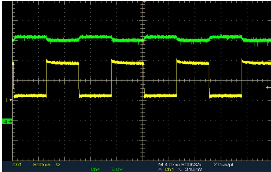
Figure 86 Output Voltage (CH4-Green) and Current (CH1-Yellow) Waveforms for  $R_{out}$  Change from 200 $\Omega$  to 20 $\Omega$
