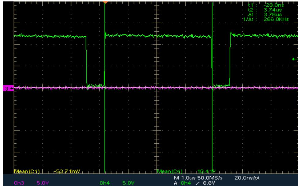
Figure 73 PWM pulses (CH4-Green) for VSENSE=1.922V
