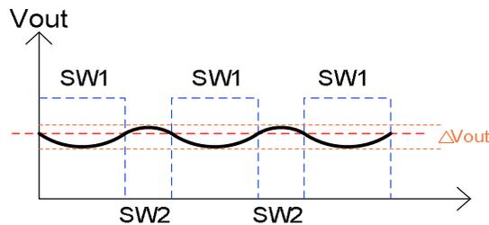
Figure 13 Waveform for  $V_{out}$
