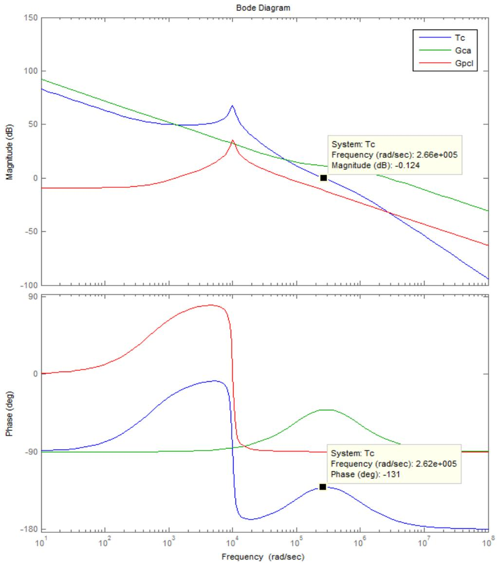
Figure 39 Bode Plot for  $T_c(s)$ ,  $G_{ca}(s)$  and  $G_{pcl}(s)$
