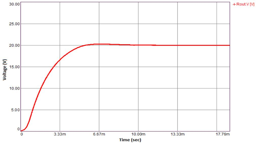
Figure 54 Settling Time for Vout for  $V_{in}=28V$  and  $R_{out}=20\Omega$
