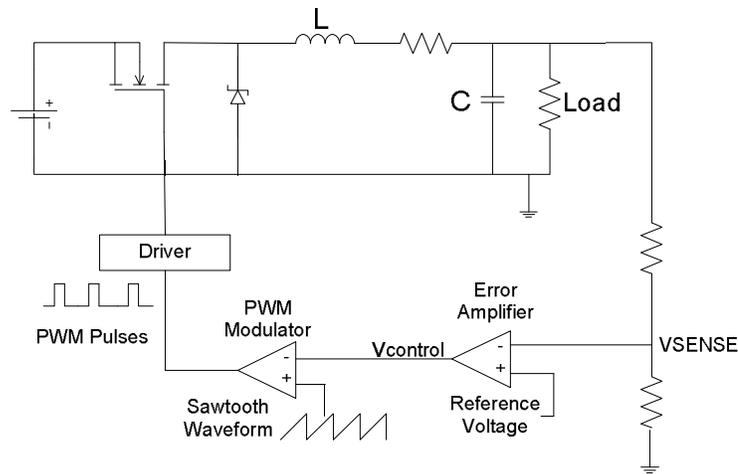
Figure 22 Voltage Mode Control
