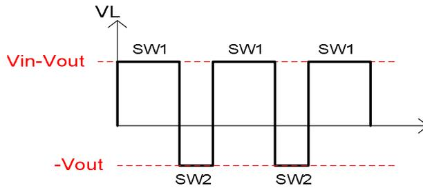
Figure 12 Waveform for  $V_L$
