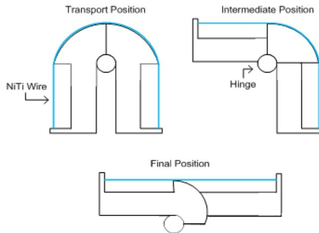
Figure 90 SMA Hinge [45, 55]
