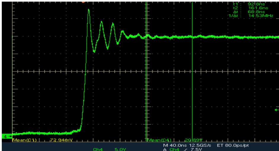
Figure 81 Zoomed View for the Ringing in the Freewheeling Diode (CH4-Green)
