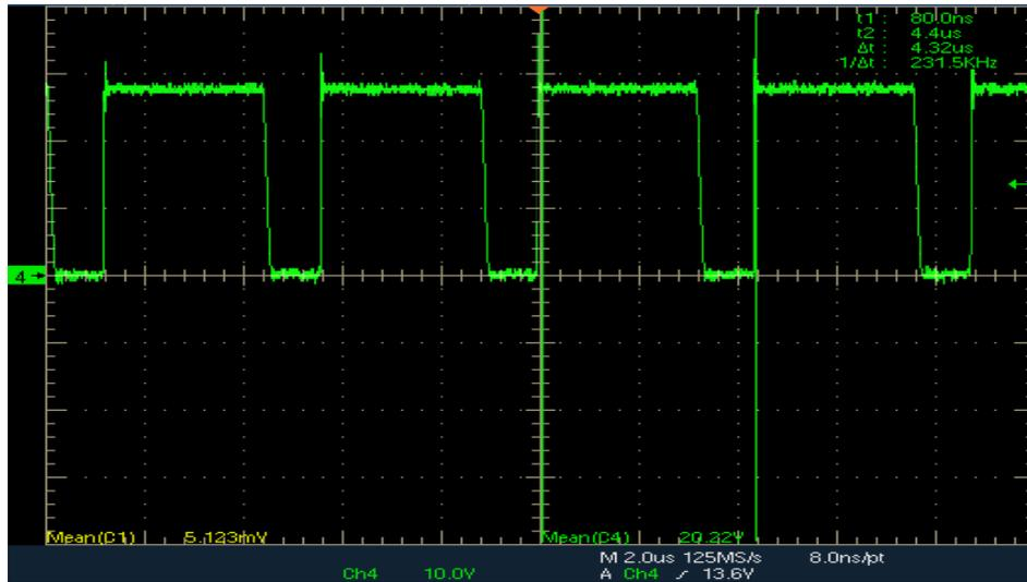
Figure 80 Waveform of the Freewheeling Diode (CH4-Green)
