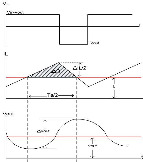
Figure 19 Buck Converter Output Voltage Ripple
