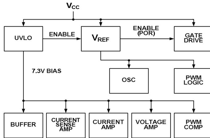
Figure 43 Power Distribution Blocks within UC3886 [70]
