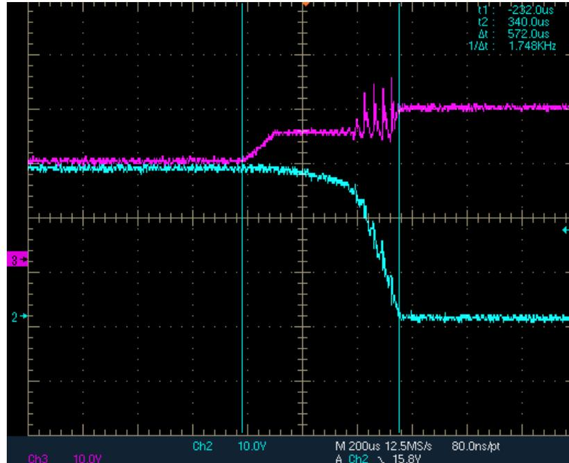
Figure 95 MOSFET Switch Turn Off during an overload
