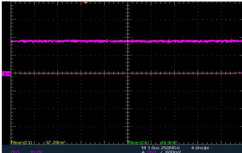
Figure 71 Output Voltage Waveform (20V) for  $V_{in}=28V$
