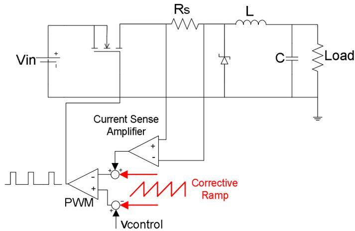
Figure 24 Slope Compensation in Current Mode Control
