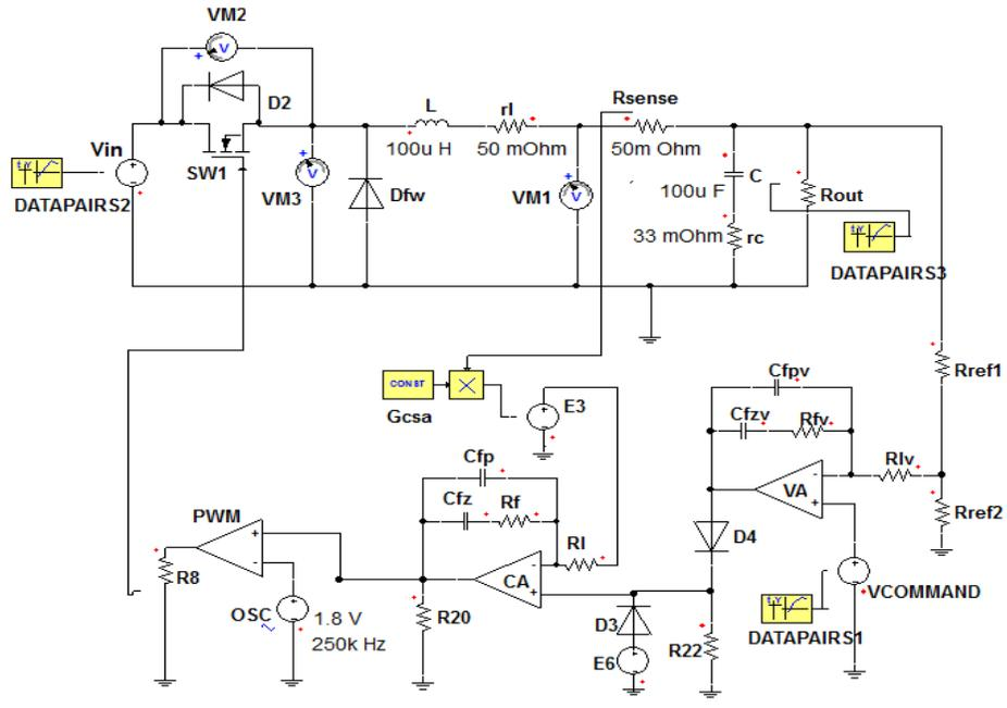
Figure 52 Buck Converter Schematic
