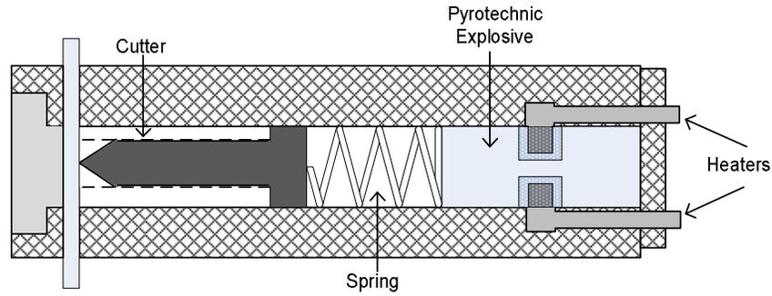
Figure 88 Pyrotechnic Cutter
