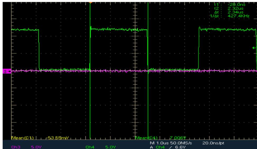
Figure 74 PWM pulses (CH4-Green) for VSENSE=1.945V
