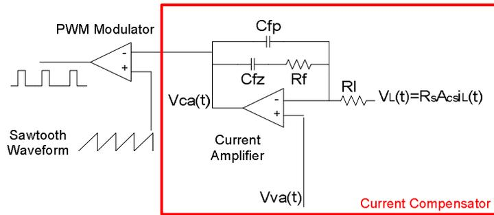
Figure 33 Current Compensator
