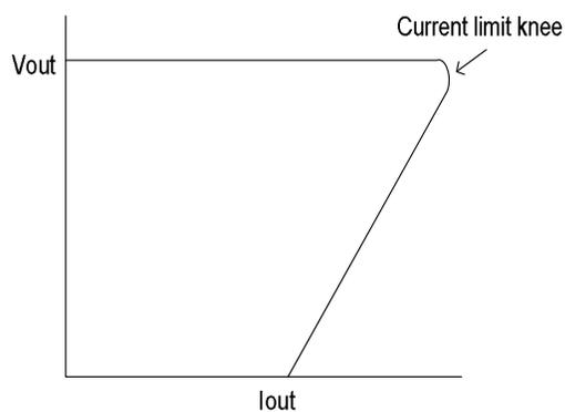
Figure 92 Fold-back Current Limiting
