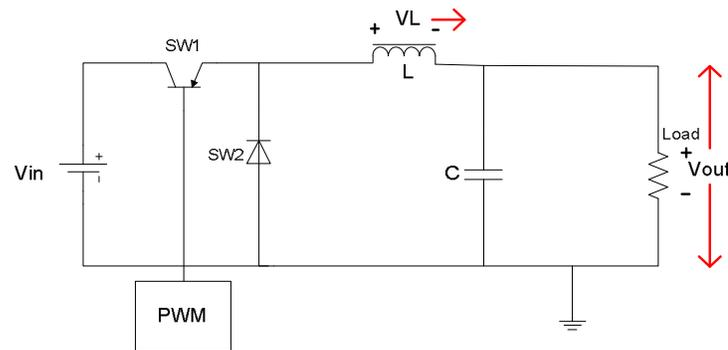
Figure 8 Buck Converter Basic Logic
