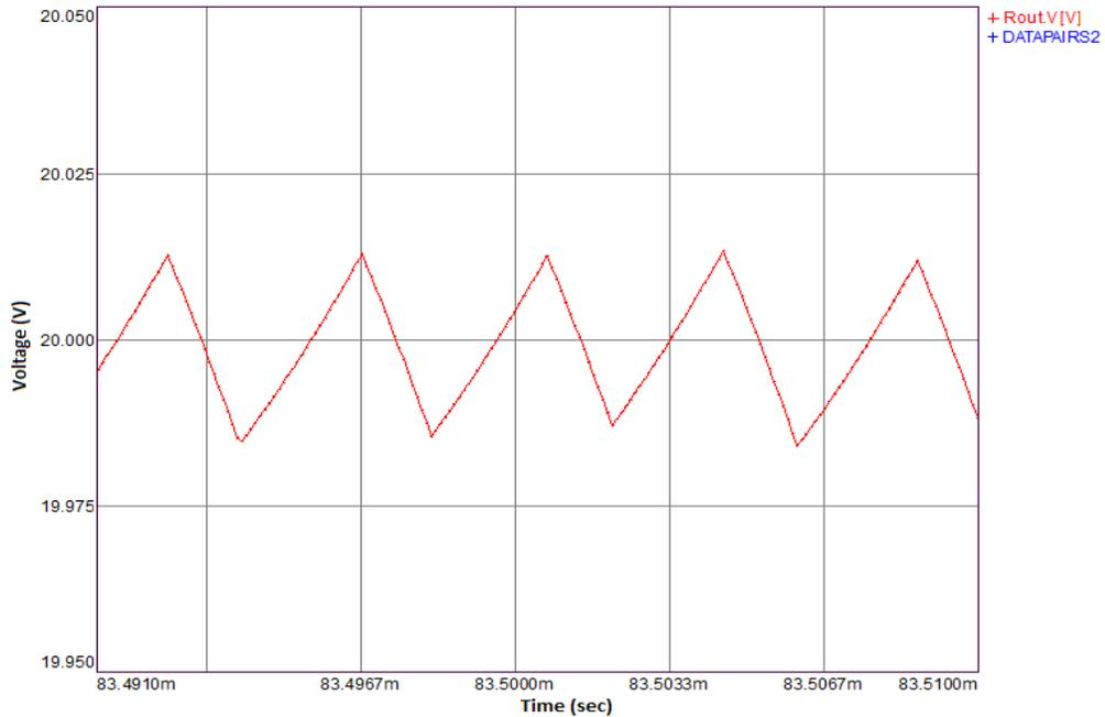
Figure 64 Output Voltage Ripple at  $V_{in}=33V$
