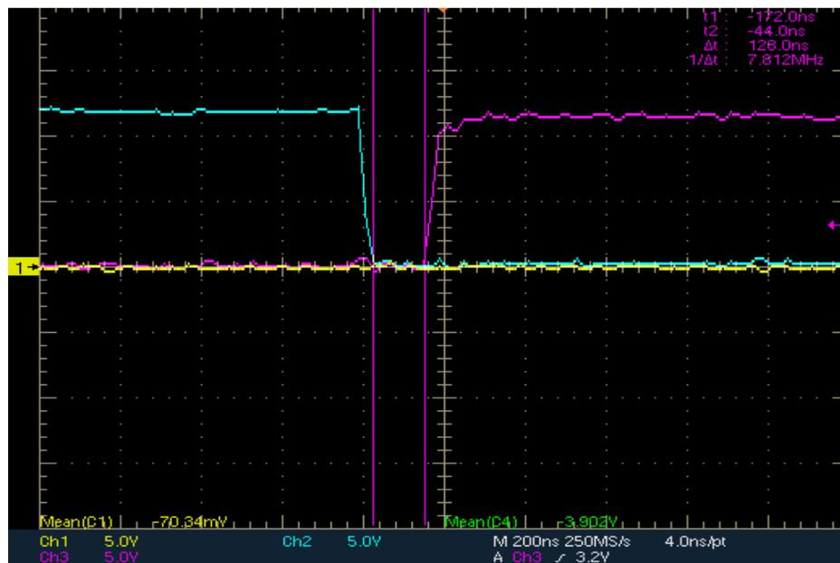
Figure 69 Closer View for LO (CH2-Blue) and HO (CH3-Purple) Outputs with  $R_{gate}=120\Omega$
