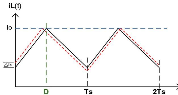
Figure 25 For  $D < 50\%$ , disturbances die out with each cycle
