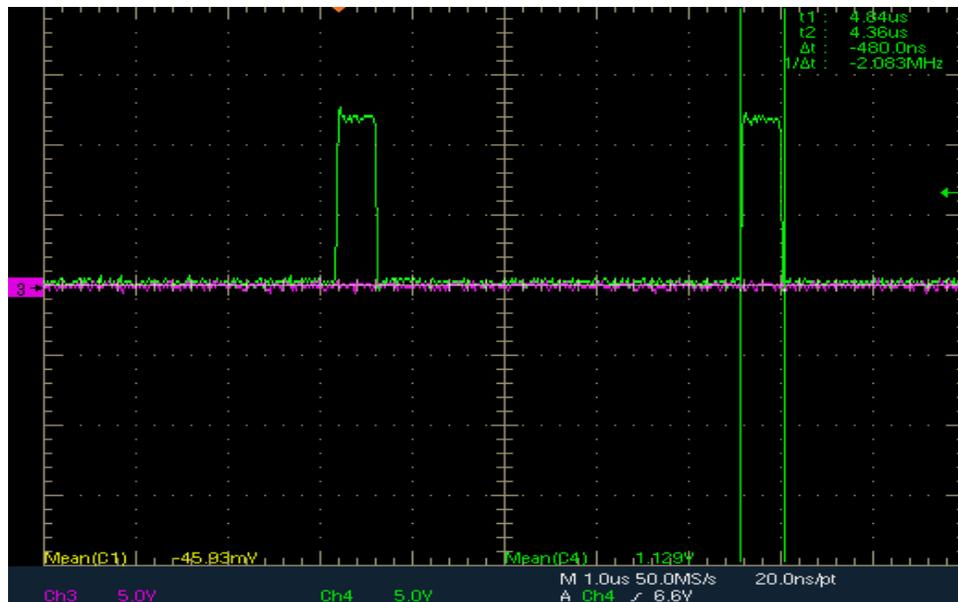
Figure 76 PWM pulses (CH4-Green) for VSENSE=1.972V
