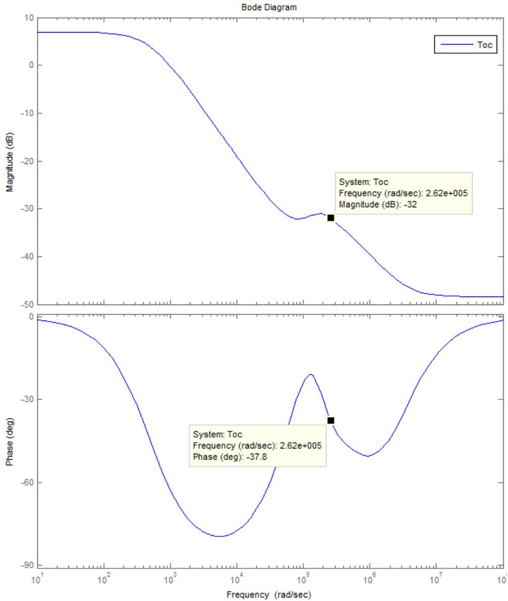
Figure 40 Bode Plot for  $T_{oc}(s)$
