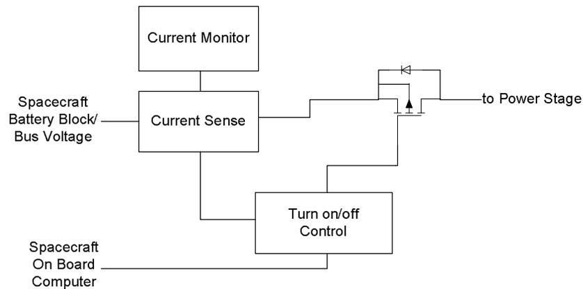
Figure 93 Fold-back Current Limiter with External Turn On/Off Control
