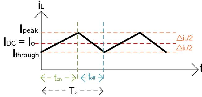
Figure 17 Inductor Current Waveform
