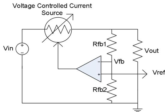
Figure 5 Linear Regulator with Feedback
