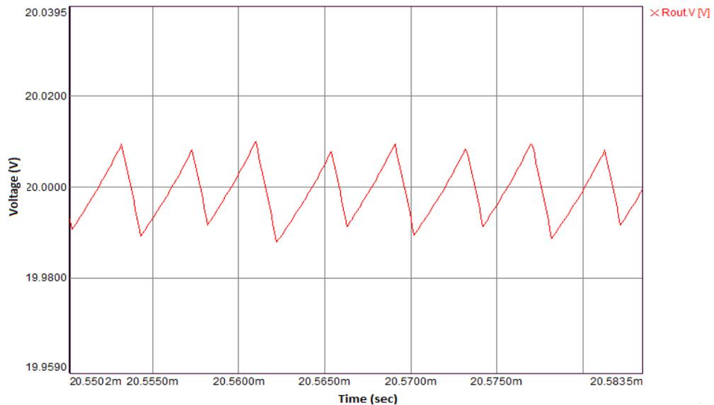
Figure 55 Output Voltage Ripple
