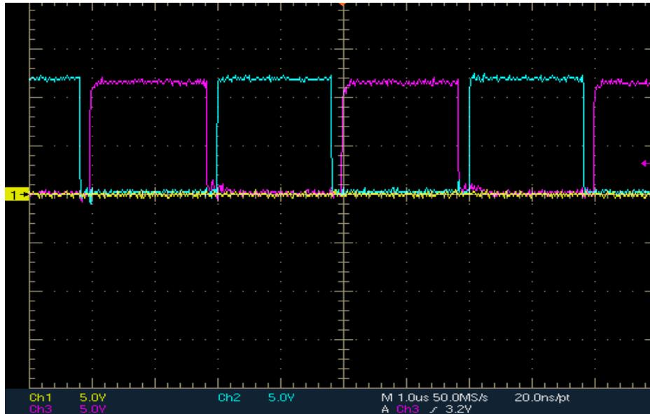
Figure 68 LO (CH2-Blue) and HO (CH3-Purple) Outputs with  $R_{gate}=120\Omega$
