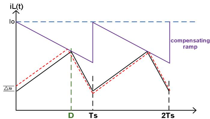
Figure 27 With Slope Compensation Disturbances Die Out with each cycle and for any  $D$
