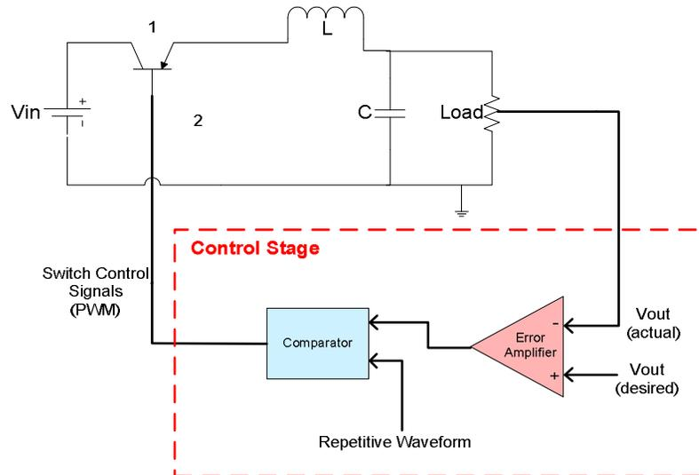
Figure 20 Control Stage of the Buck Converter
