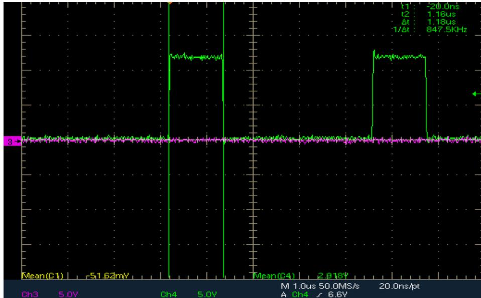
Figure 75 PWM pulses (CH4-Green) for VSENSE=1.963V
