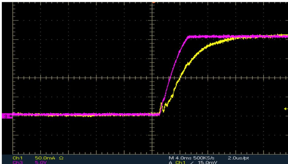
Figure 85 Output Voltage (CH3-Purple) Rise from and Output Current (CH1-Yellow) Rise
