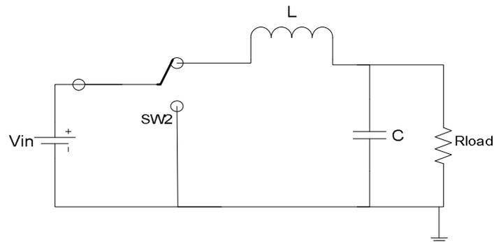
Figure 7 Buck Converter Power Stage
