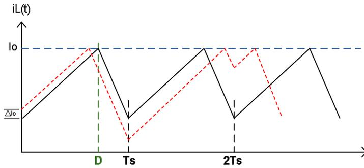
Figure 26 For  $D > 50\%$ , disturbances grow with each cycle and sub-harmonic oscillations are observed
