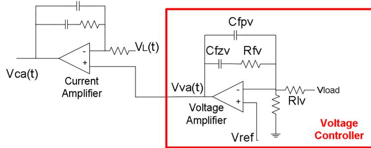
Figure 35 Voltage Controller
