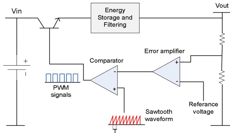
Figure 6 Switch Mode Regulator
