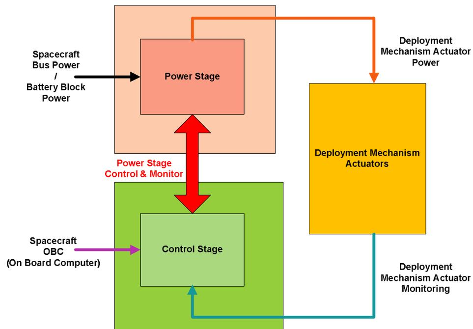
Figure 1 Deployment Mechanism Driver Main Blocks
