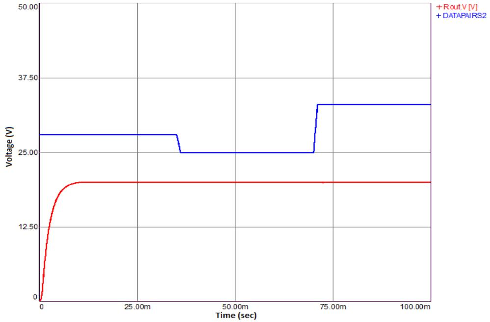
Figure 60 Input Voltage Change (Blue Line) and Output Voltage Response (Red Line)
