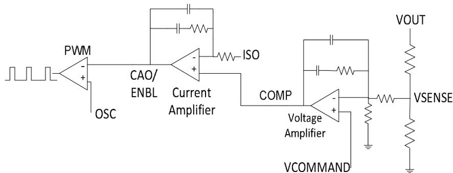
Figure 49 Current Compensator, Voltage Controller and PWM configuration
