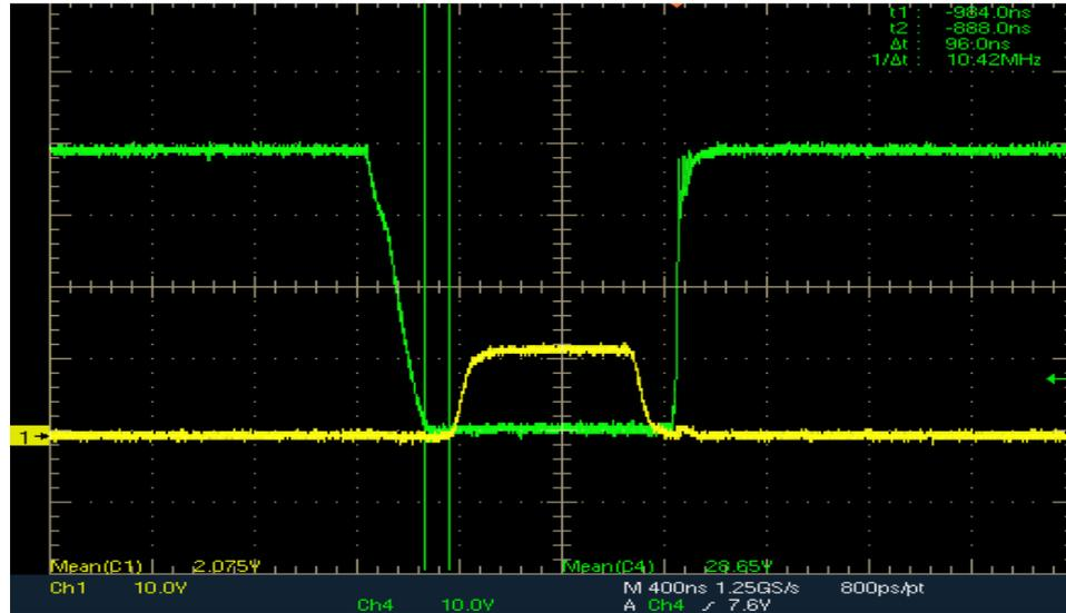
Figure 82 Delay between High Side (CH4-Green) and Low Side (CH1-Yellow) Switch Drive Pulses
