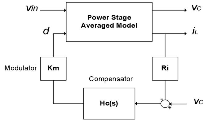
Figure 31 Block Diagram of State Space Averaged Converter Model [62]
