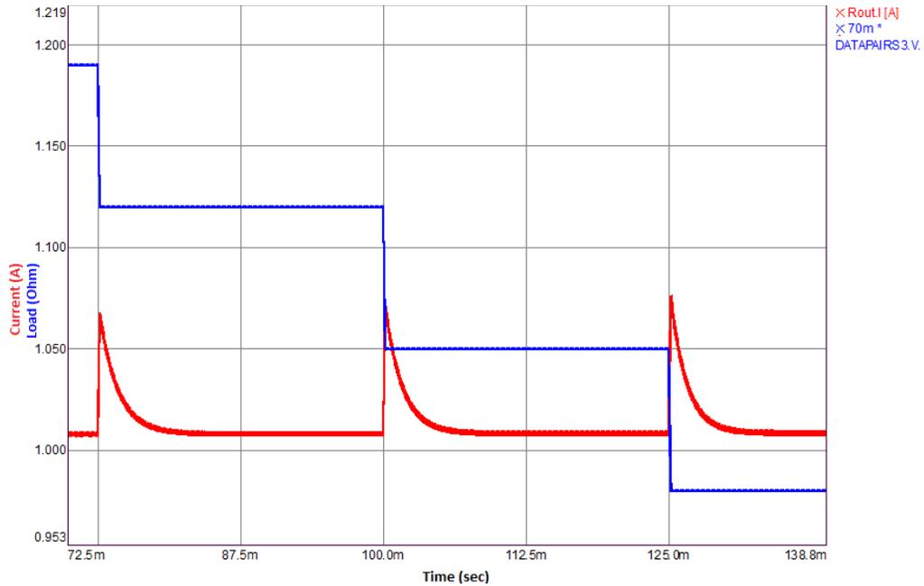
Figure 59 Zoomed View for Output Current (Red Line) during Output Load Change (Blue Line)
