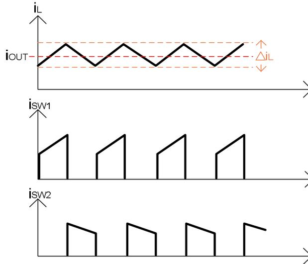
Figure 14 Waveforms in Continuous Conduction Mode
