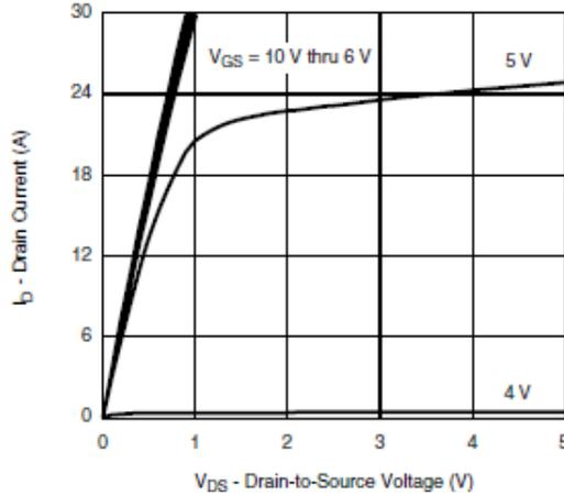
Figure 37 Output Characteristics [69]
