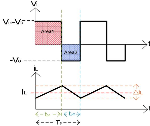
Figure 16 Inductor Voltage  $V_L$  and Inductor Current  $I_L$  during CCM Operation
