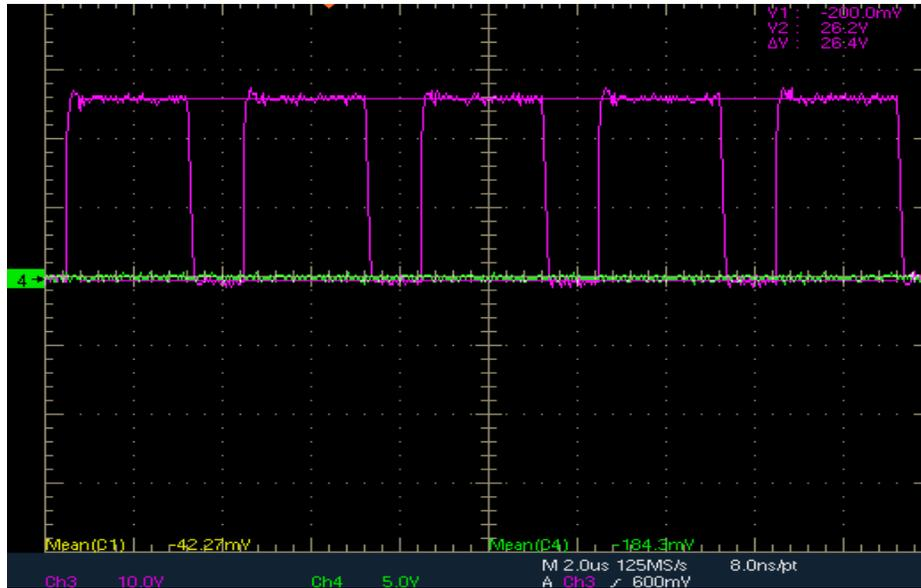
Figure 70 Freewheeling Diode Waveform
