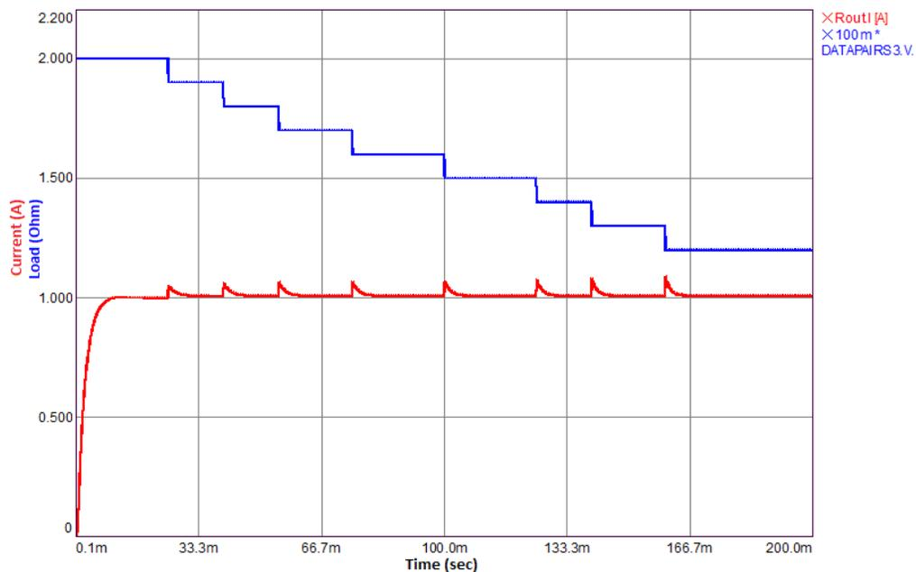
Figure 58 Output Current (Red Line) during Output Load Change (Blue Line)
