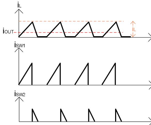
Figure 15 Waveforms in discontinuous conduction mode
