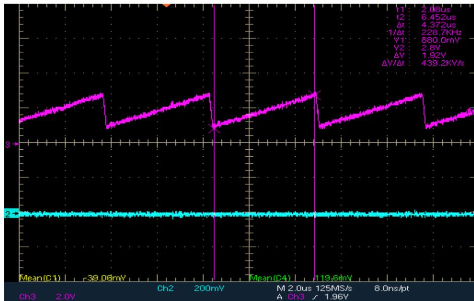
Figure 72 Sawtooth Voltage Waveform (CH3-Purple)
