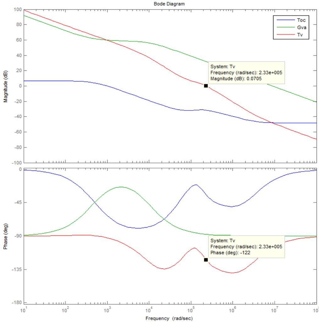
Figure 41 Bode Plot for  $T_{oc}(s)$ ,  $T_v(s)$  and  $G_{va}(s)$
