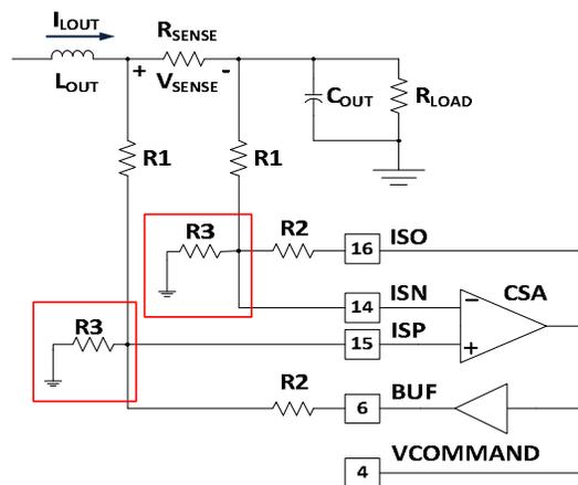
Figure 48 Current Sense Amplifier with Voltage Divider Network
