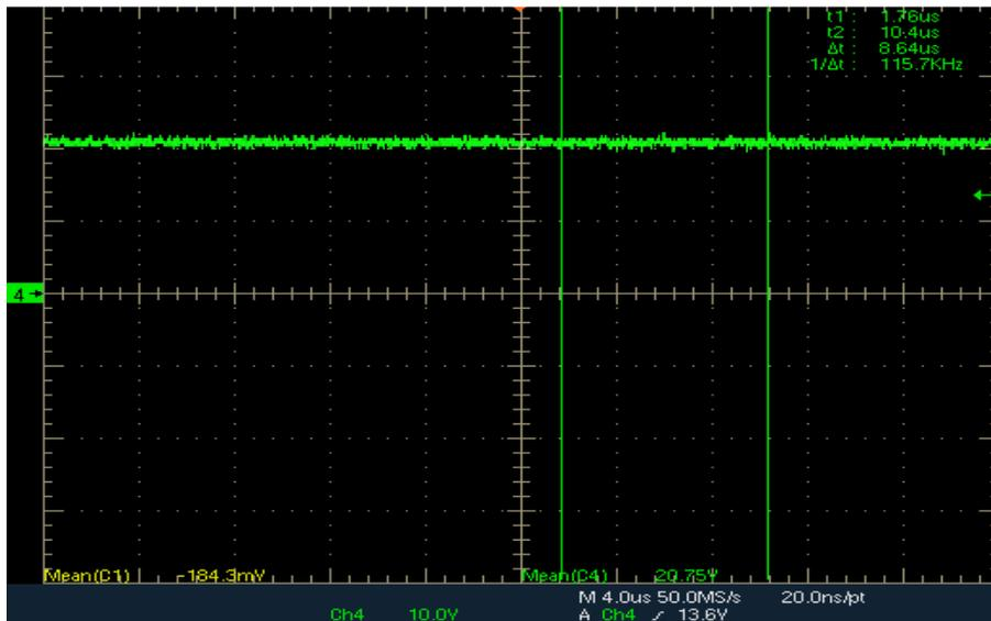
Figure 77 Output Voltage for  $V_{in}=28V$  and  $R_{out}=200\Omega$
