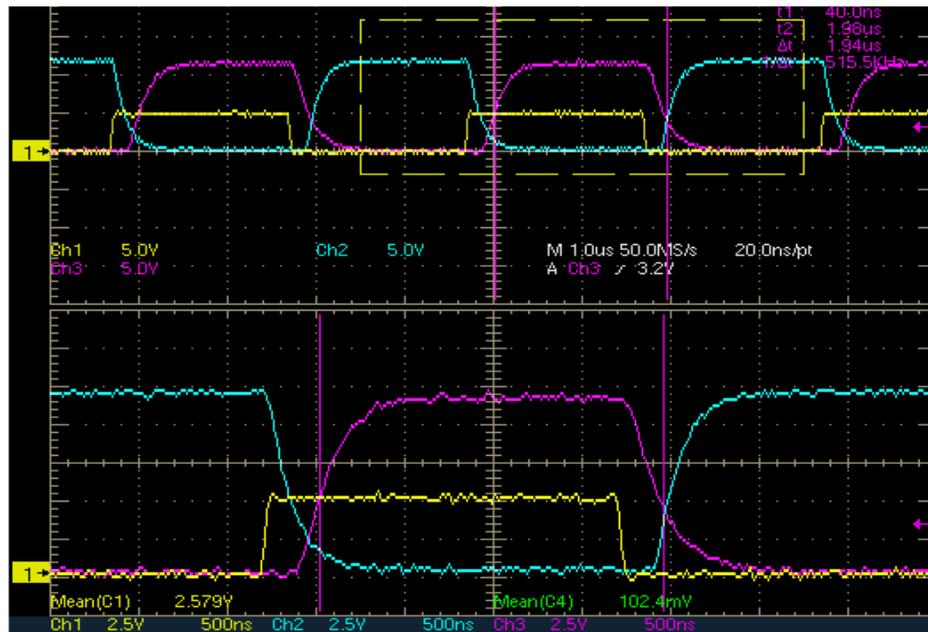
Figure 67 PWM Pulses (CH1-Yellow), LO (CH2-Blue) and HO (CH3-Purple) Outputs
