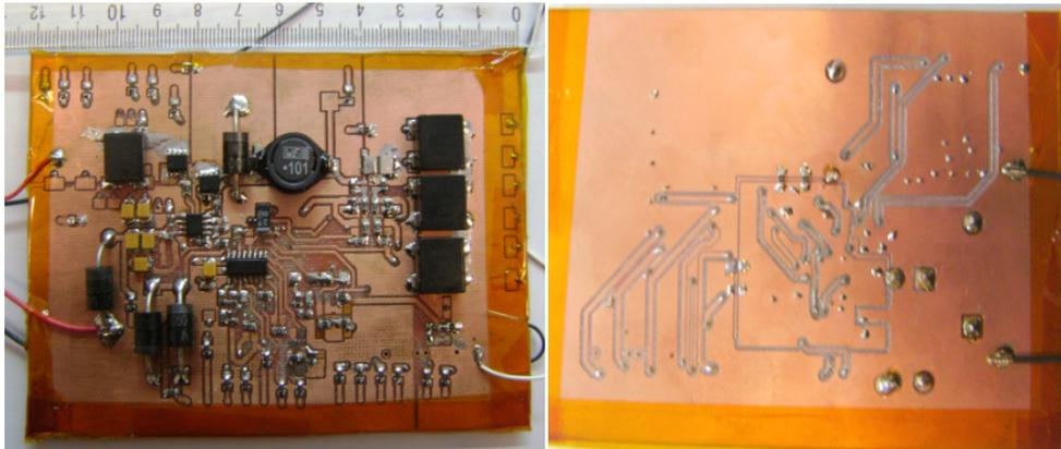
Figure 66 Power Stage Circuitry Top and Bottom Views Respectively
