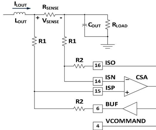
Figure 47 Current Sense Amplifier Configuration [24]
