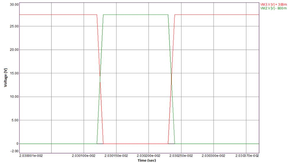
Figure 57 Voltage Waveforms for SW1 and  $Df_w$  via VM2.V (Green Line) and VM3.V (Red Line) respectively
