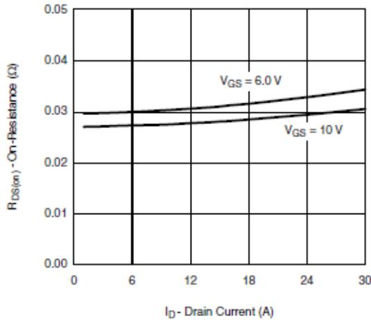
Figure 38 On-Resistance vs. Drain Current [69]
