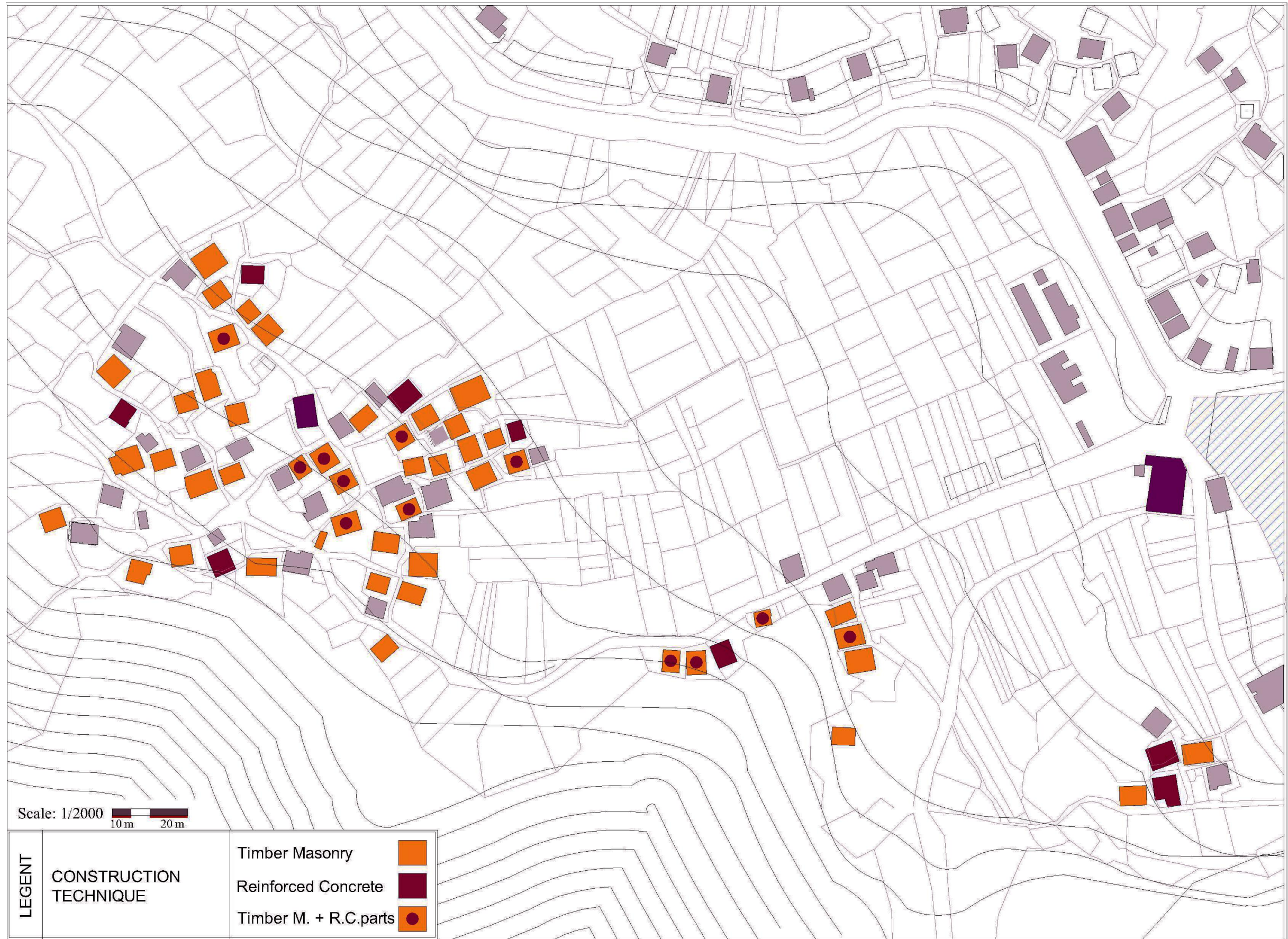
Figure 139, Construction Technique of the Buildings in the Study Area
