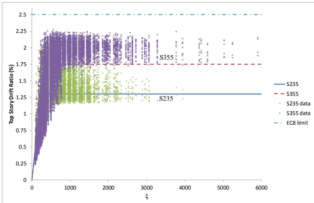
Figure 4.4: Inelastic Top Story Drift Ratios for IC III with Overstrength Rule
