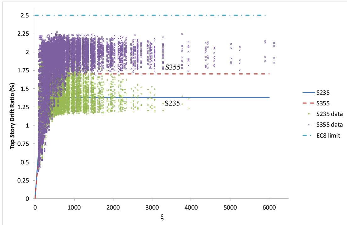
Figure 4.7: Inelastic Top Story Drift Ratios for IC III without Overstrength Rule
