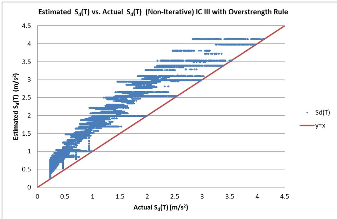
Figure 3.15: Estimated  $S_d(T)$  vs. Actual  $S_d(T)$  – IC III – Non-Iterative with Overstrength Rule
