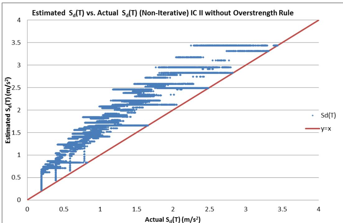
Figure 3.23: Estimated  $S_d(T)$  vs. Actual  $S_d(T)$  – IC II – Non-Iterative without Overstrength Rule
