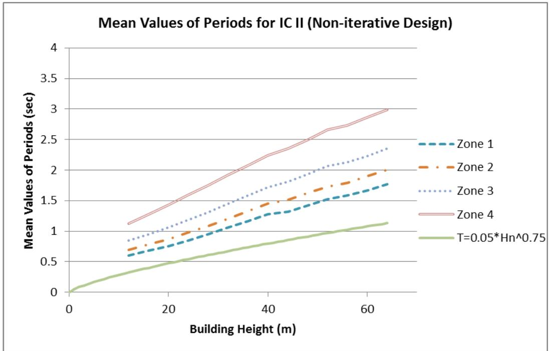
Figure 3.33: Mean Values of Periods for IC II (Non-Iterative Design)
