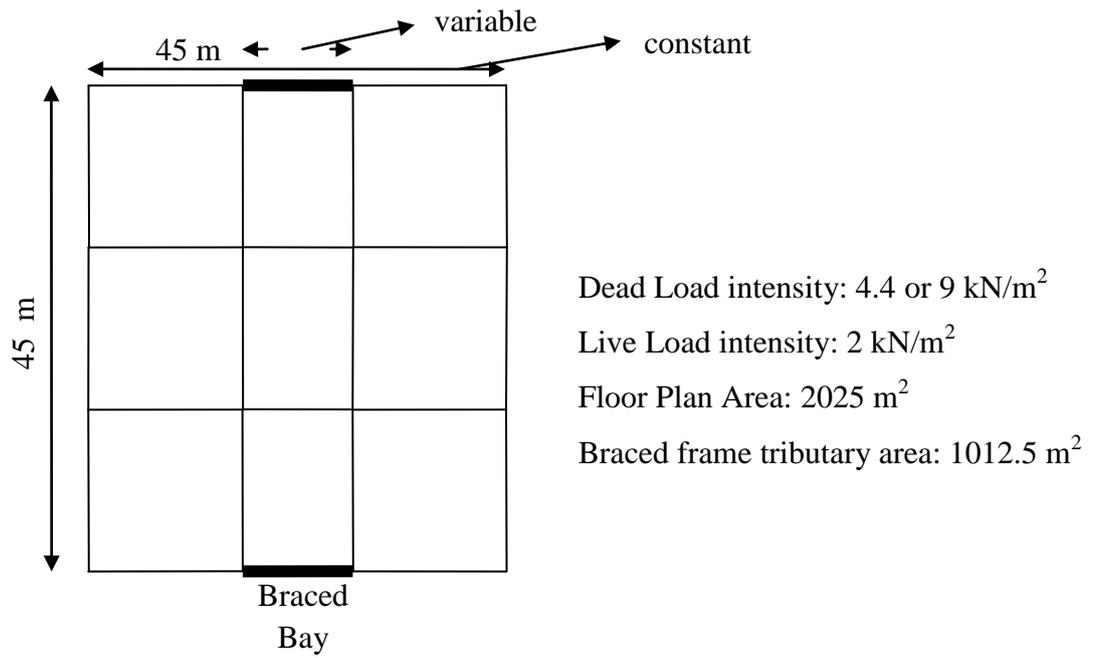
Figure 3.6: Plan View of the Building with Two Braced Bays with BFTA of 1012.5 m<sup>2</sup>
