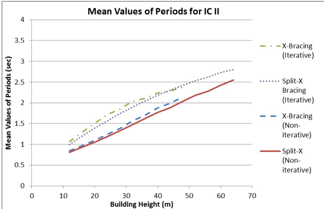
Figure 3.35: Mean Values of Periods according to Bracing Types for IC II
