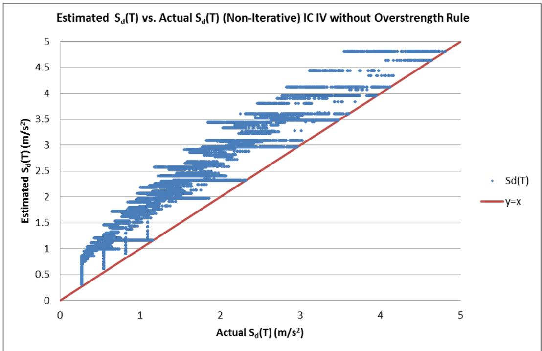
Figure 3.31: Estimated  $S_d(T)$  vs. Actual  $S_d(T)$  – IC IV – Non-Iterative without Overstrength Rule
