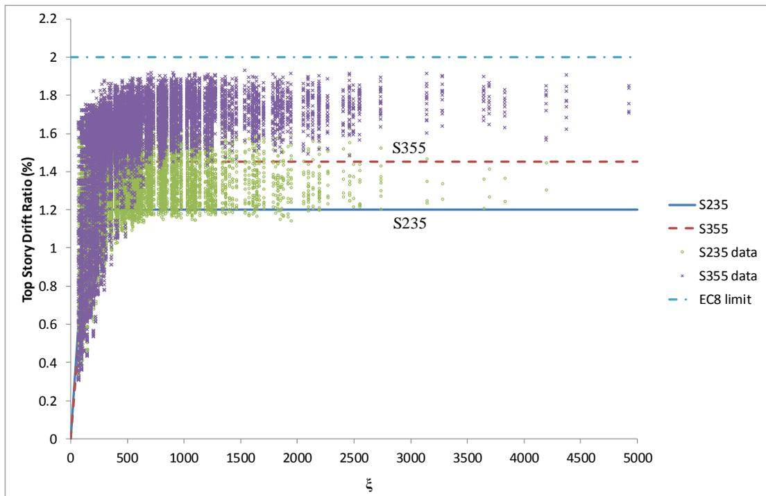
Figure 4.6: Inelastic Top Story Drift Ratios for IC II without Overstrength Rule
