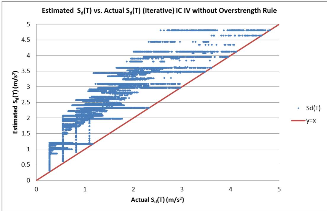
Figure 3.32: Estimated  $S_d(T)$  vs. Actual  $S_d(T)$  – IC IV – Iterative without Overstrength Rule
