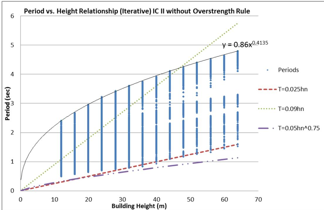
Figure 3.22: Period vs. Height Relationship – IC II – Iterative without Overstrength Rule
