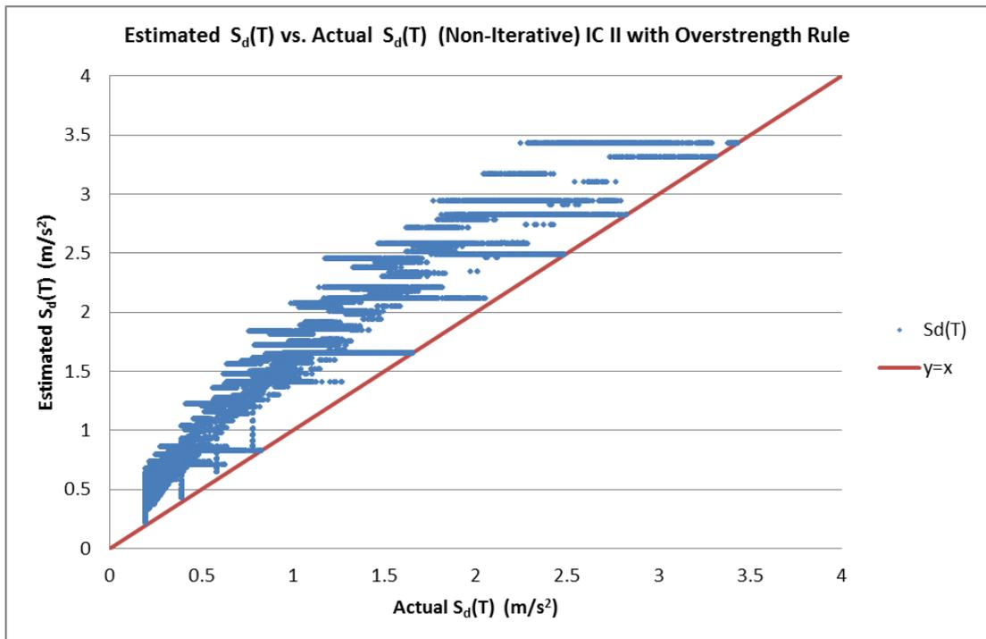
Figure 3.11: Estimated  $S_d(T)$  vs. Actual  $S_d(T)$  – IC II – Non-Iterative with Overstrength Rule
