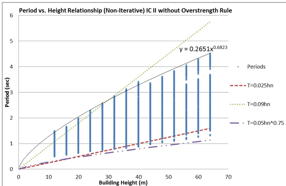
Figure 3.21: Period vs. Height Relationship – IC II – Non-Iterative without Overstrength Rule
