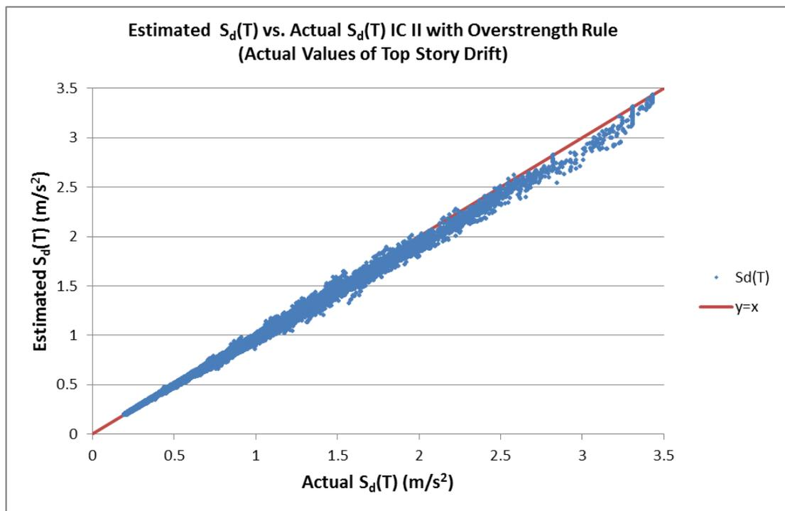
Figure 4.9: Estimated vs. Actual  $S_d(T)$  IC II with Overstrength Rule (Actual Values of Top Story Drift)
