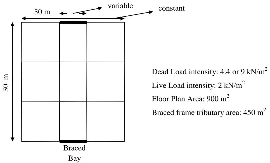
Figure 3.4: Plan View of the Building with Two Braced Bays with BFTA of 450 m<sup>2</sup>
