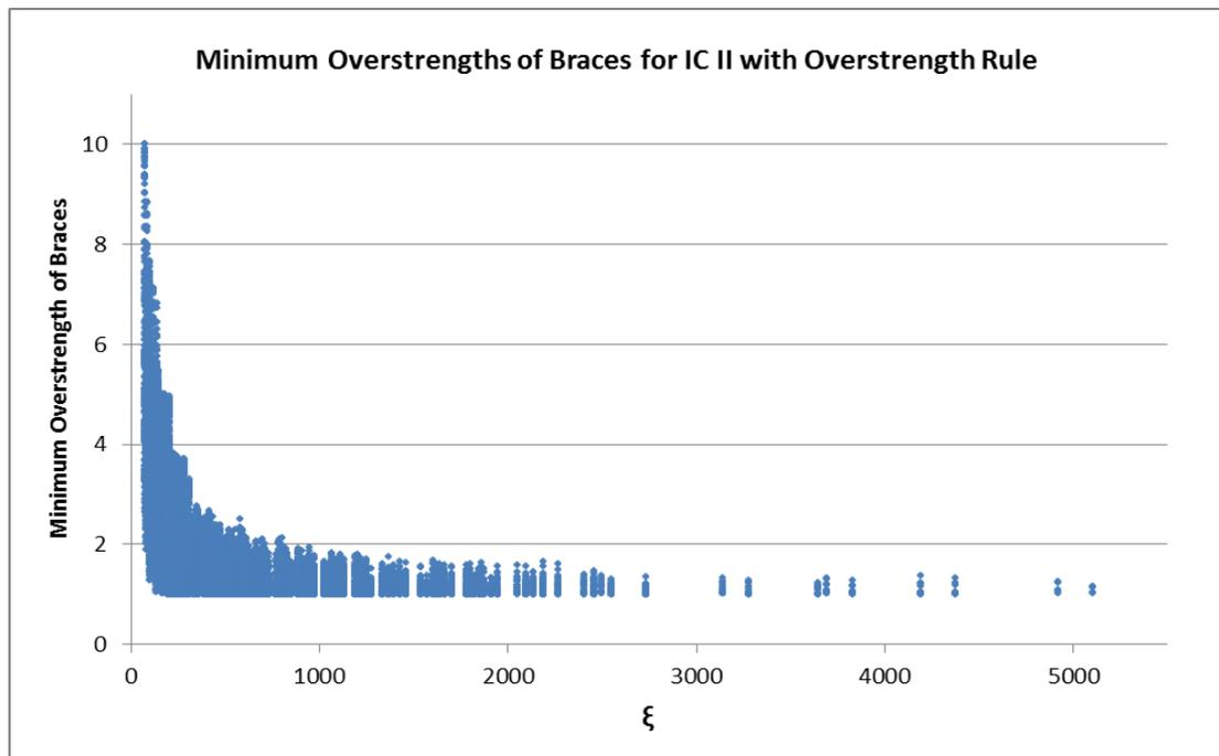
Figure 3.36: Minimum Overstrengths of Braces for IC II with Overstrength Rule
