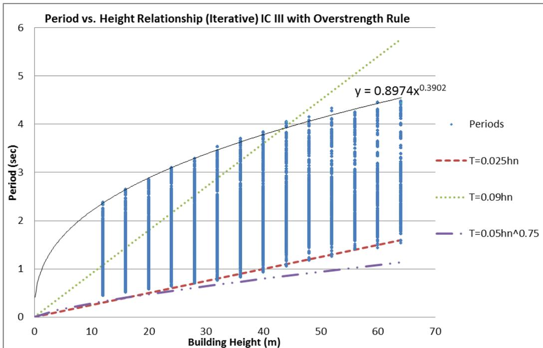
Figure 3.14: Period vs. Height Relationship – IC III – Iterative with Overstrength Rule
