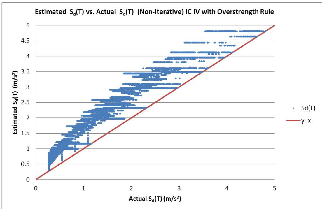
Figure 3.19: Estimated  $S_d(T)$  vs. Actual  $S_d(T)$  – IC IV – Non-Iterative with Overstrength Rule
