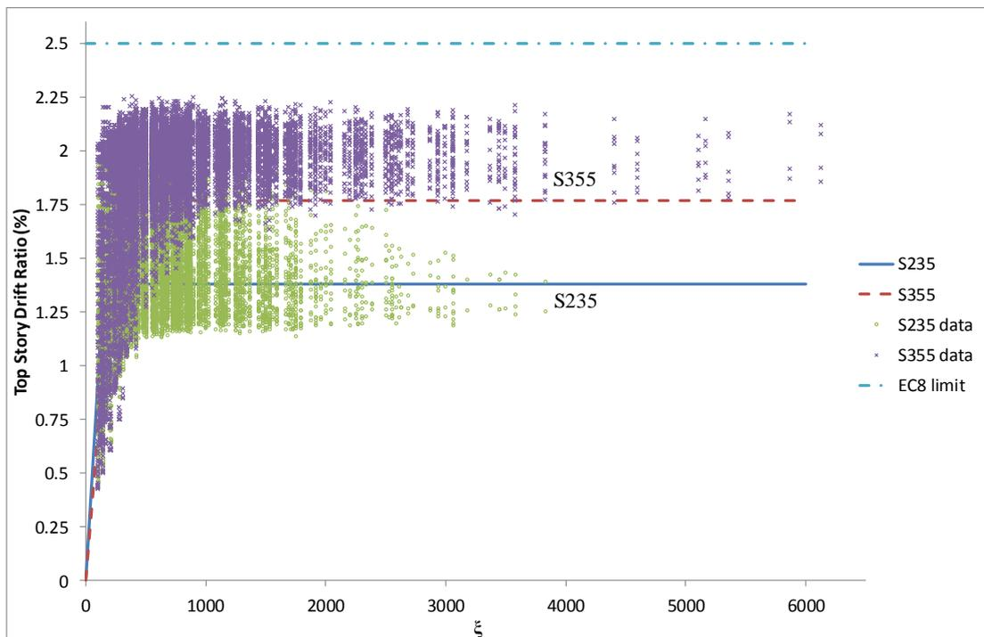
Figure 4.8: Inelastic Top Story Drift Ratios for IC IV without Overstrength Rule
