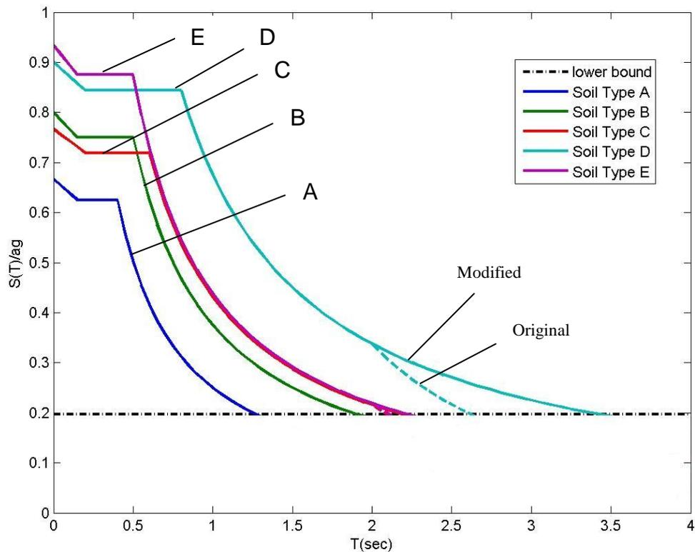
Figure 4.2: A Comparison of the Original and Modified Spectra for  $q=4$
