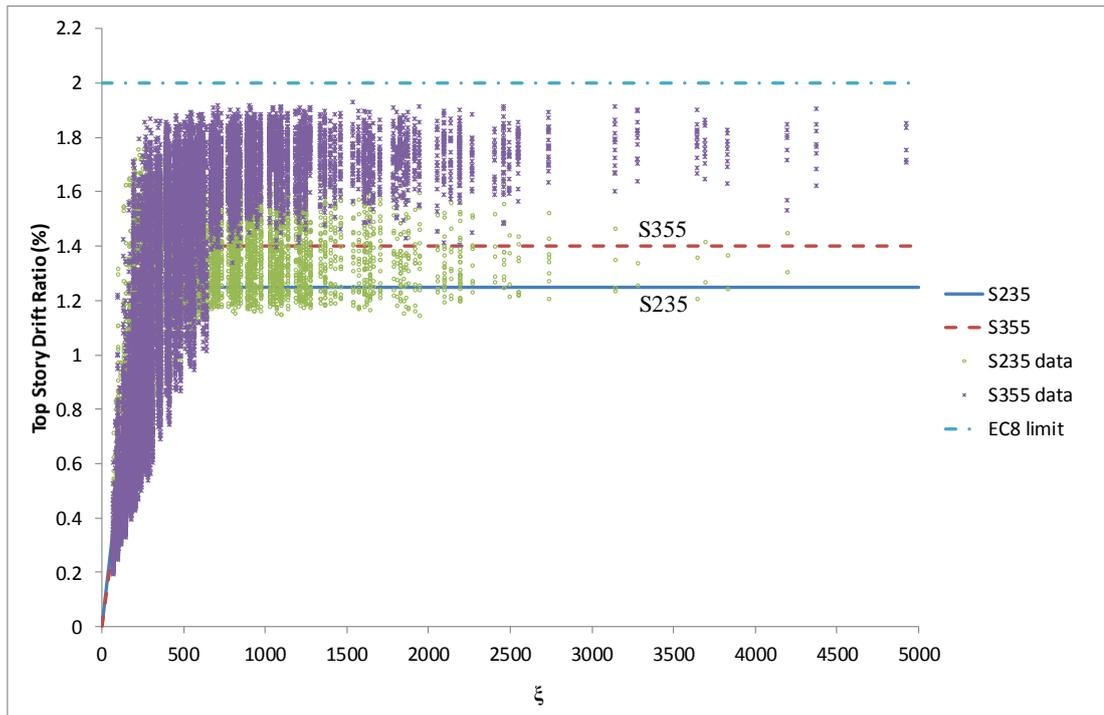
Figure 4.3: Inelastic Top Story Drift Ratios for IC II with Overstrength Rule
