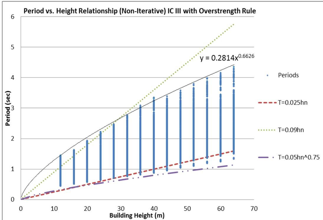
Figure 3.13: Period vs. Height Relationship – IC III – Non-Iterative with Overstrength Rule
