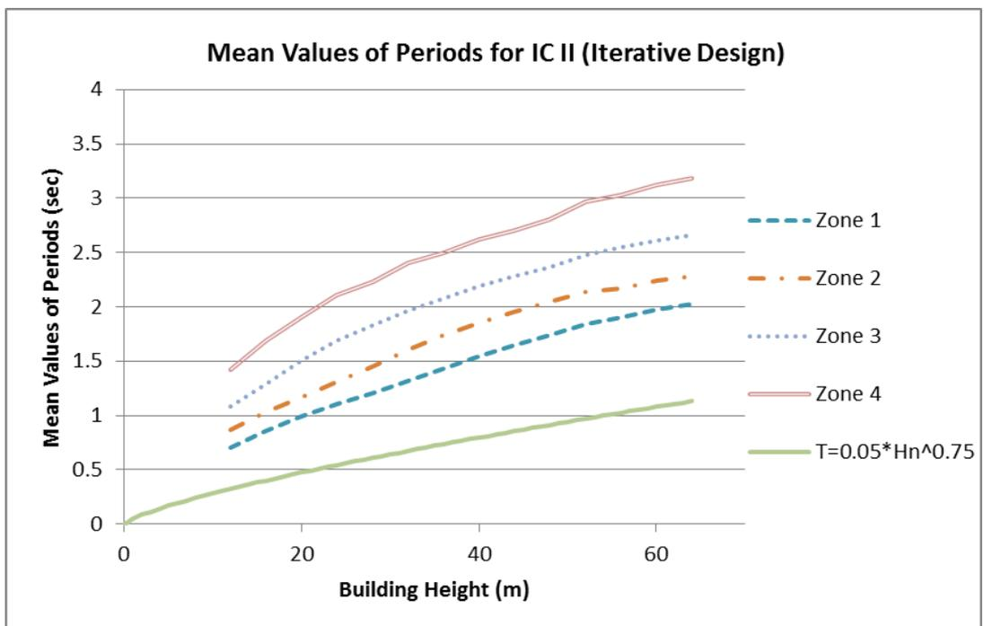
Figure 3.34: Mean Values of Periods for IC II (Iterative Design)
