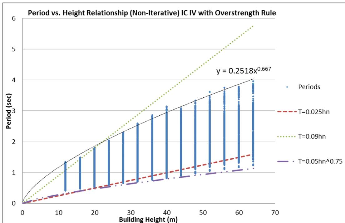
Figure 3.17: Period vs. Height Relationship – IC IV – Non-Iterative with Overstrength Rule
