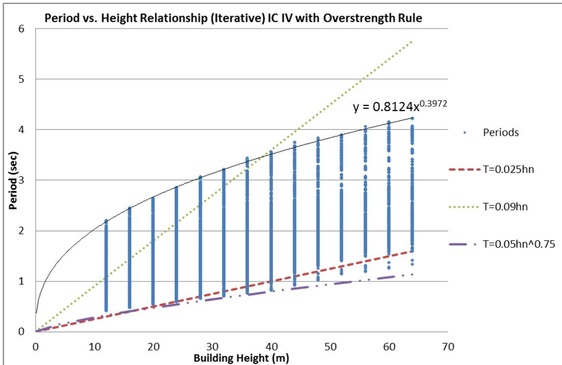
Figure 3.18: Period vs. Height Relationship – IC IV – Non-Iterative with Overstrength Rule
