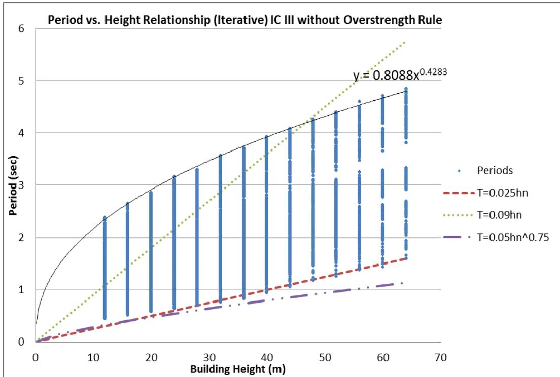
Figure 3.26: Period vs. Height Relationship – IC III – Iterative without Overstrength Rule
