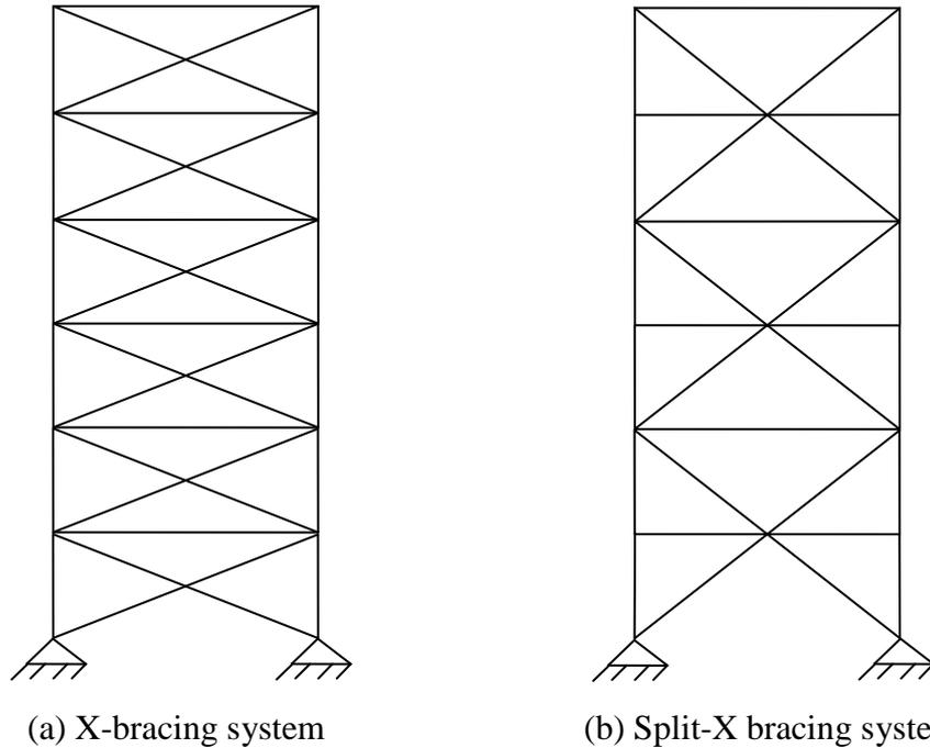
Figure 3.1: Bracing Systems (a) X-bracing system, (b) Split-X bracing system
