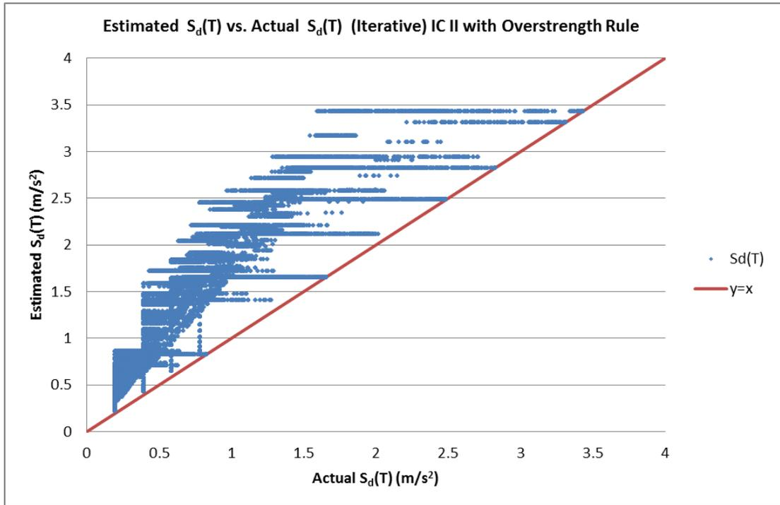
Figure 3.12: Estimated  $S_d(T)$  vs. Actual  $S_d(T)$  – IC II – Iterative with Overstrength Rule
