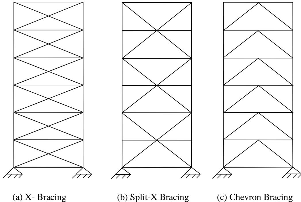
Figure 1.1: Typical Concentrically Braced Frames
