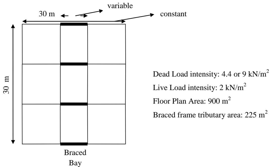
Figure 3.5: Plan View of the Building with Four Braced Bays with BFTA of 225 m<sup>2</sup>
