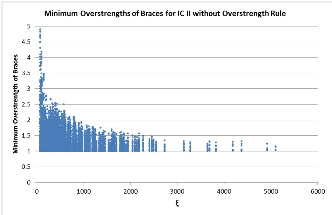
Figure 3.37: Minimum Overstrengths of Braces for IC II without Overstrength Rule
