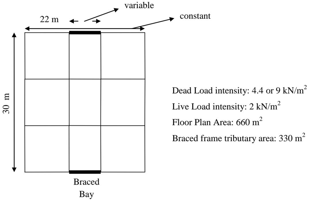
Figure 3.2: Plan View of the Building with Two Braced Bays with BFTA of 330 m<sup>2</sup>
