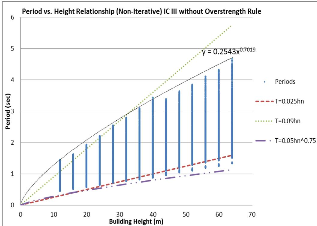
Figure 3.25: Period vs. Height Relationship – IC III – Non-Iterative without Overstrength Rule
