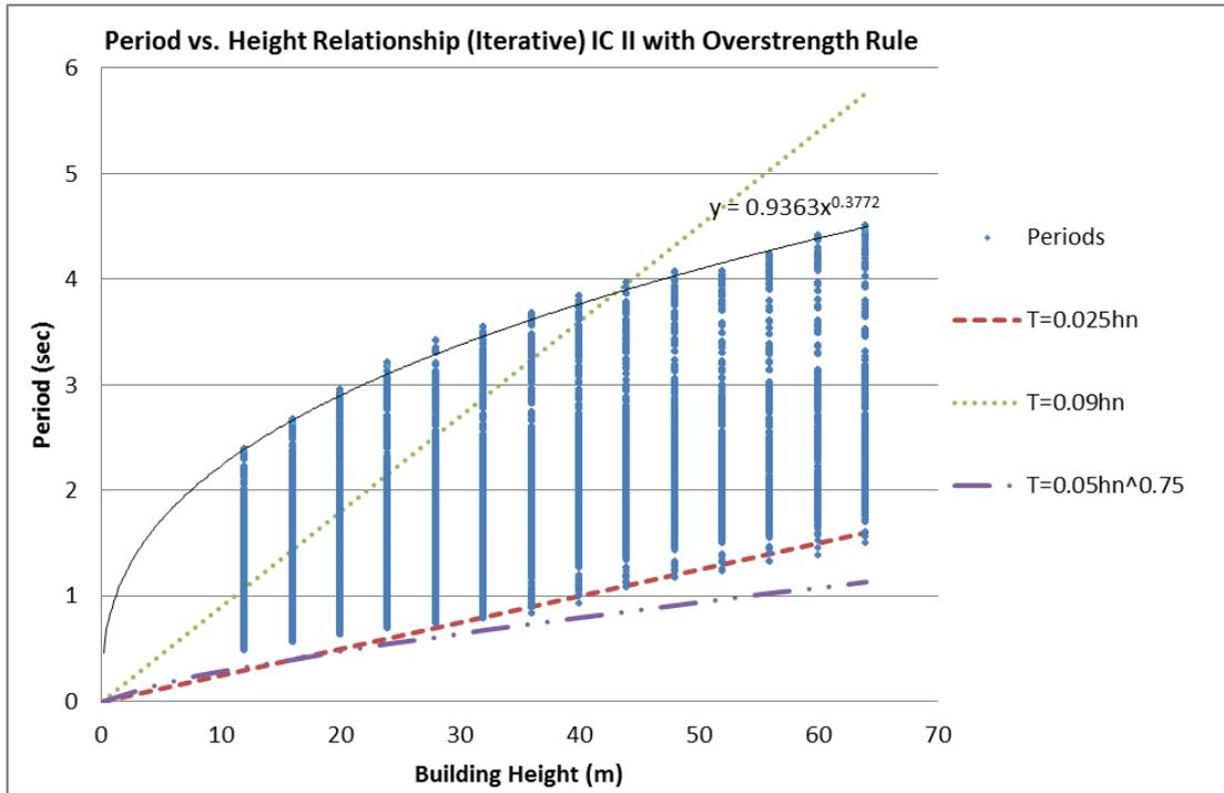
Figure 3.10: Period vs. Height Relationship – IC II – Iterative with Overstrength Rule
