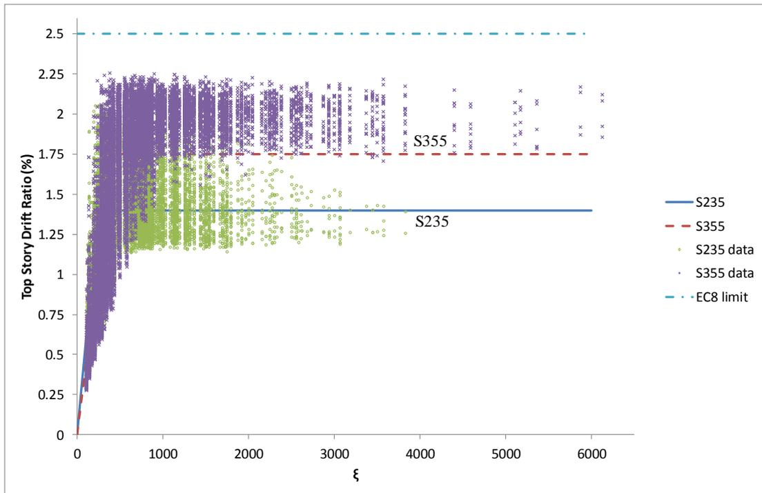
Figure 4.5: Inelastic Top Story Drift Ratios for IC IV with Overstrength Rule
