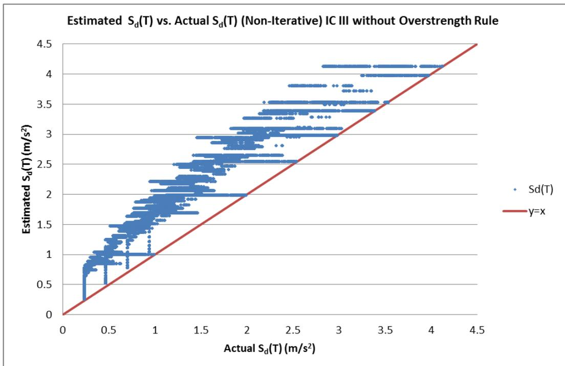
Figure 3.27: Estimated  $S_d(T)$  vs. Actual  $S_d(T)$  – IC III – Non-Iterative without Overstrength Rule
