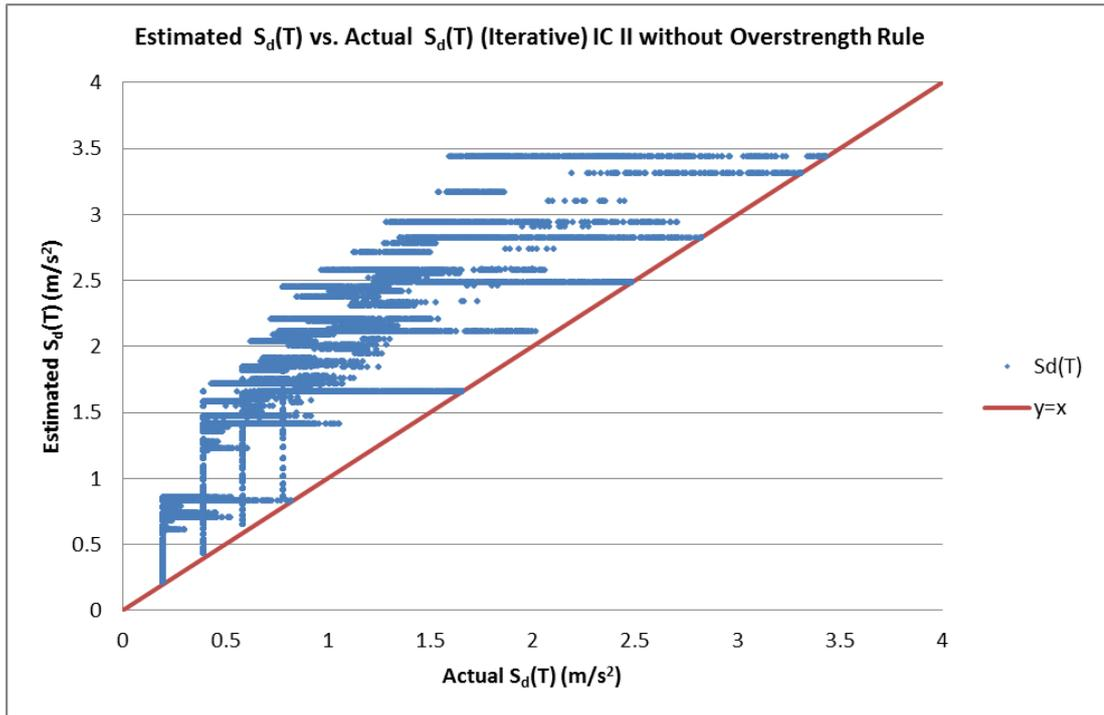
Figure 3.24: Estimated  $S_d(T)$  vs. Actual  $S_d(T)$  – IC II – Iterative without Overstrength Rule
