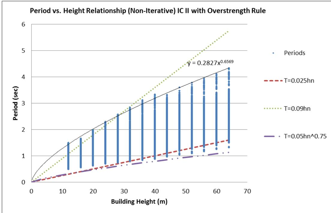
Figure 3.9: Period vs. Height Relationship – IC II – Non-Iterative with Overstrength Rule
