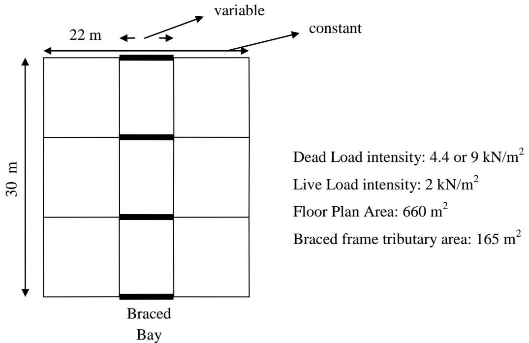
Figure 3.3: Plan View of the Building with Four Braced Bays with BFTA of 165 m<sup>2</sup>
